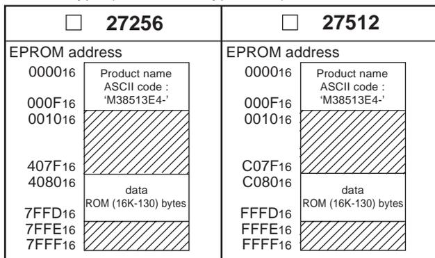
In the address space of the microcomputer, the internal ROM area is from address C080<sub>16</sub> to FFFD<sub>16</sub>. The reset vector is stored in addresses FFFC<sub>16</sub> and FFFD<sub>16</sub>.
