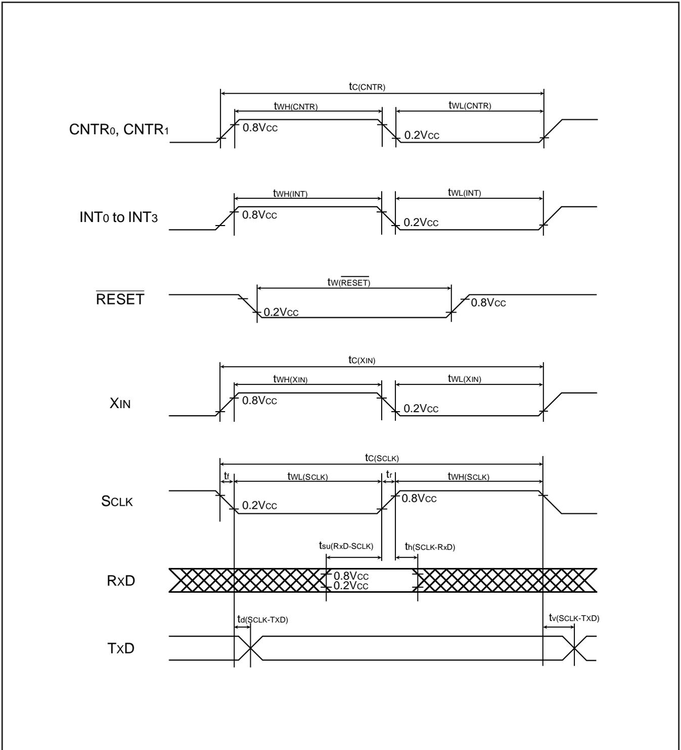
Fig. 52 Timing diagram
