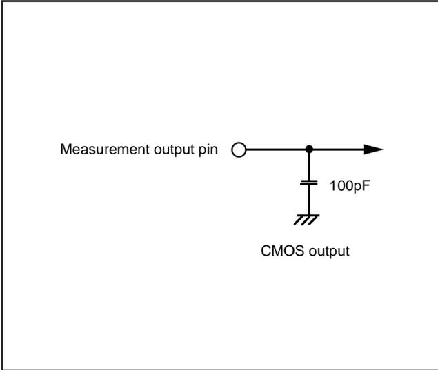
Fig. 50 Circuit for measuring output switching characteristics (1)
