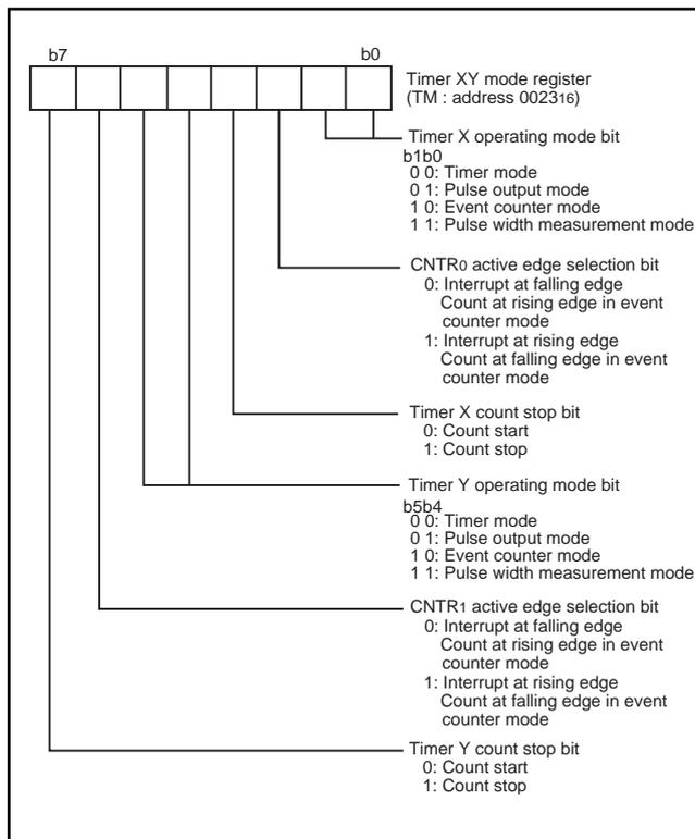
Fig. 11 Structure of timer XY mode register
