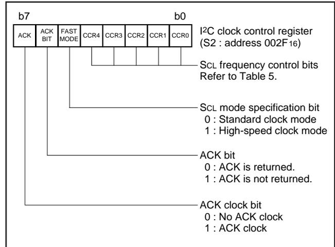
**Fig. 21 Structure of I<sup>2</sup>C clock control register**
