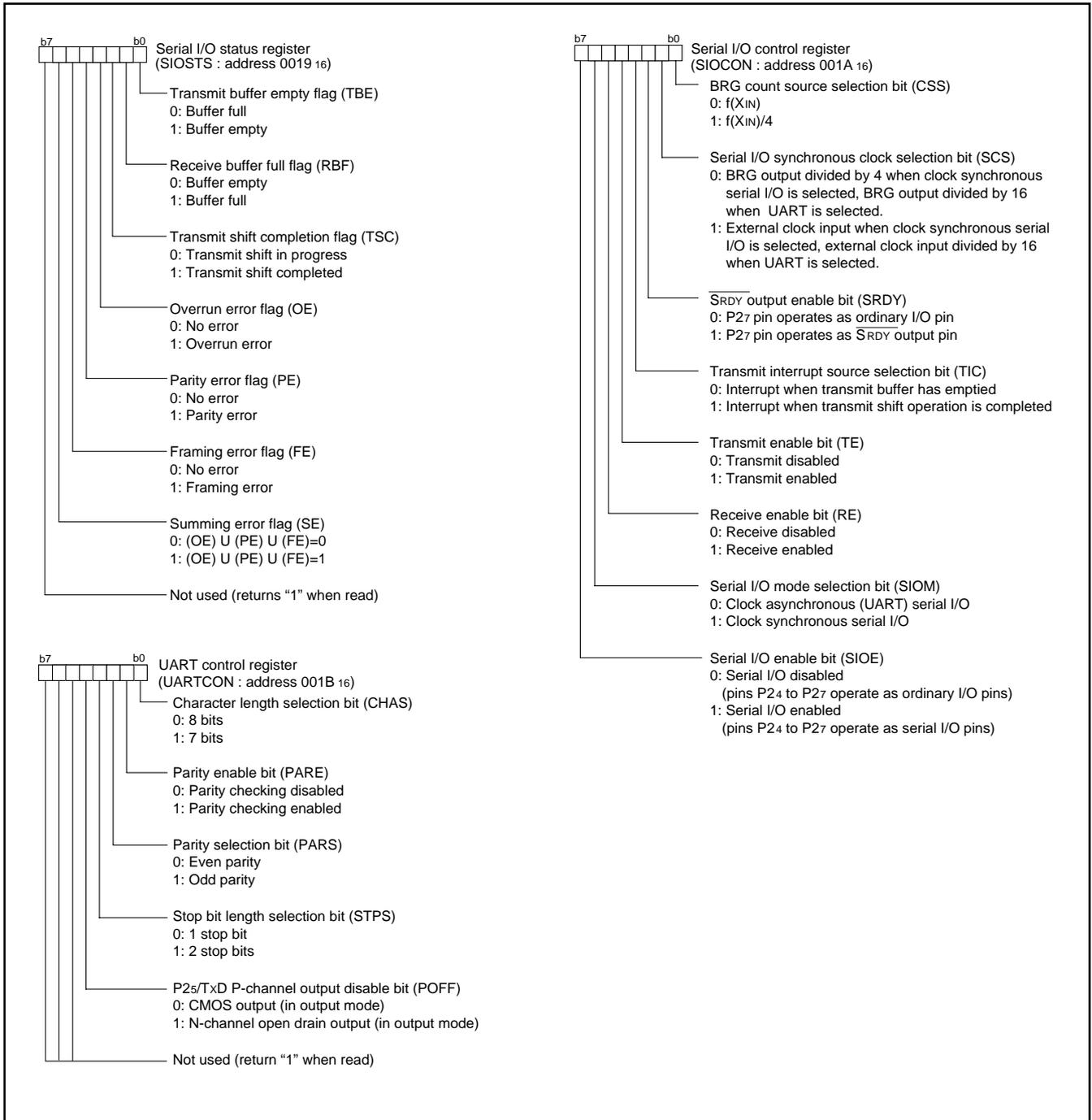
Fig. 18 Structure of serial I/O control registers
