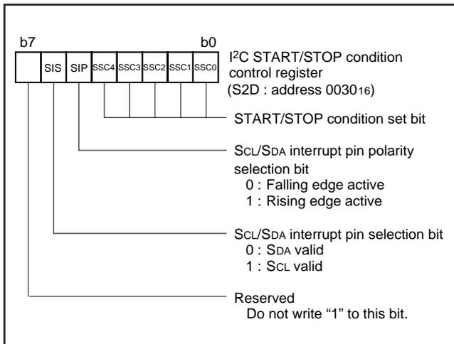
Fig. 30 Structure of I<sup>2</sup>C START/STOP condition control register
