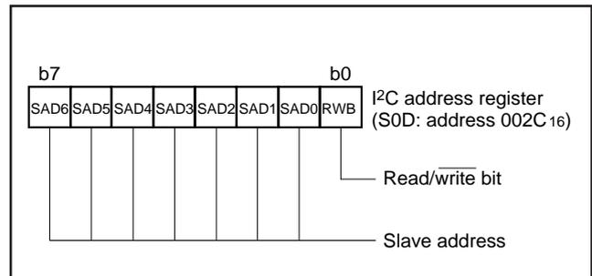
Fig. 20 Structure of I<sup>2</sup>C address register
