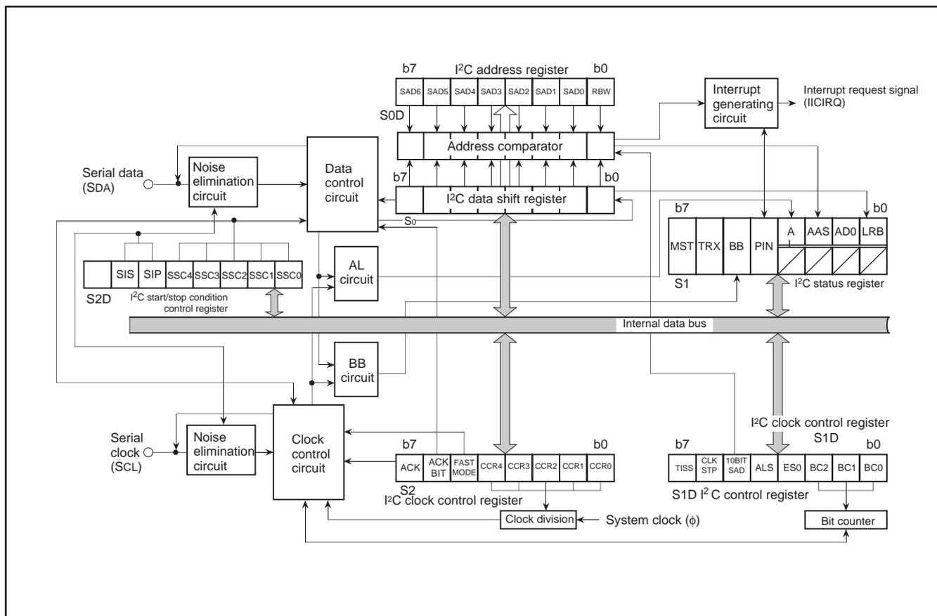
**Fig. 19 Block diagram of multi-master I<sup>2</sup>C-BUS interface**
