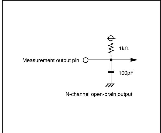
Fig. 51 Circuit for measuring output switching characteristics (2)
