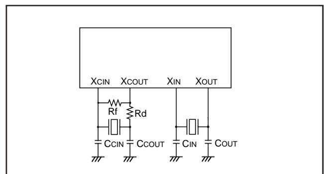
Fig. 44 Ceramic resonator circuit
