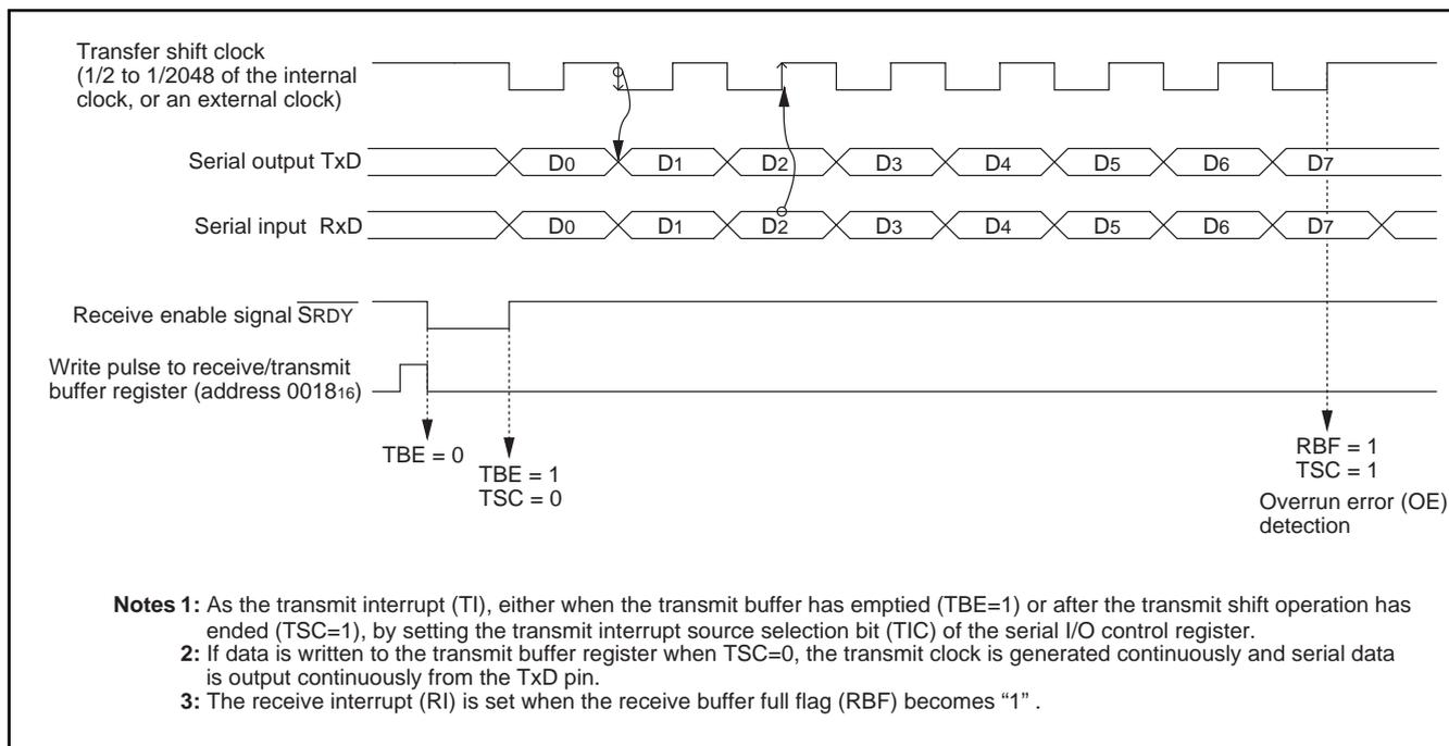
Fig. 15 Operation of clock synchronous serial I/O function
