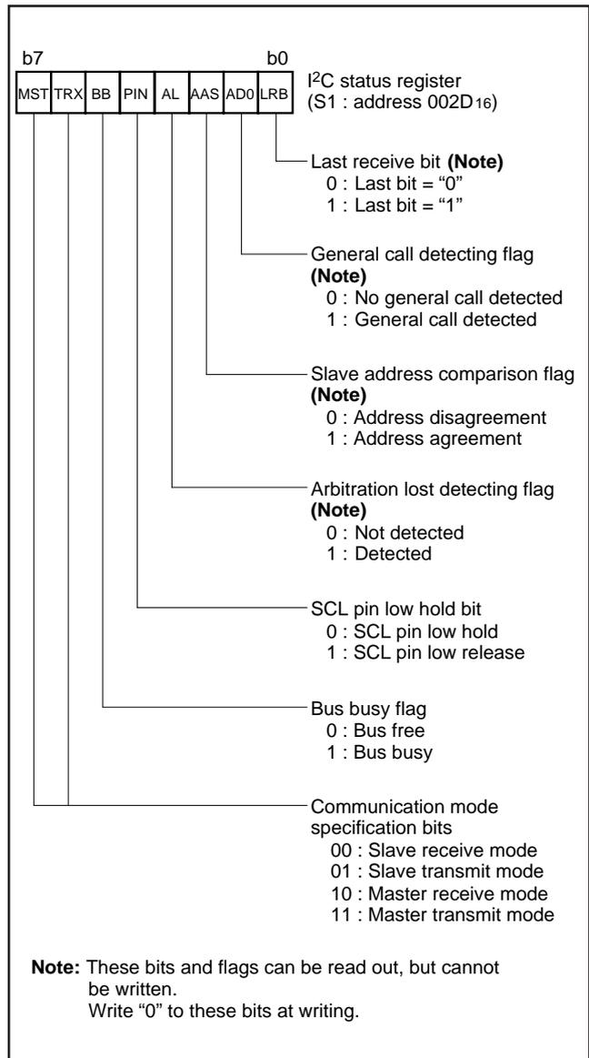
Fig. 24 Structure of I<sup>2</sup>C status register
