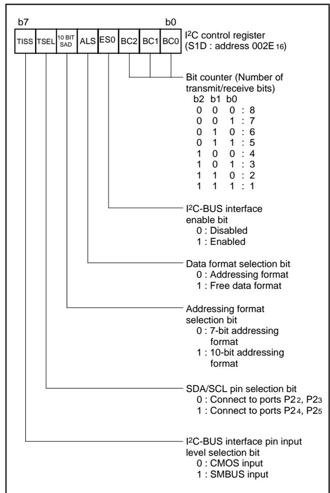
Fig. 23 Structure of I<sup>2</sup>C control register
