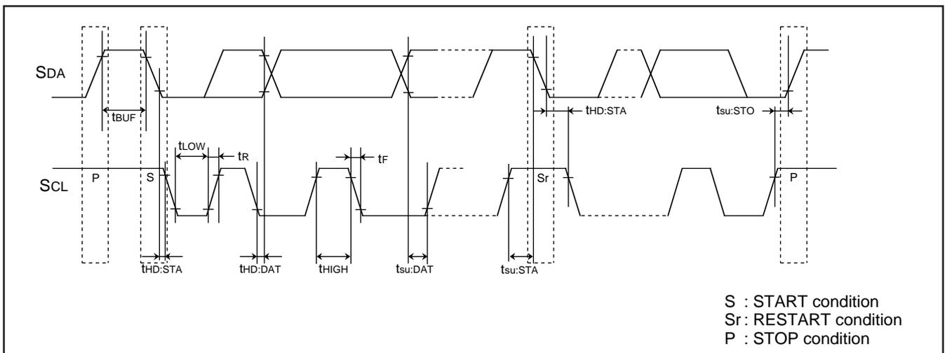
**Fig. 53 Timing diagram of multi-master I<sup>2</sup>C-BUS**
