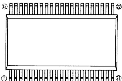
Note1: If the Special Mark is to be printed, indicate the desired layout of the mark in the left figure. The layout will be duplicated as close as possible. Mitsubishi lot number (6-digit or 7-digit) and Mask ROM number (3-digit) are always marked.
