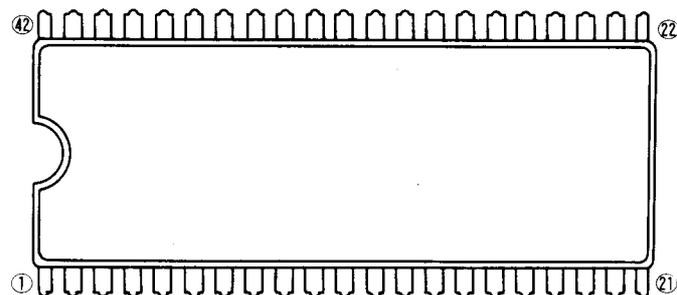
Note1 : If the special mark is to be printed, indicate the desired layout of the mark in the upper figure. The layout will be duplicated as close as possible. Mitsubishi lot number (6-digit or 7-digit) and mask ROM number (3-digit) are always marked.
