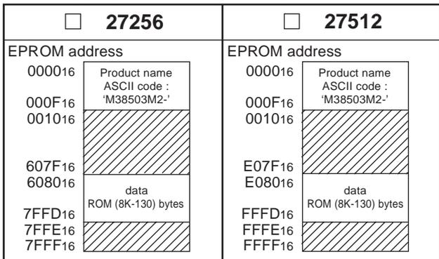
In the address space of the microcomputer, the internal ROM area is from address 6080<sub>16</sub> to FFFD<sub>16</sub>. The reset vector is stored in addresses FFFC<sub>16</sub> and FFFD<sub>16</sub>.
