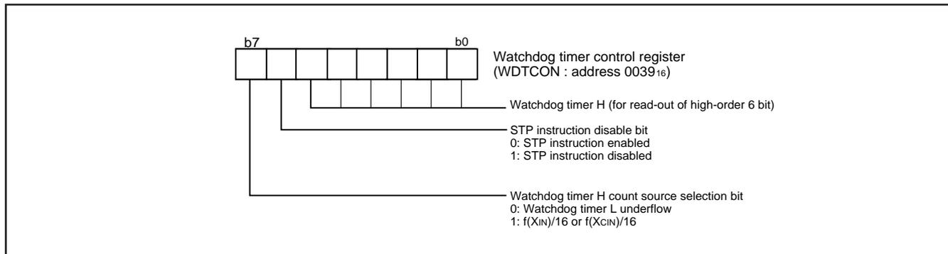
Fig. 28 Structure of Watchdog timer control register
