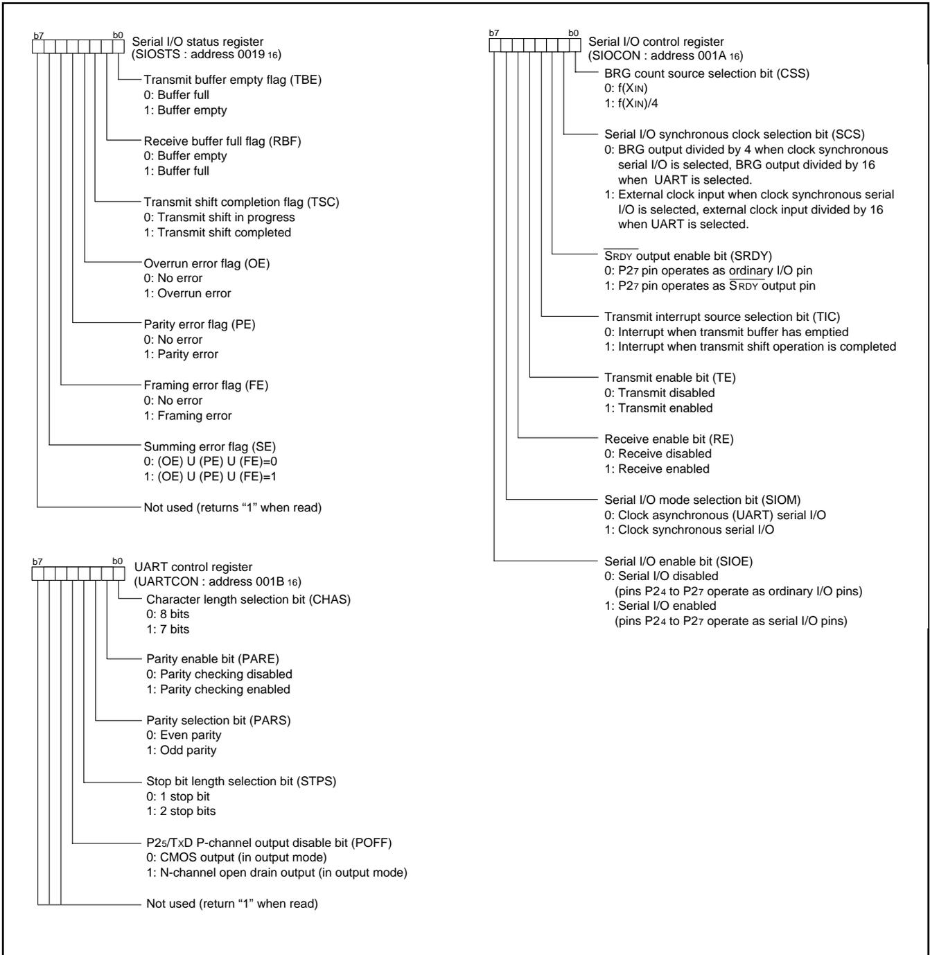
Fig. 19 Structure of serial I/O control registers
