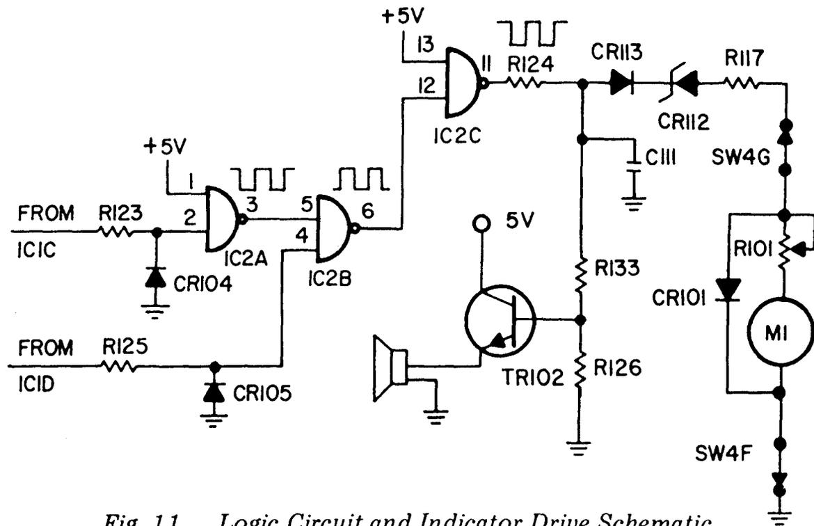
Fig. 11 Logic Circuit and Indicator Drive Schematic
