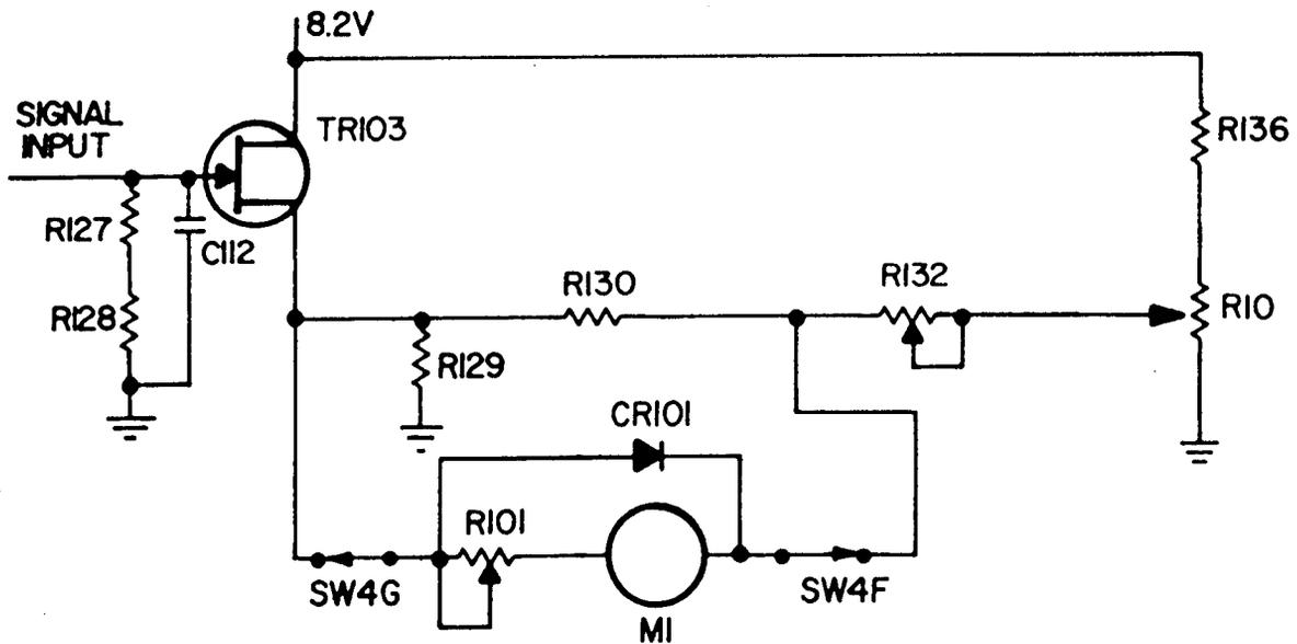
*Fig. 6 Tube-test Bridge Circuit*
