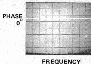
*This indicates that the electrical lengths in the incident and reflected channels of the reflectometer are equal.*
