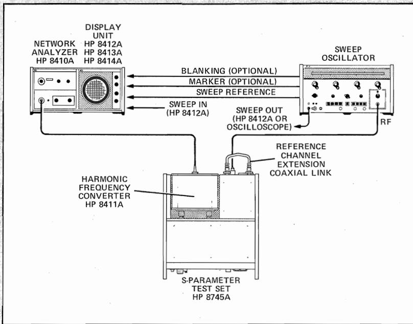
Figure 3-1. Cable Connections When Using the 8745A
