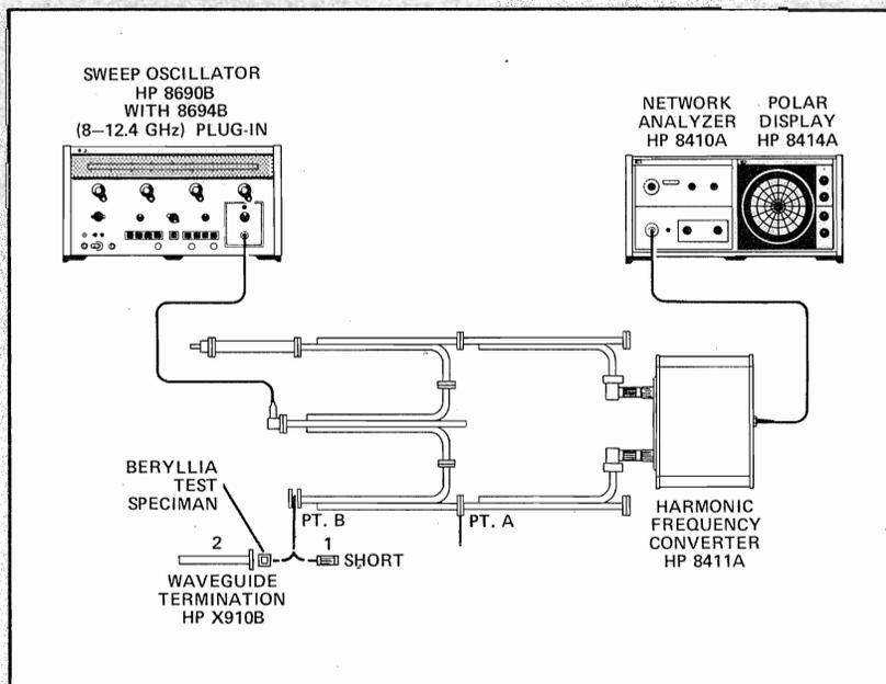
Figure 7-6. Equipment Setup
