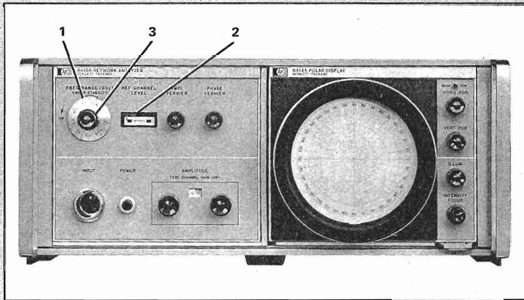
1. Set sweep of source for an octave band within the frequency range of interest, e.g., 1–2 MHz, and sweep speed to 0.01 sec.
