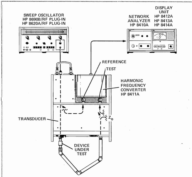
Figure 2-1 (b). Transmission Measurement Using
