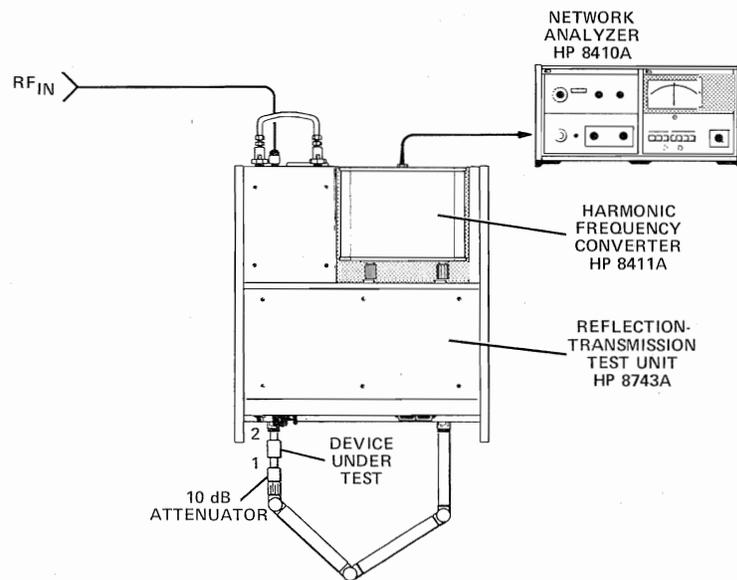
b) Setup for Measuring  $S_{22}$  and  $S_{12}$
