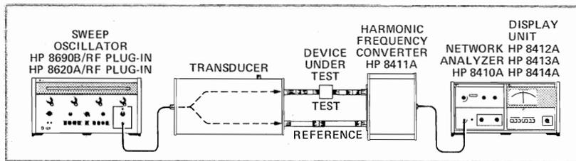
Figure 2-1 (a). Transmission Measurement Using
