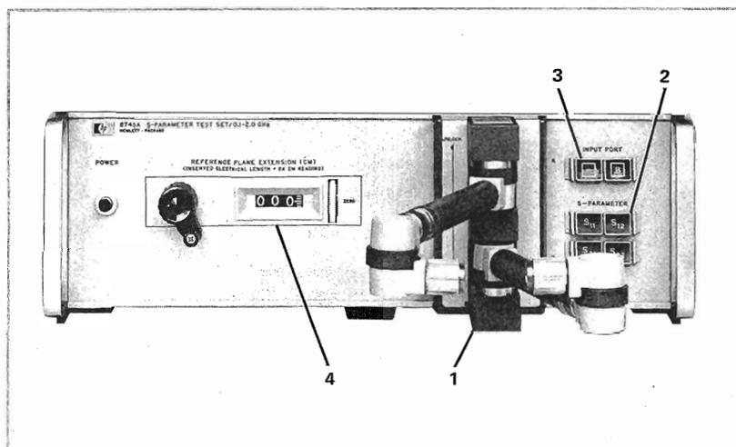
Figure 4-1. The HP 8745A S-Parameter Test Set
