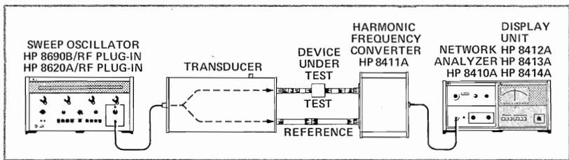
There are three plug-in display devices available. These units give the user a choice of convenient and varied read-outs of the processed information. In addition, peripheral equipment, such as an oscilloscope or X-Y recorder, can be tied into the system.
