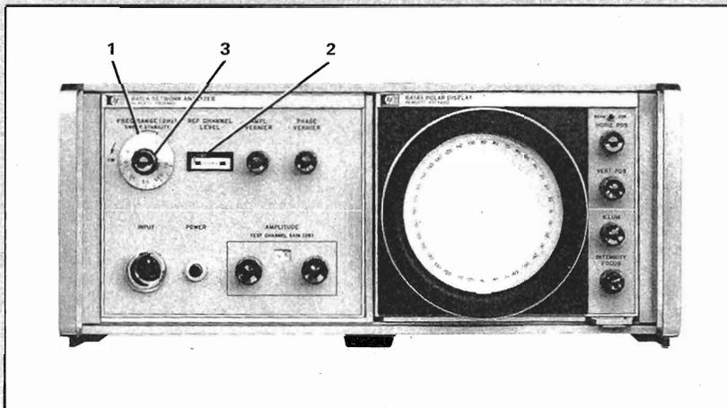
1. Set sweep of source for an octave band within the frequency range of interest, e.g., 1-2 GHz, and sweep speed to 0.01 sec.
