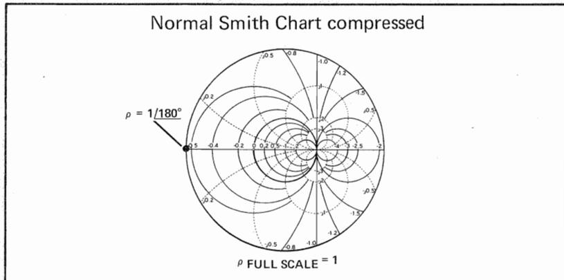
6. Since a tunnel diode with negative resistance has a reflection coefficient greater than one, reduce the 8410A test channel gain by 10 dB. This makes the outer circle equal to a reflection coefficient of 3.16.
