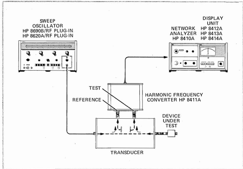
Figure 2-2. Reflection Measurement
