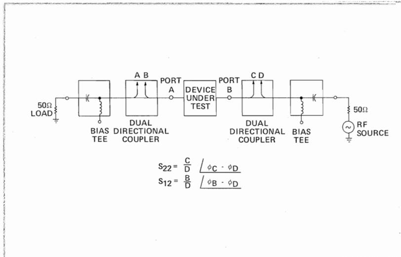
Figure 4-3. Setup for Measuring  $S_{22}$  and  $S_{12}$
