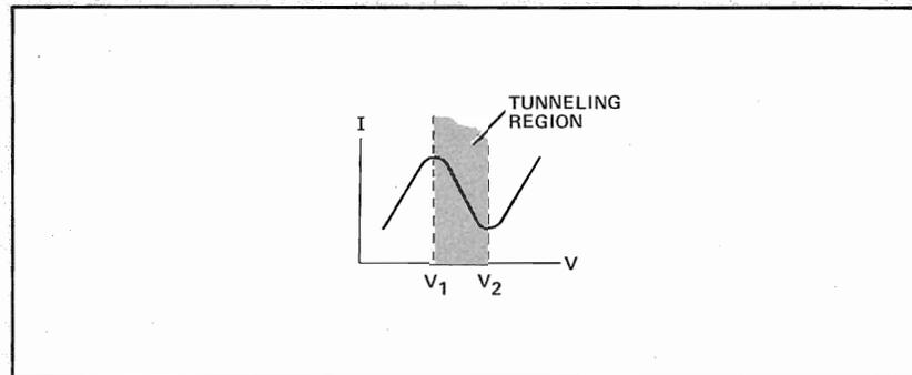
By using markers on the sweep oscillator, the frequency at which tunneling ceases can be determined. To do this, bias the diode for tunneling again and then raise the RF frequency to sweep between 250-500 MHz. By using a marker on the 8690B, the frequency at which  $S_{2,2} = 1$  can be determined.
