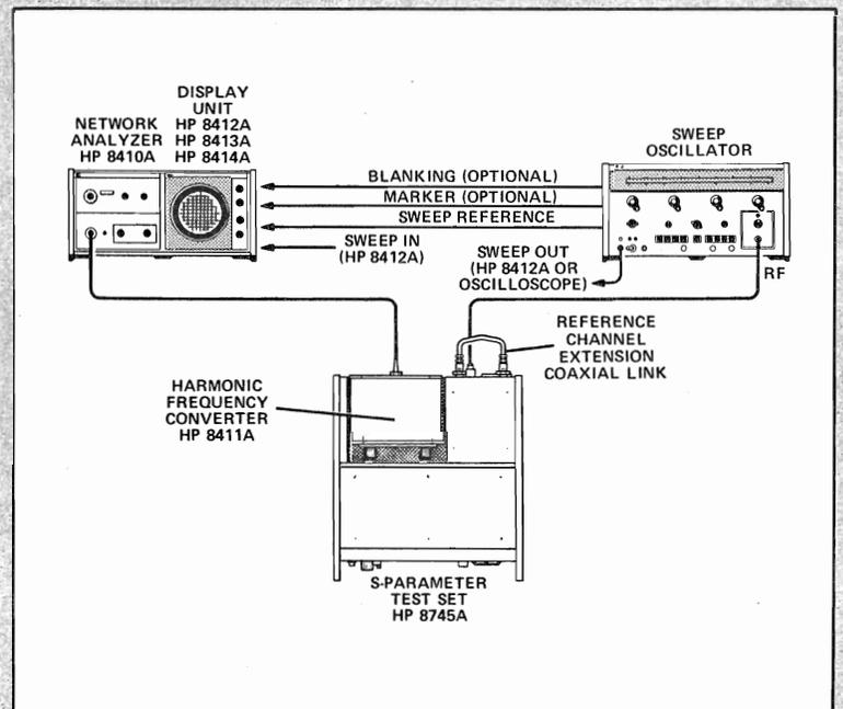
Figure 1. Cable Connections When Using the 8745A
