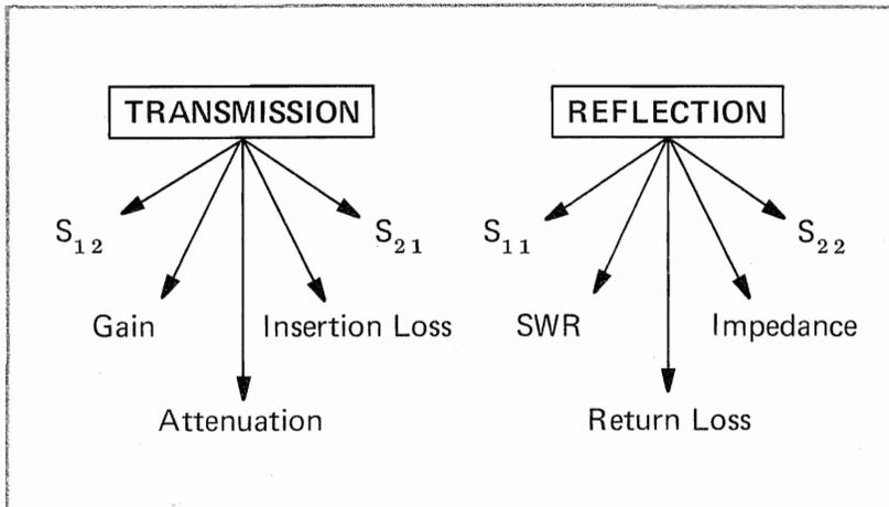
*Figure 1-9. Network Parameters from Transmission & Reflection Measurements*
