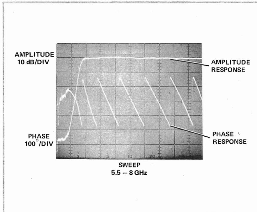
Figure 1-6. Typical Output Display for a Bandpass Filter
