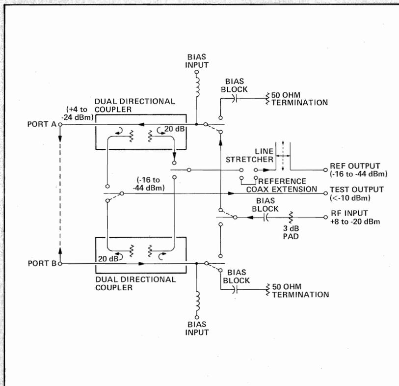
Figure 4-14. Simplified 8745A RF Schematic Diagram
