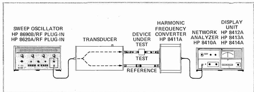
In these basic test setups, the RF signal source shown is the HP 8690B/8620A Sweep Oscillator with the 8690/8630 series RF plug-ins. While all HP sweep oscillators are designed to provide optimal results with the network analyzer system, however, other sweep oscillators are usable if they meet the following specification:
