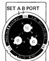
This means that the 8745A Port A is the port connected to the transistor input.
