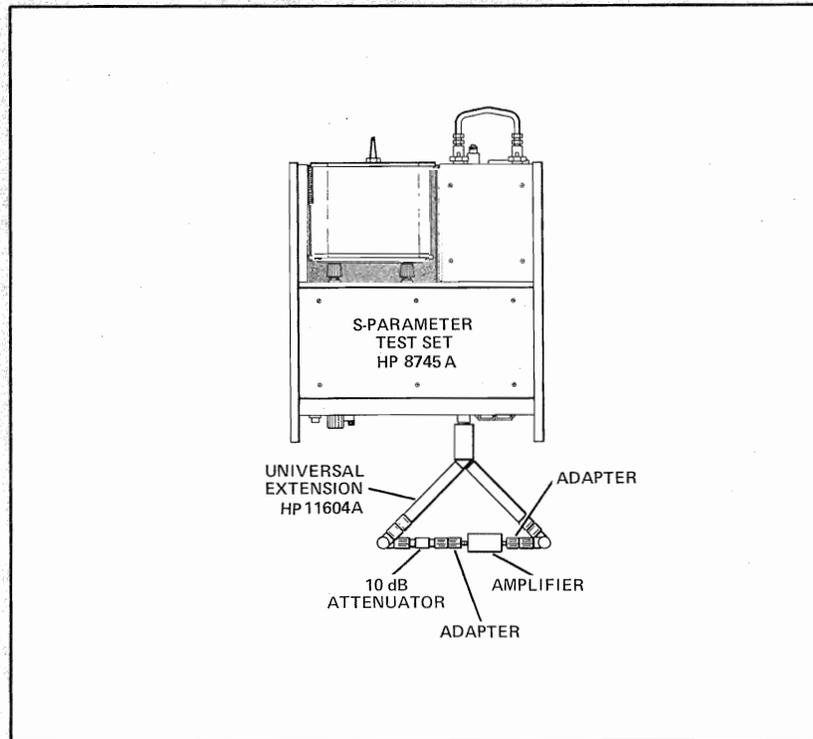
Set the proper bias level according to the amplifier specifications. The gain is measured on the 8412A Phase-Magnitude Display. The nominal gain of 40 dB is observed. The biasing voltages are then turned off.
