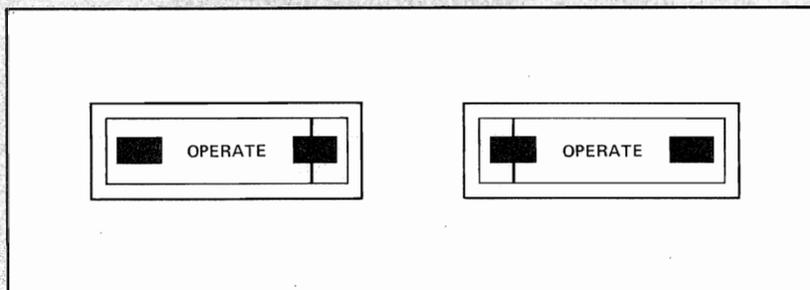
during this test, reduce power from the sweeper. If the needle moves into the left black portion, this could indicate that the system is dropping out of phase lock. Increase RF power or readjust sweep stability control.
