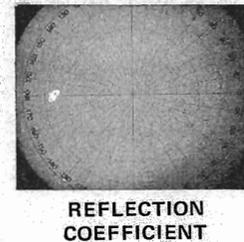
Set Degree Offset switch on 8412A (No. 6) to  $180^\circ$  and increase resolution to  $1^\circ/\text{div}$  for this step.
