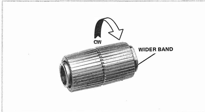
2. **IMPORTANT:** Part the connectors carefully to prevent striking the inner conductor contact.
