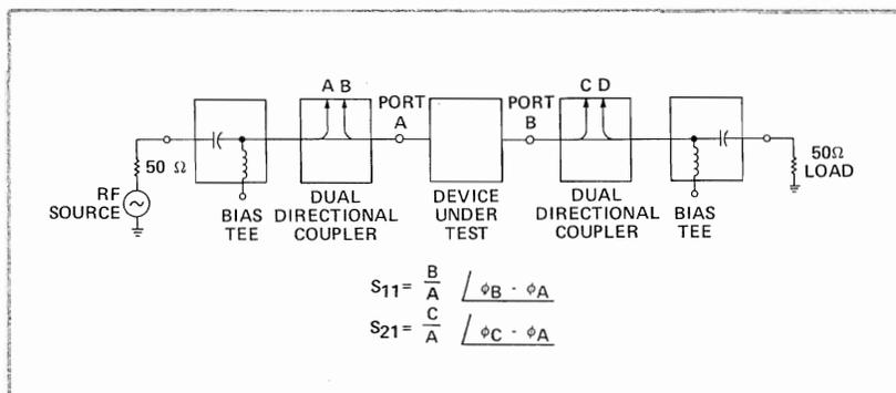
Figure 4-2. Setup for Measuring  $S_{11}$  and  $S_{21}$
