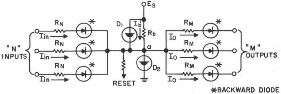
**CHOW'S ANALOG-THRESHOLD LOGIC CIRCUIT**
