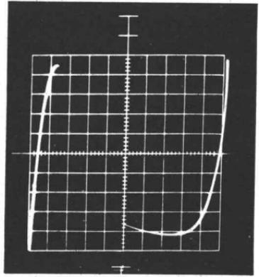
cessive series inductance in the test circuit. As the sweep goes through the negative conductance region, this inductance will resonate with the diode and circuit capacitances, making the circuit oscillate and causing a display as shown in Figure 7.2.
