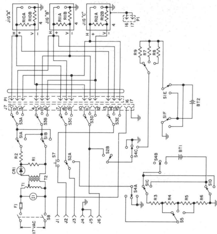
V-I CURVE TRACER CIRCUIT DIAGRAM
