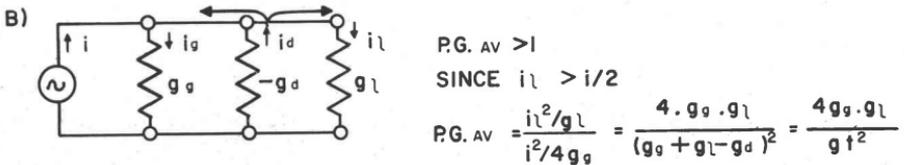
**POWER TRANSFER HAVING NEGATIVE CONDUCTANCE IN CIRCUIT**
