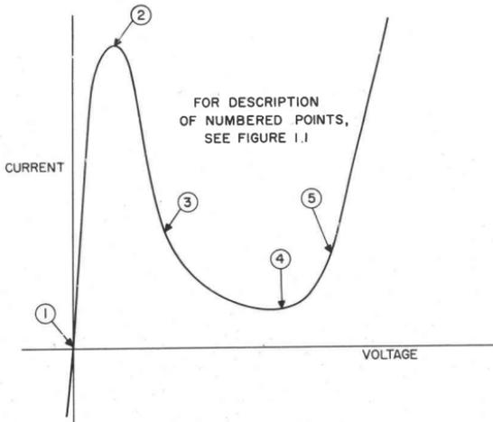
**TUNNEL DIODE CHARACTERISTIC**
