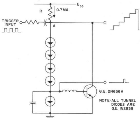
**SERIES CONNECTED TUNNEL DIODES USED FOR 5:1 PULSE
