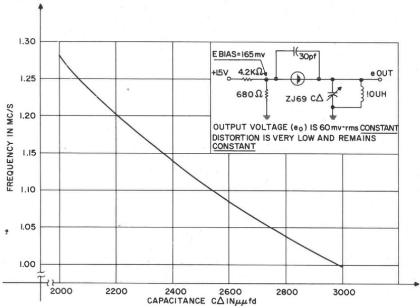
**FREQUENCY TUNING BY MEANS OF  $C_{\Delta}$**
