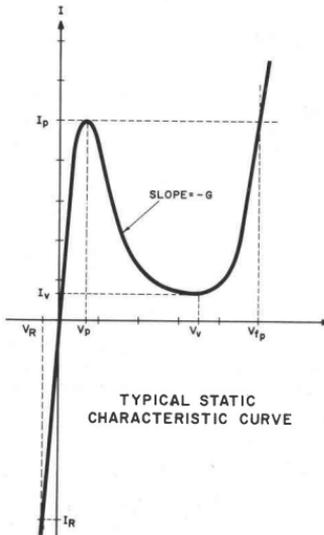
TYPICAL STATIC CHARACTERISTIC CURVE
