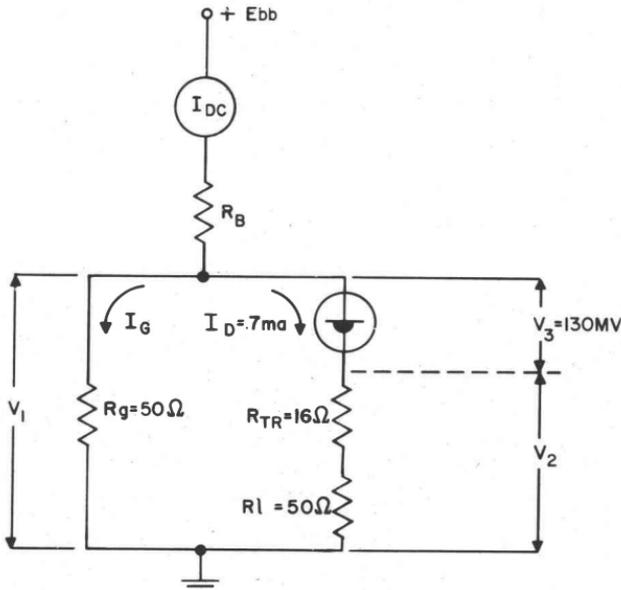
**DC BIAS CIRCUIT FOR 100 Mc/s AMPLIFIER STAGE**
