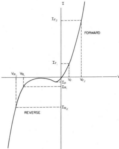
TYPICAL STATIC CHARACTERISTIC CURVE
