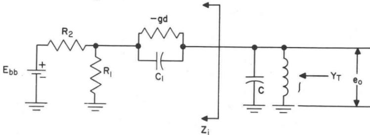
**SIMPLIFIED EQUIVALENT CIRCUIT OF "SERIES-PARALLEL" SINEWAVE OSCILLATOR**
