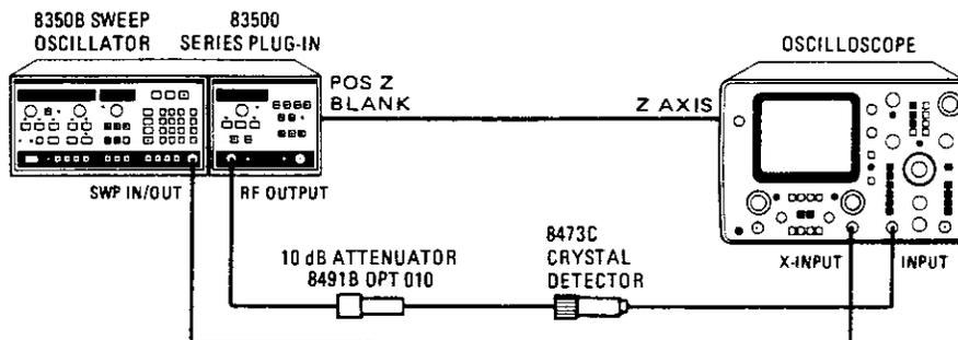
Connect the equipment listed above as shown in the above diagram. Select External Sweep on oscilloscope.
