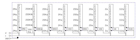
Figure 2 Model DB877 Schematic
