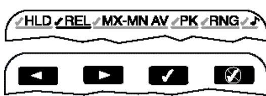
Either **◀** or **▶** key engages the menu bar in the display and moves the cursor (underline) left or right. While the cursor is under the desired function, press the **✓** key to activate that function. A check mark appears to its left. To deactivate an active function, press the **✗** key while the function is selected on the menu bar (underlined). Press **✗** key twice to deselect all menu functions.
