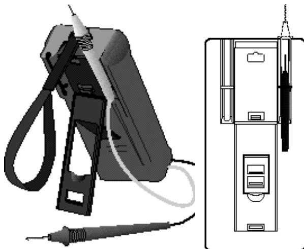
Your shipping carton should include the multimeter, a holster, one test lead set (one black, one red), one 9V battery (installed) and this manual. If any of the items are damaged or missing, immediately return the complete package
