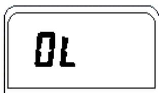
Range Overload is indicated by "OL" and a continuous tone. Take immediate steps to remove the cause of the overload. Select the next higher range until a value is displayed. If overload still exists in the highest range, remove test leads from the measurement setup as it is beyond the range of the meter. Overload indication is normal in the OHMS and continuity ranges when the leads are not connected to anything or when the measured value is higher than the selected resistance range.
