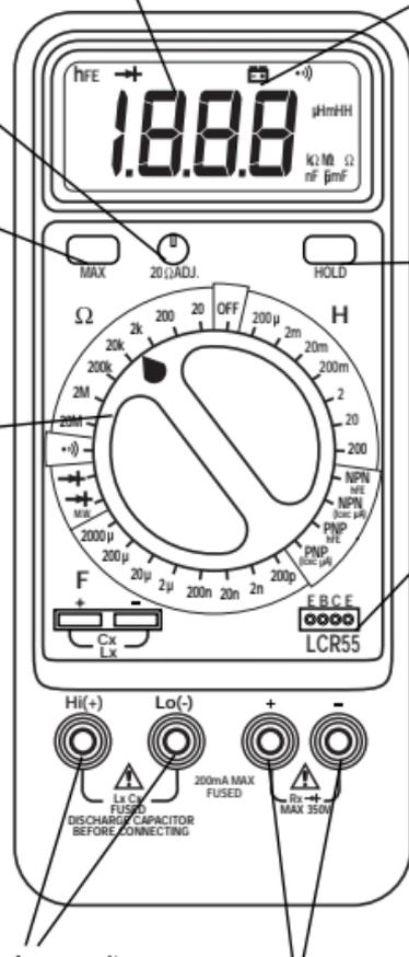
High (+) and Low (-) inputs for capacitance
