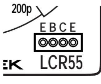
The Transistor must be out of circuit. ❶ Set the Function/Range switch to the PNP(hFE) or NPN(hFE) position, according to the type of transistor to be measured. ❷ Plug the emitter, base and collector leads of the transistor into the correct holes of test socket. ❸ Read the  $h_{FE}$  beta, (DC current gain) in the display.
