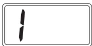
Range overload is indicated by "OL" in the display. Take immediate steps to remove the cause of overload. Select higher range. If in highest range, interrupt measurement. Overload indication is normal in the OHMS range with open circuit or too high a resistance.
