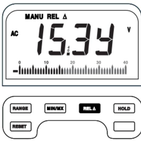
With a measured value on the display, press REL to enter the Relative Mode. "REL Δ" appears on display, the displayed reading is memorized as reference value and the display resets to zero. For the next measurements, the display shows the difference between the new value and the stored reference value. Range Lock also works in Relative Mode. Press and hold down
