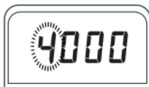
Range Overload is indicated by a flashing "4" (MSD) and three non-flashing zeros (plus a beep tone for voltage, capacitance and current). Take immediate steps to remove the cause of the overload. Select the next higher
