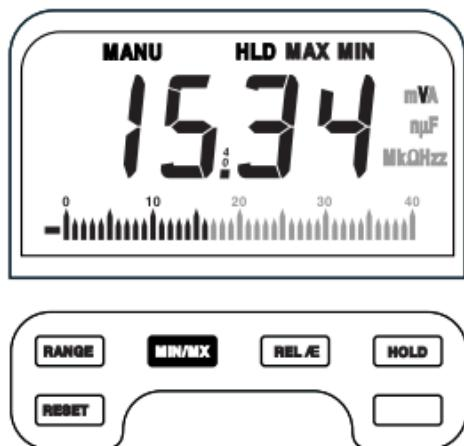
Press MN/MX button to enter MIN Recording mode. The meter switches to manual ranging with HOLD invoked. The last min. value is kept on the display until replaced by a lower reading. Press MN/MX button again to change to MAX recording mode. (MIN or MAX annunciator indicates what value is recorded). Overrange (flashing 4) is displayed when the range is exceeded.
