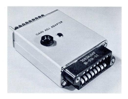
Gain Adjust Adapter—Permits an external calibrating signal to bypass the plug-in preamplifier, for calibrating the sensitivity of the main amplifier of Type 530, 540 and 550-Series Oscilloscopes.
