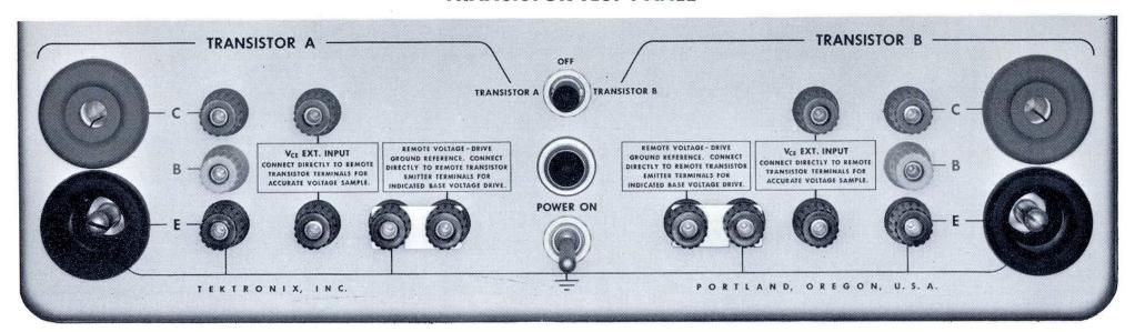
The Type 175 Transistor Test Panel is basically the same as that of the Type 575. Special connectors and cables are provided for high-current applications and for elimination of measurement errors due to voltage drops in high-current carrying leads. The collector,
