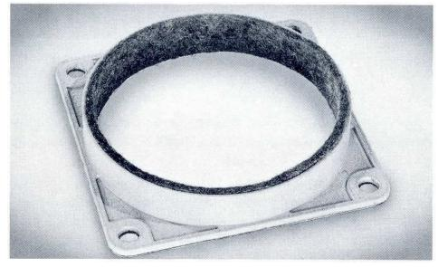
**Bezel**—For mounting cameras, other than Tektronix types, on Tektronix 5" oscilloscopes. Dimensions— $5\frac{7}{8}$ " square; ring  $\frac{7}{8}$ " deep, diameter  $5\frac{5}{8}$ " outside,  $5\frac{1}{8}$ " inside. Die-cast construction, wrinkle finish, felt lined.
