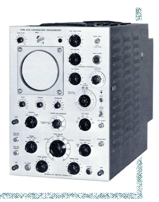
**Signal Delay**—Approximately 65 nsec of delay cable is incorporated in the vertical amplifier. This delay, along with an inherent 55 nsec delay in the amplifier, permits the sweep to start before the signal reaches the vertical deflection plates.
