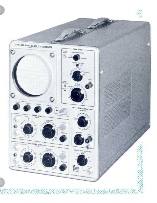
**Calibration Accuracy** — Internal adjustments are provided for setting the gain of both amplifiers. When accurately set, sensitivities at all positions will be within 3% of the panel readings.
