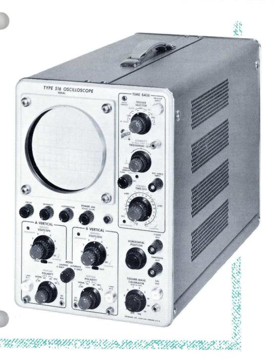
assures uniform beam current for all sweep speeds and repetition rates at any setting of the intensity control. An external crt cathode terminal permits beam-intensity modulation.
