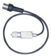
**Calibrator Adapter**—Converts a 50-volt output from the oscilloscope calibrator to 40 millivolts at 50  $\Omega$  impedance, for use in calibrating the gain of the Type N unit. PART NO. 017-010 . . . . . . . . . . . \$15.00
