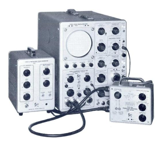
A convenient method of testing fast-switching transistors is shown. Input signal is  $\pm 5$  volts, output is about  $\pm 25$  millivolts. The Type 111 supplies a 10 to 100 kc repetition rate input pulse source. Use of the
