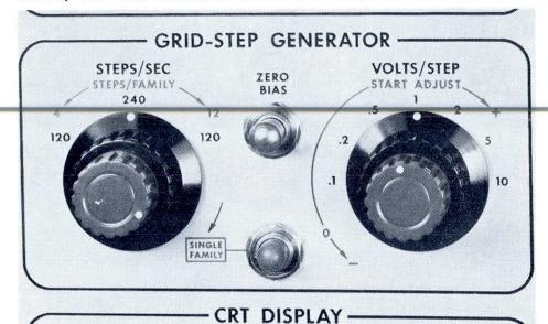
either end of the curves displayed. (When the Type 570 is used with a 50-cycle supply frequency, the step/sec rate will be either 100 or 200.)
