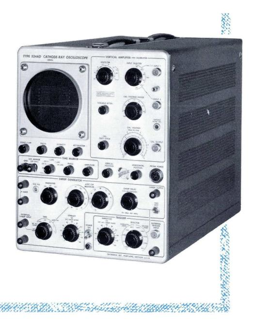
**Sweep Magnifier**—Sweep magnification is obtained by increasing the drive to the sweep-output amplifier by a factor of either 3 or 10. The center portion of the normal sweep is expanded equally to left and right of center. The 3-turn horizontal-position control has sufficient range to cover the entire magnified sweep. Accuracy is within 5%.
