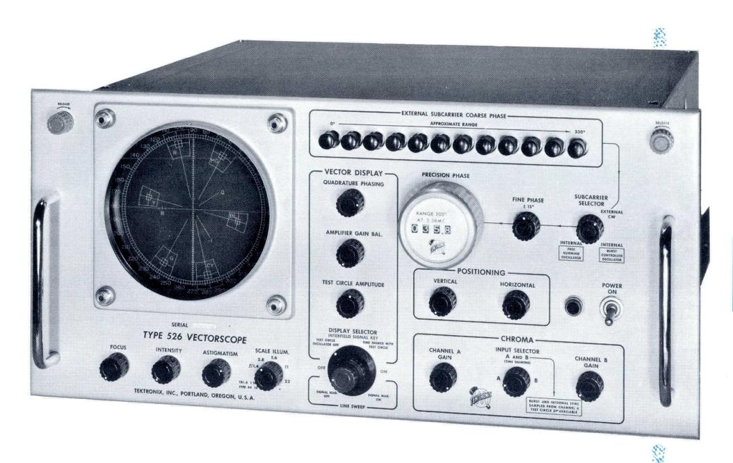
When using the vector display, an internally generated reference signal (test circle) can be fed into either channel A or B to calibrate the instrument, or both channel A and channel B signals can be displayed together for comparison measurements. The signal into a
