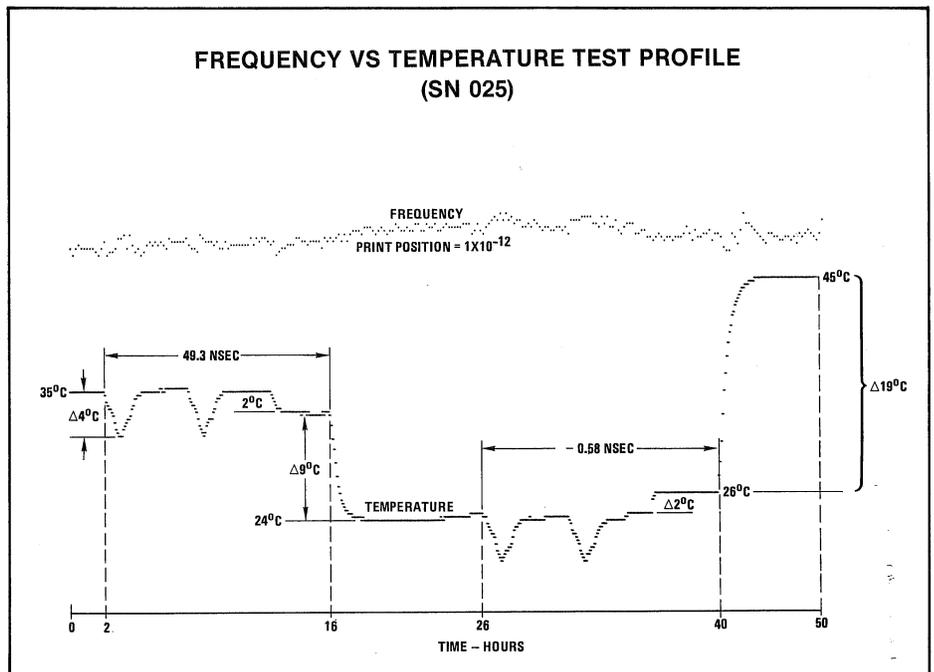
Fig. 9. Clock mounting plate temperature is graphed against the beat periods from the test.
