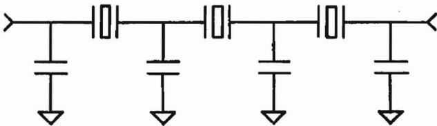
Fig. 3. Simplified circuit of the 30-Hz crystal filter.
