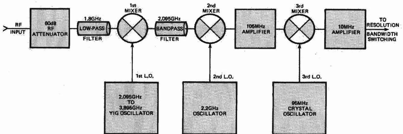
Fig. 1. Frequency conversion system of the 7L13.
