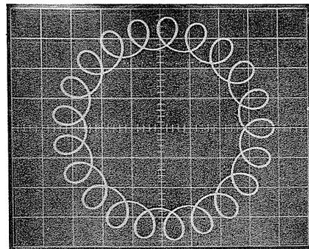
Fig. 3. Roulette pattern for a frequency ratio of 20:1.
