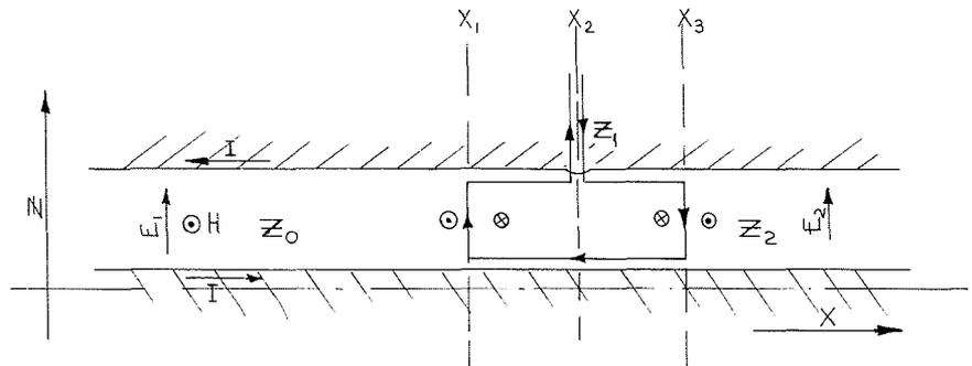
Figure 1. A single-turn winding inserted in the space between the inner and outer conductor of a coaxial transmission line of impedance  $Z_0$ .
