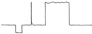
Figure 7.  $\text{Sin}^2$  test signal with dips and bumps caused by frequency response irregularities.
