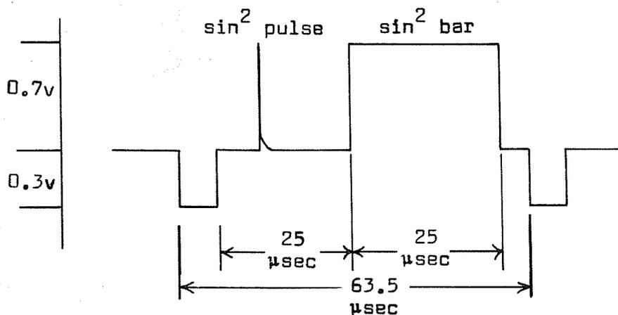
Figure 5. Composite test signal with typical time spacings.
