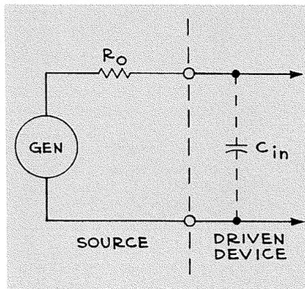
Fig. 2 — Here a signal source has an internal impedance  $R_o$ . The source drives a circuit whose input capacitance is  $C_{in}$ . If the time constant  $R_o C_{in}$  of this arrangement is small, then the risetime of the combination is short. One way to keep the time constant small is to make  $C_{in}$  very small. Then the risetime is short even if  $R_o$  is relatively large.
