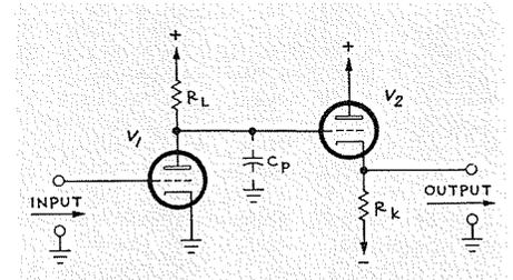
Fig. 11—Here a plate-loaded amplifier  $V_1$  drives the input of a cathode follower  $V_2$ . The plate-to-ground capacitance of  $V_1$  (plus the small input capacitance of  $V_2$ ) is represented by  $C_p$ . The risetime of the coupling circuit between  $V_1$  and  $V_2$  is determined by the time constant  $R_k C_p$ .
