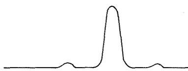
Figure 8.  $\text{Sin}^2$  pulse showing a leading and a trailing reflection or echo.
