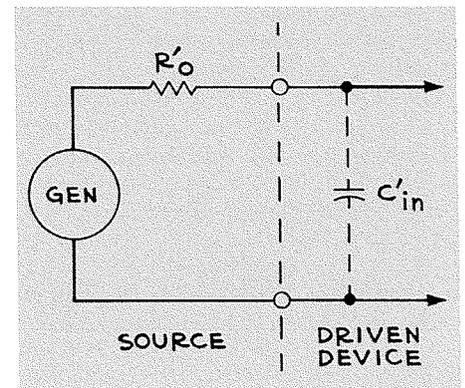
Fig. 3 — Here a second signal source whose internal impedance is  $R'_o$  drives a circuit whose input capacitance is  $C'_{in}$ . One way to keep the time constant  $R'_o C'_{in}$  short is to make  $R'_o$  very small. Then the risetime is short even if  $C'_{in}$  is relatively large.
