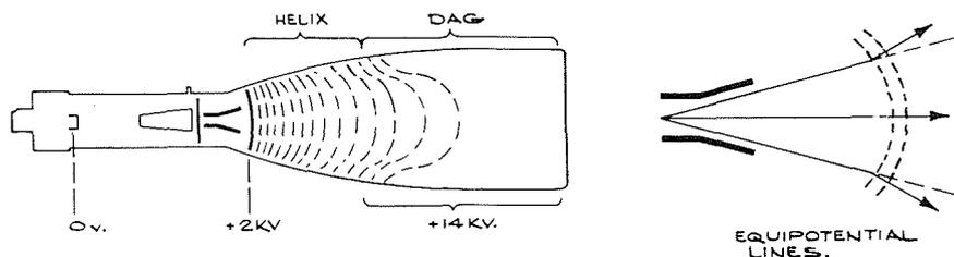
FIGURE 2. MESH-TYPE CRT.
