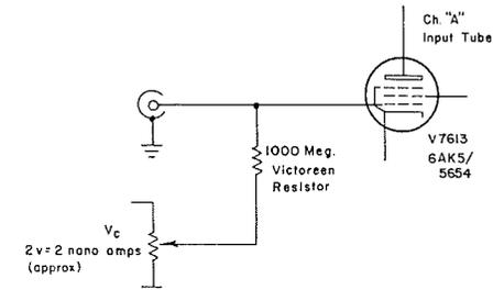
Schematic showing the Type Z Unit input modified to give an input resistance of 1000 megohms.
