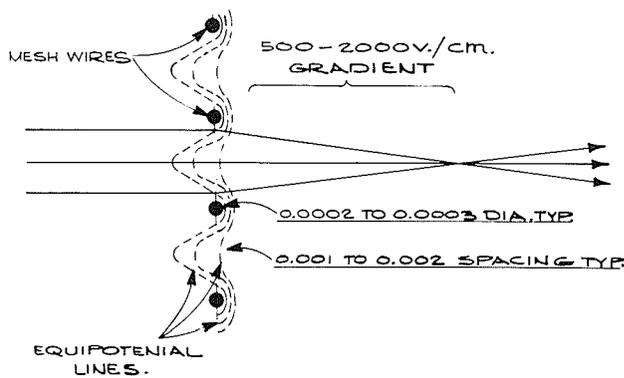
FIGURE 3. ACCELERATION FIELD OF THE MESH STRUCTURE.
