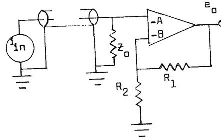
$$R_1 + R_2 = R, R_2 = Z_o, R_1 = R + Z_o,$$
