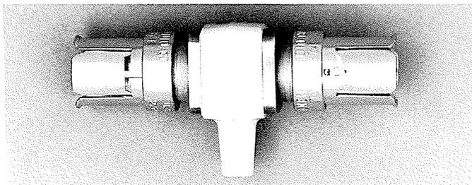
The VP-1 is a 50-ohm coaxial tee with GR fittings on each end and a plastic center collar. The collar is formed to provide a branch for insertion of P6034 10X or P6035 100X low-capacity, miniature passive probes.
