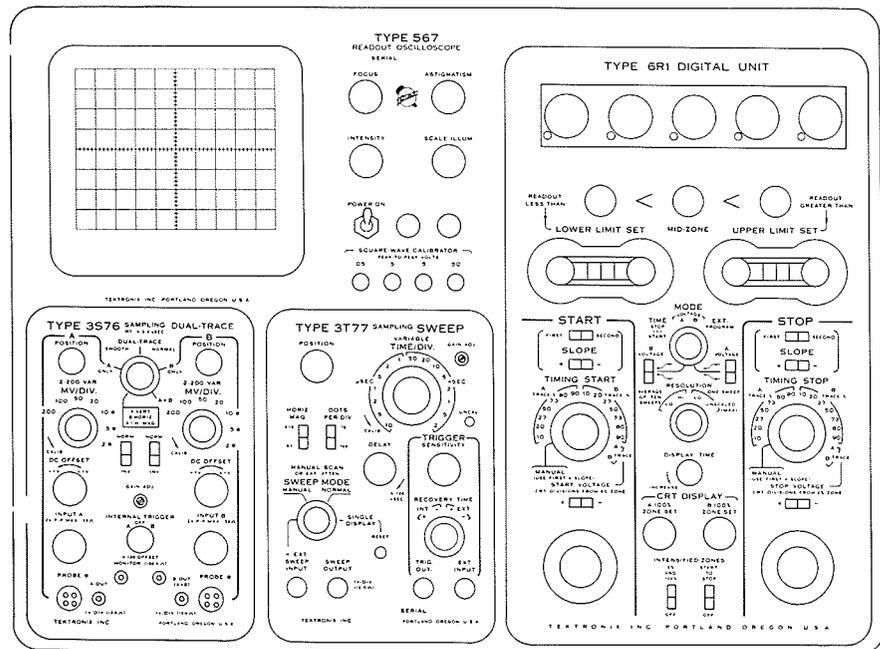
**DATA:** This is a Type 567 Test Set-Up Chart. It provides a ready means of recording instrument control settings for any given test or production set up. A facsimile of the trace resulting from the set up can be drawn on the chart graticule or a picture of the waveform attached to the chart. In the "DATA" space, where this message to you is printed, special instructions or pertinent information concerning the test or production set up can be recorded.
