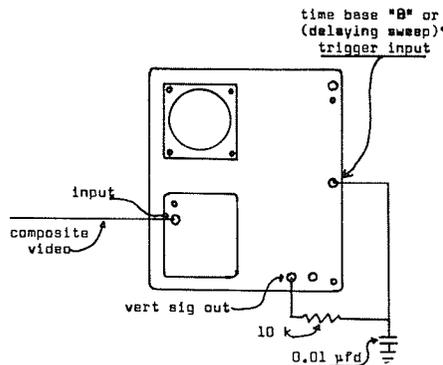
(Note: If available, Field sync pulses are preferable for triggering the Delaying Sweep.)
