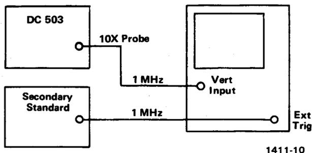
Fig. 3-3. Connections for Time Base frequency check.
