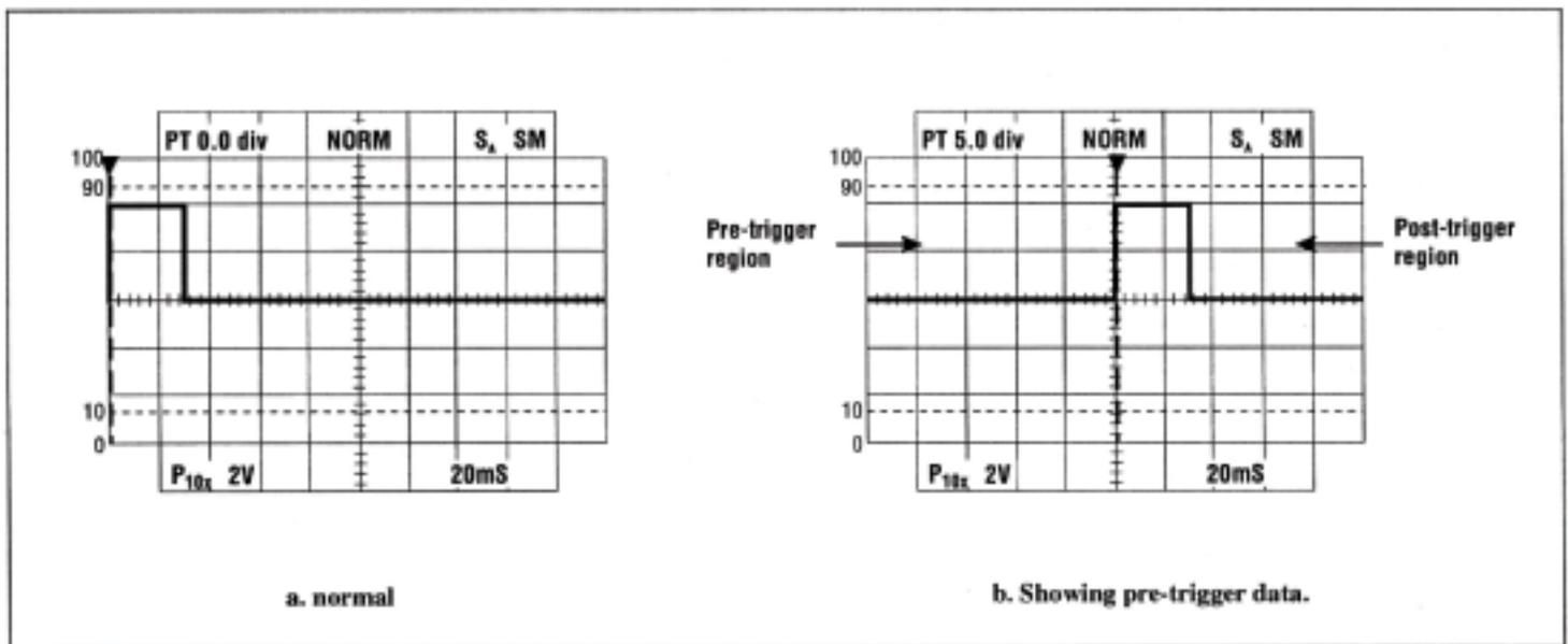
**Fig. 10 Capture of a cone-time event.**
