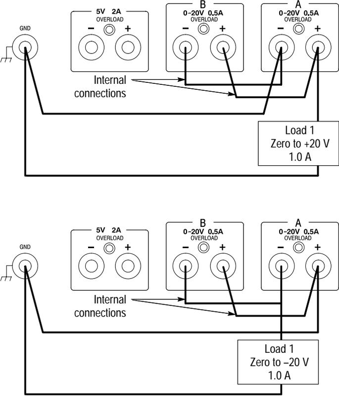
Figure 11: Parallel-Tracking Applications
