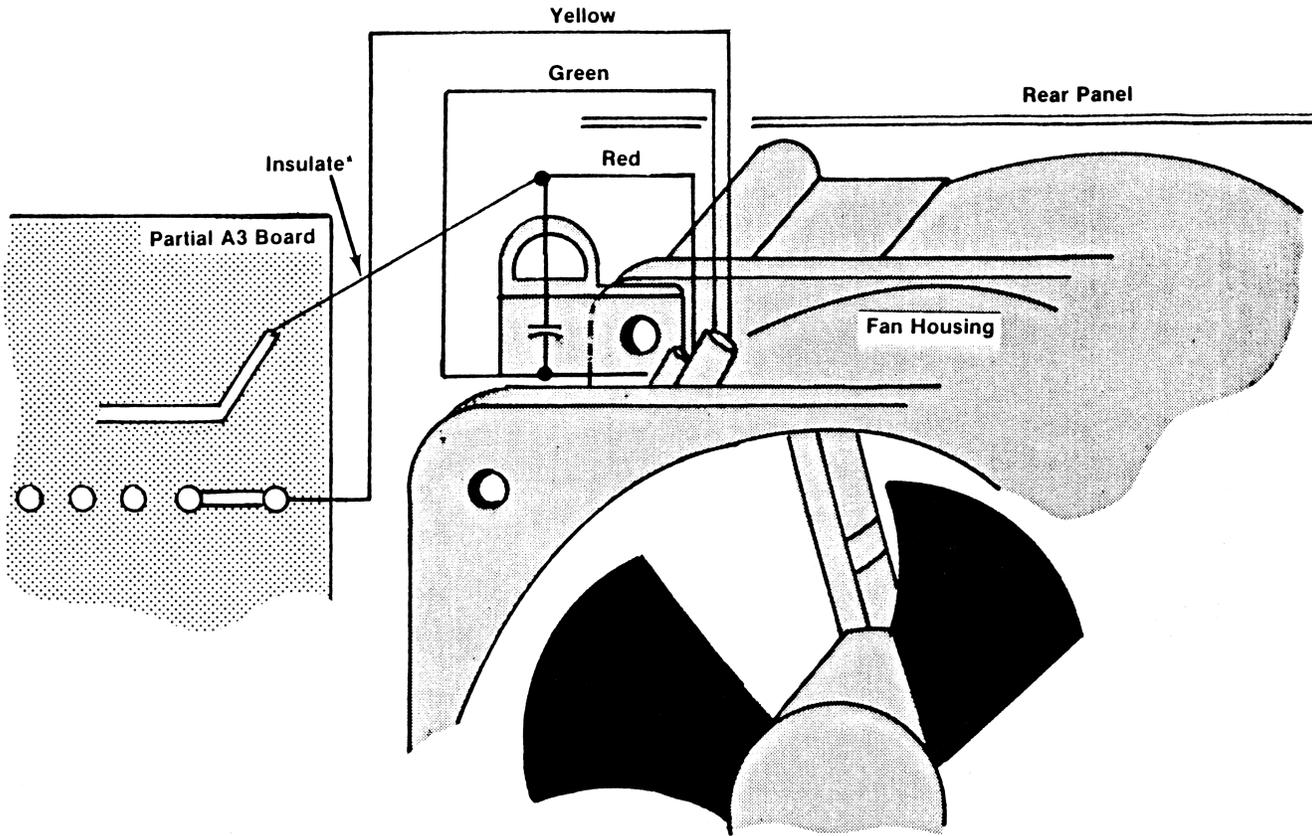
\*Insulate this lead from the capacitor with Tektronix Part No. 162-0026-00.
