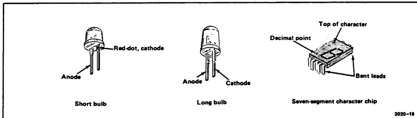
Fig. 3-3. Light-emitting diode (LED) lead orientation illustration.
