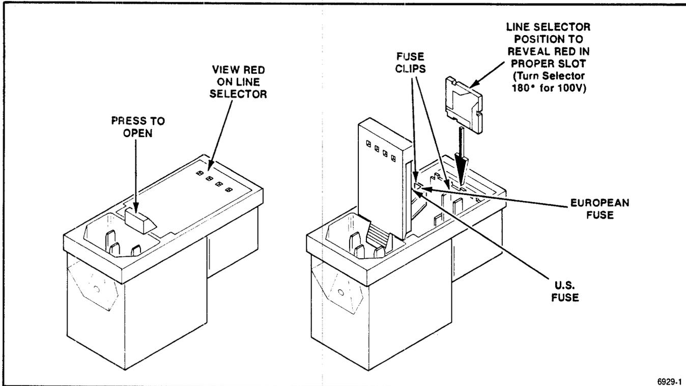
Fig. 2-1. Line Voltage Selection and Main Fuse Replacement.
