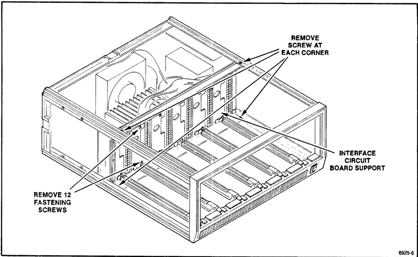
Fig. 3-4. Removal of the interface circuit board support.
