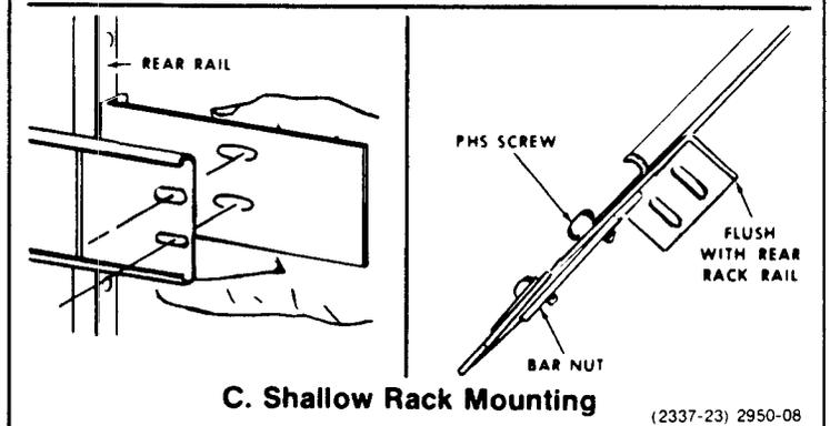
Fig. 2-8. Rackmounting slide details.
