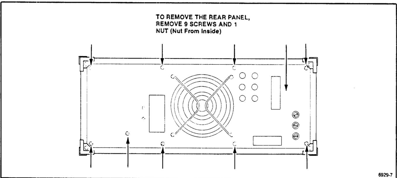
Fig. 3-5. Rear panel removal.
