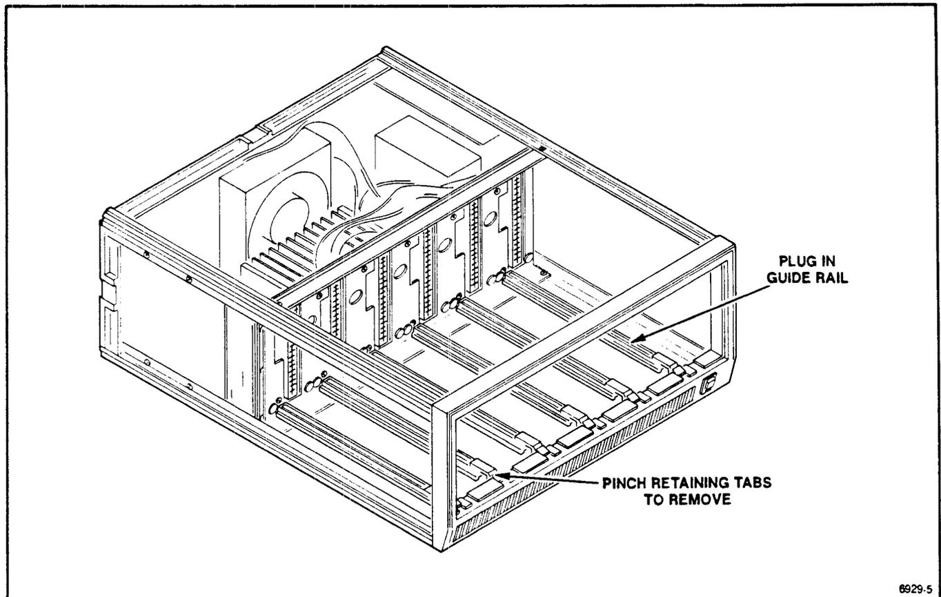
Fig. 3-3. Guide rail and air baffle removal.
