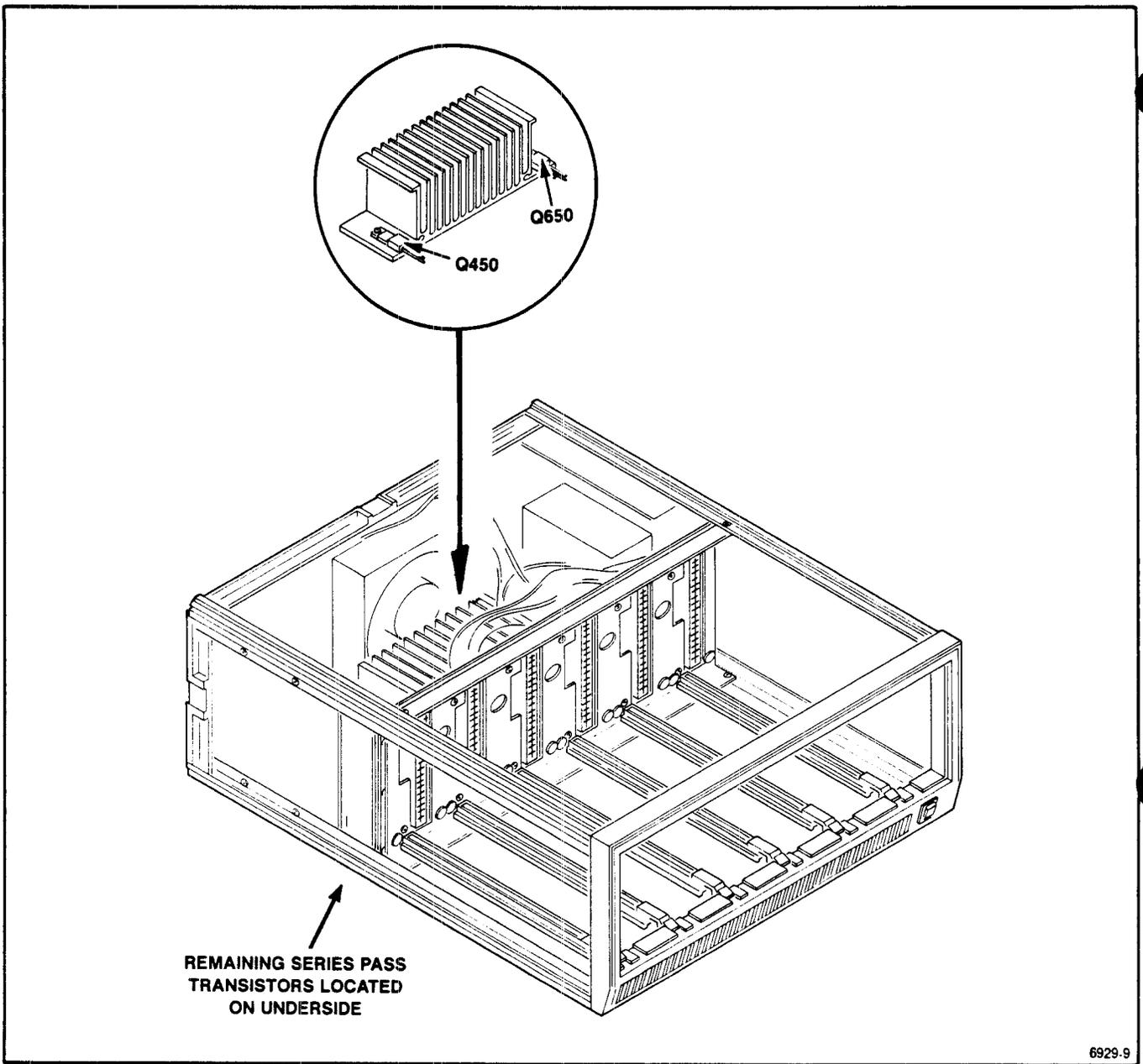
Fig. 3-7. Series pass transistor locations. The high power compartment series pass transistors Q450 and Q650 are on the right side of the heat sink. Q650 is the upper transistor.
