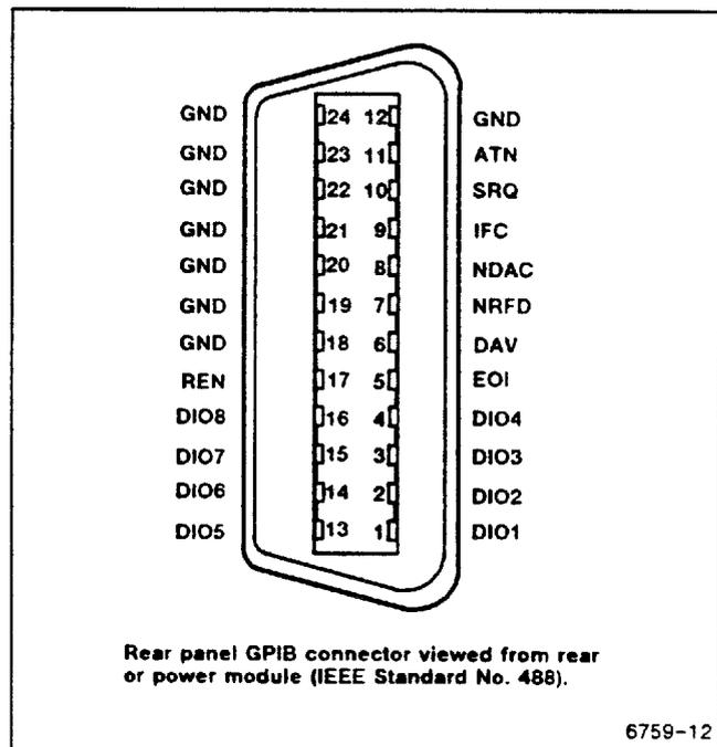
Rear panel GPIB connector viewed from rear or power module (IEEE Standard No. 488).
