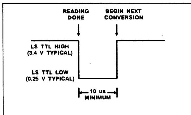
Fig. 2-12. Voltmeter Complete Pulse Specifications.
