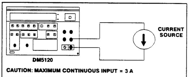
**Fig. 2-9. Current Measurements.**
