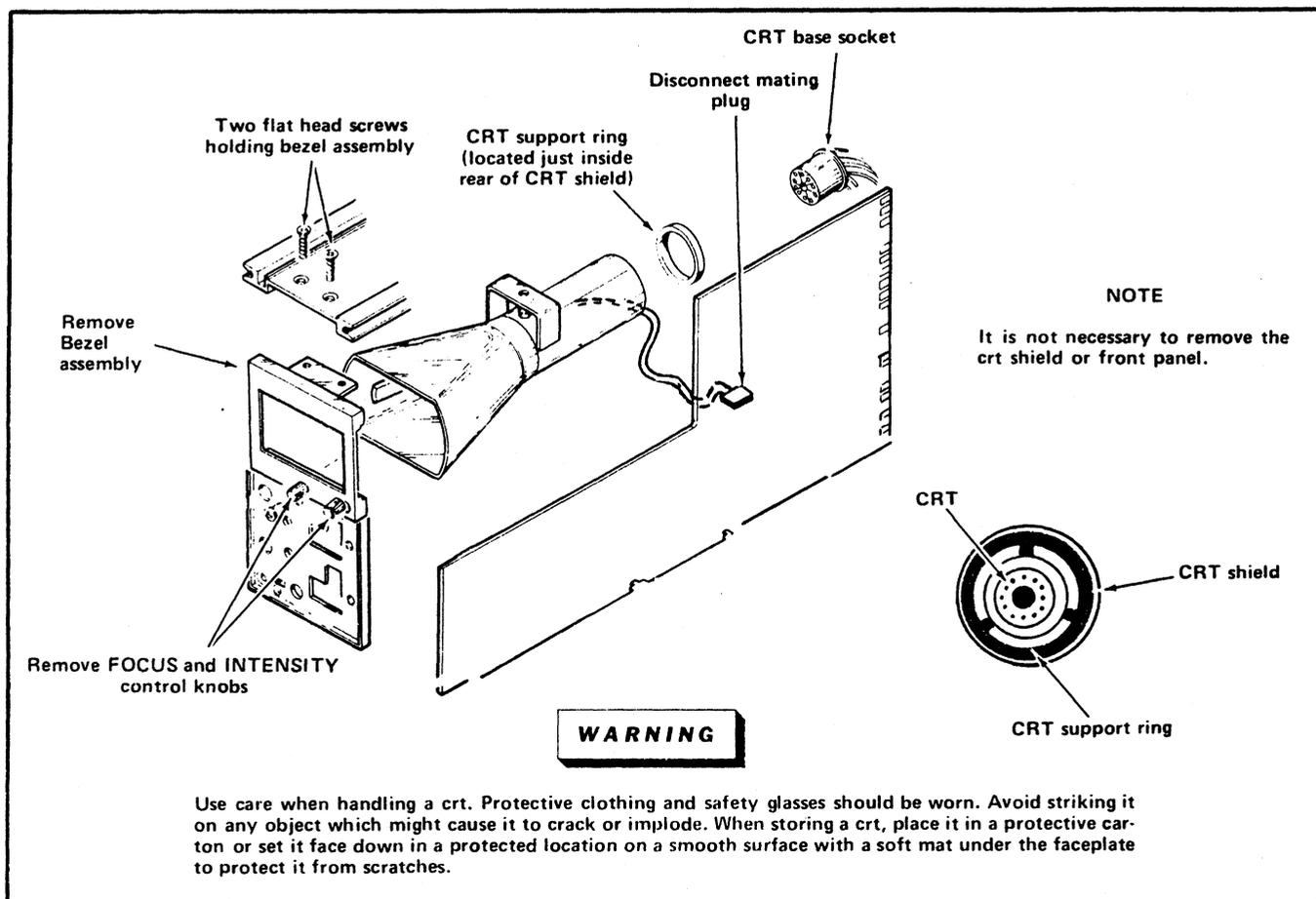
Fig. 4-1. Exploded view drawing identifying several critical parts of the crt area.
