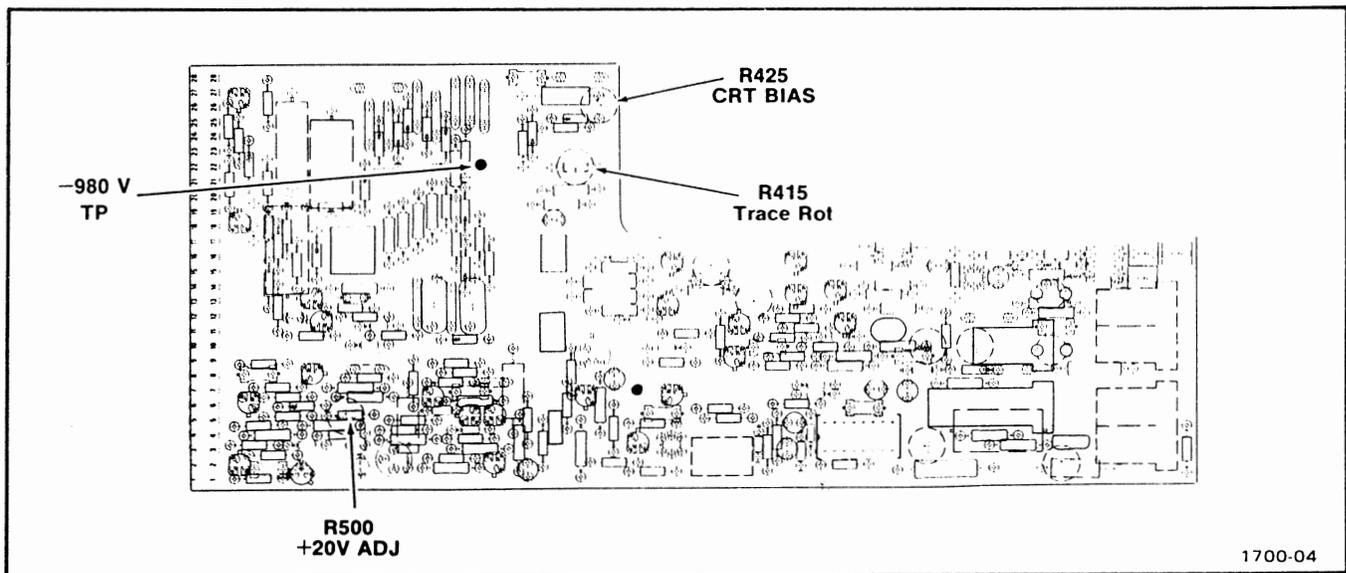
Fig. 3-2. Location of  $-980\text{ V}$  test point;  $+20\text{ V}$ , CRT Bias, and Trace Rotation adjustments.
