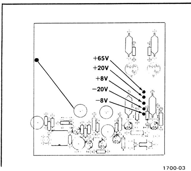
**Fig. 3-1. Location of Power Supply test points.**
