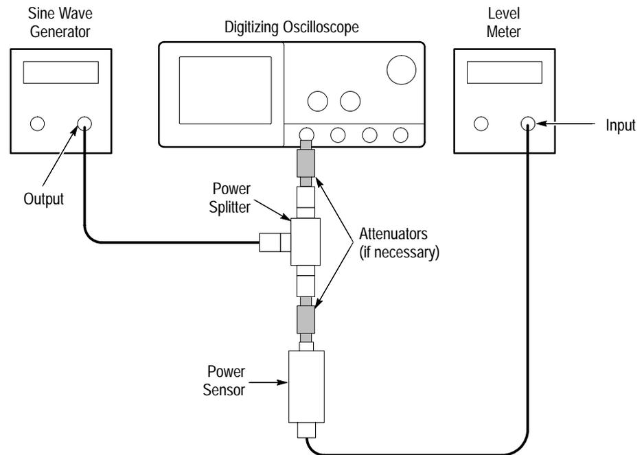
**Figure 4-41: Sine Wave Generator Leveling Equipment Setup**
