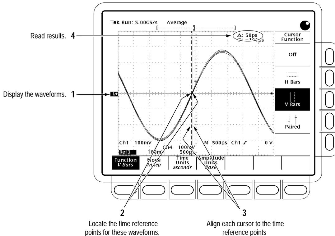
**Figure 4–11: Measurement of Channel Delay – TDS 684B Shown**
