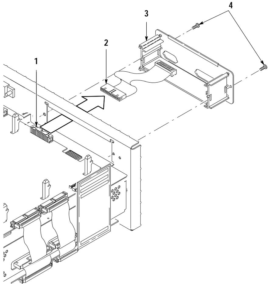
**Figure 6–12: Remove Circuit Board Assembly From Oscilloscope**
