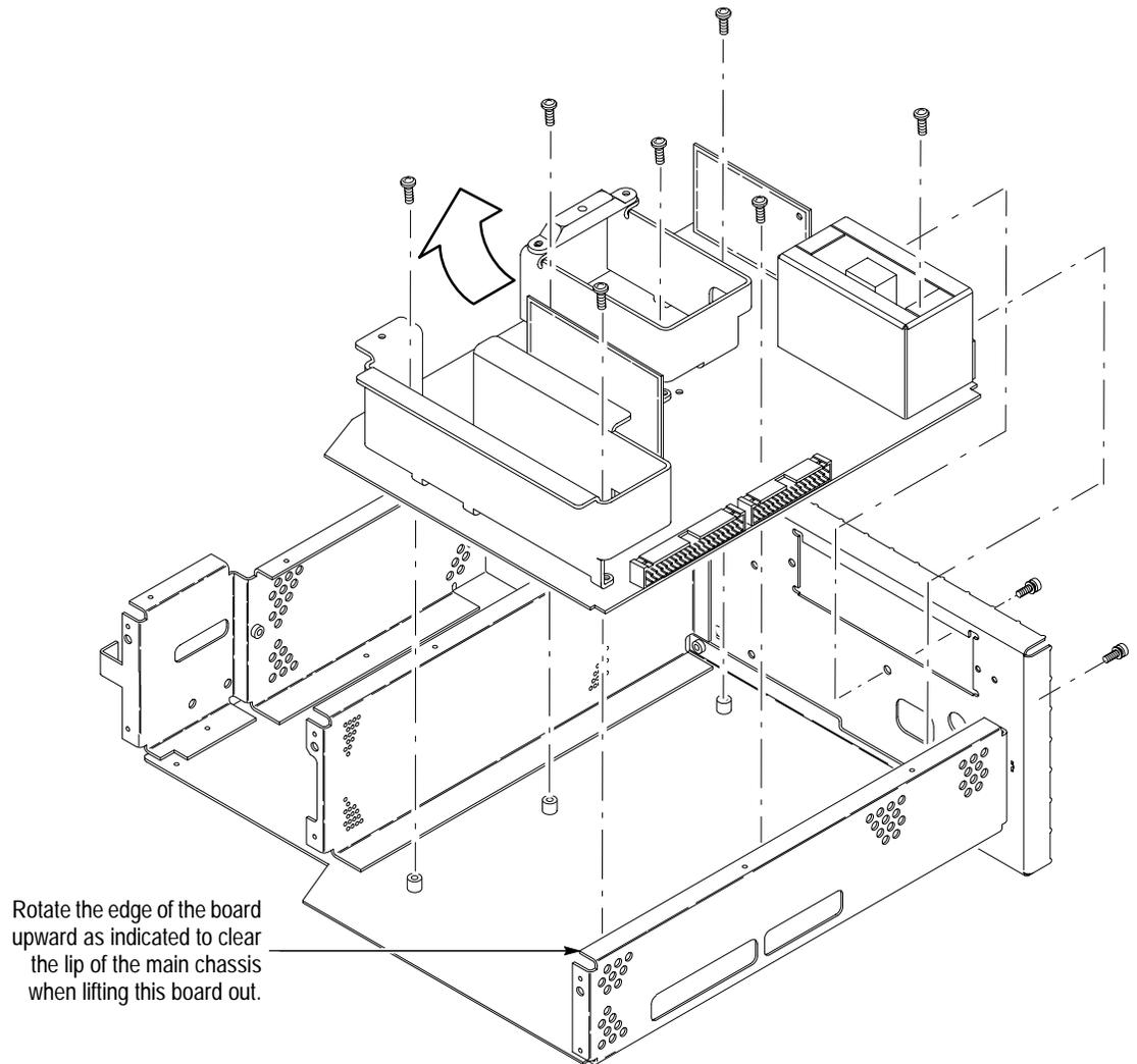
**Figure 6–21: A16 Low Voltage Power Supply Removal**
