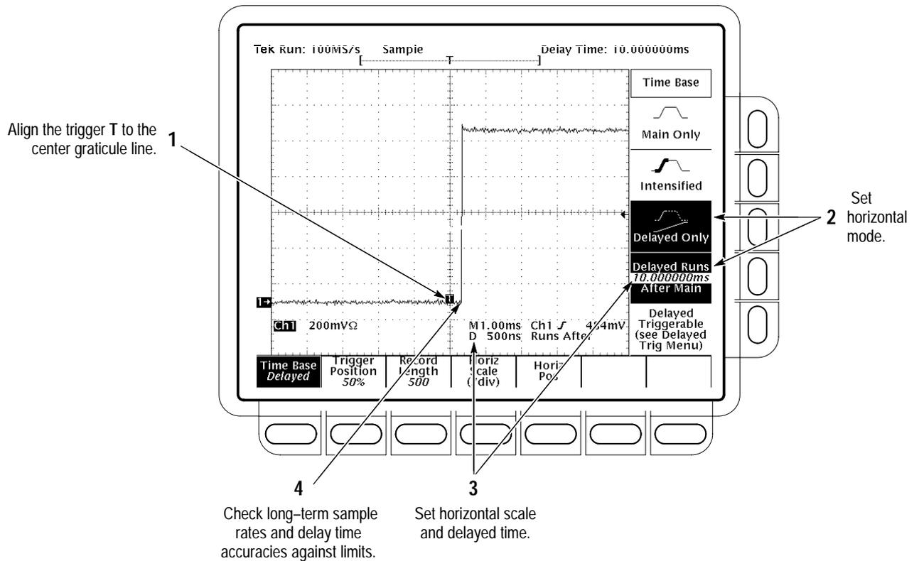
Figure 4-13: Measurement of Accuracy — Long-Term and Delay Time
