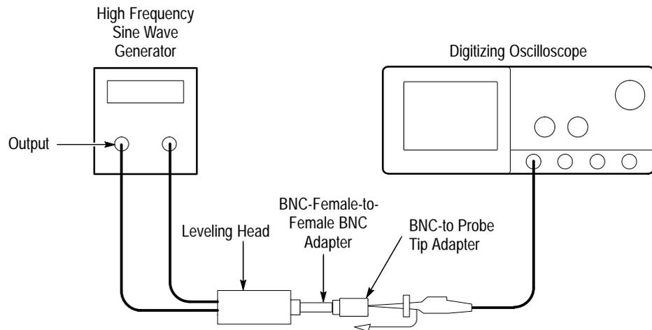
Figure 5–6: Initial Test Hookup
