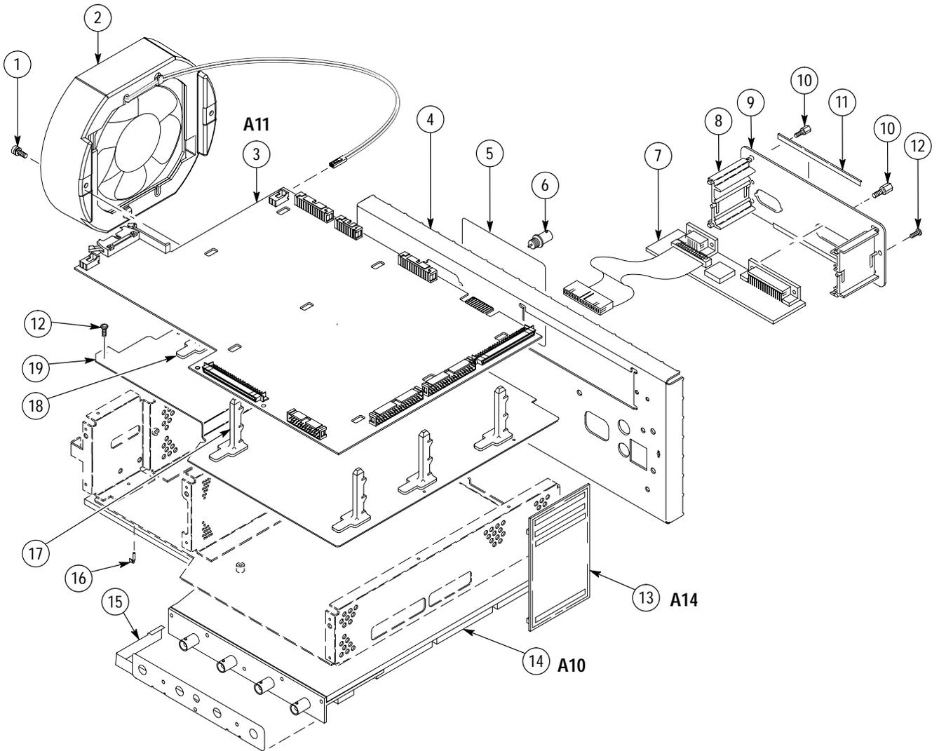
Figure 10-2: Outer-Chassis Modules
