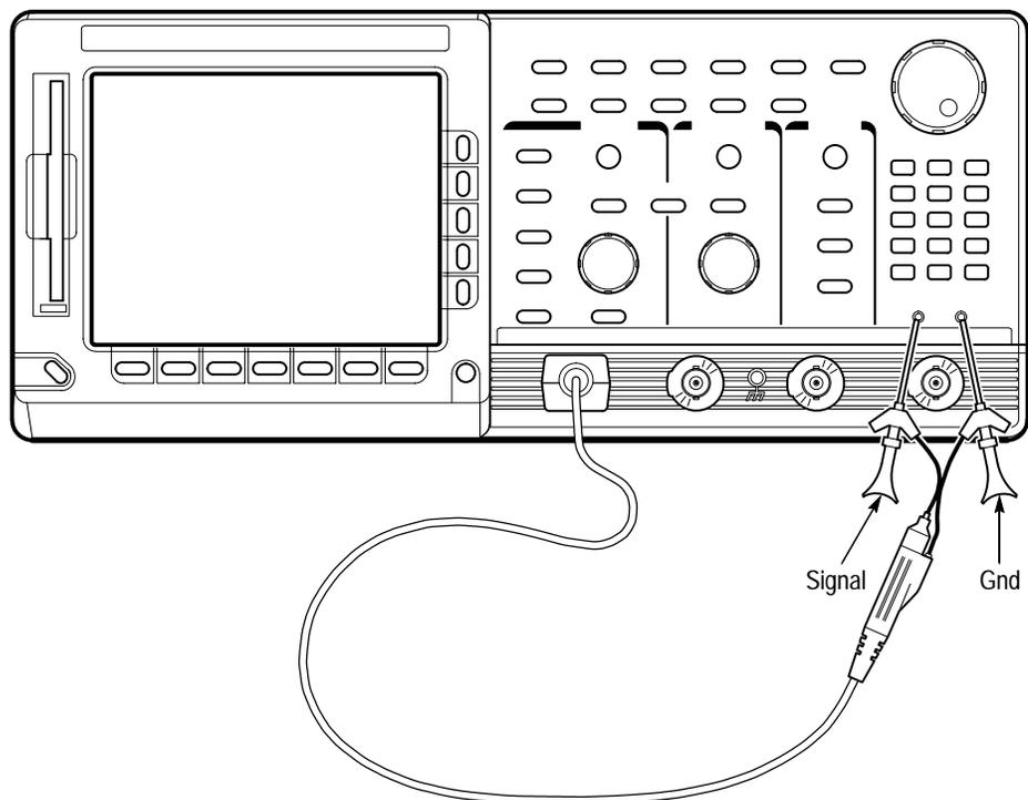
**Figure 4-3: Universal Test Hookup for Functional Tests – TDS 600B Shown****b. Initialize the oscilloscope:**
