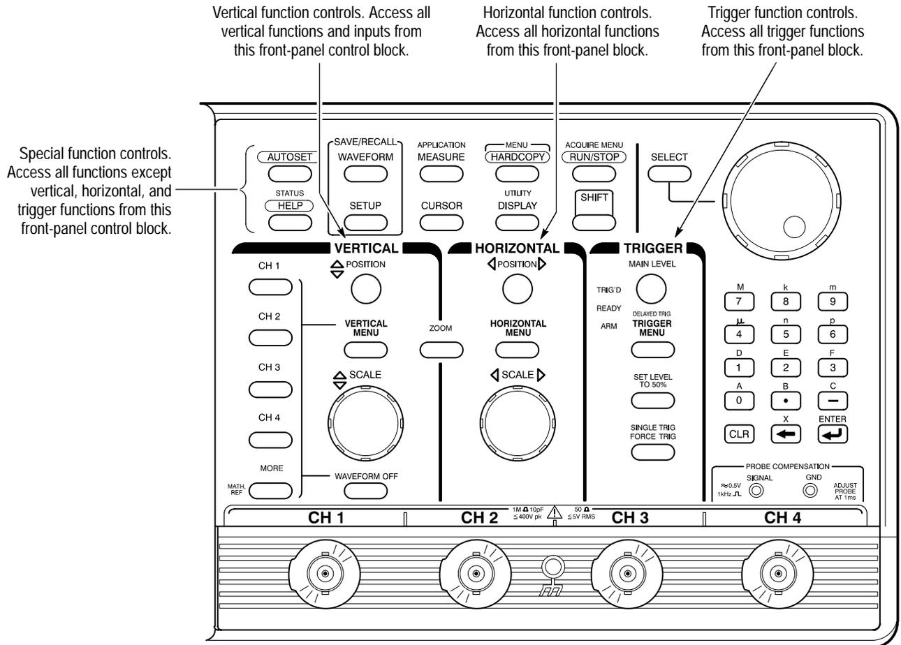
2. Select the waveform source(s). Position, scale, and set trigger level for waveform source(s) directly from the front panel. The steps that follow provide examples of possible control selections.
