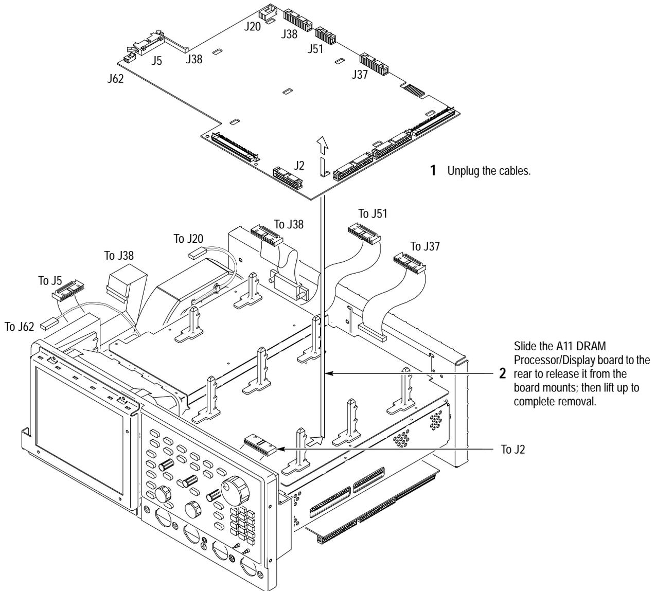
Figure 6–16: A11 Processor/Display Removal
