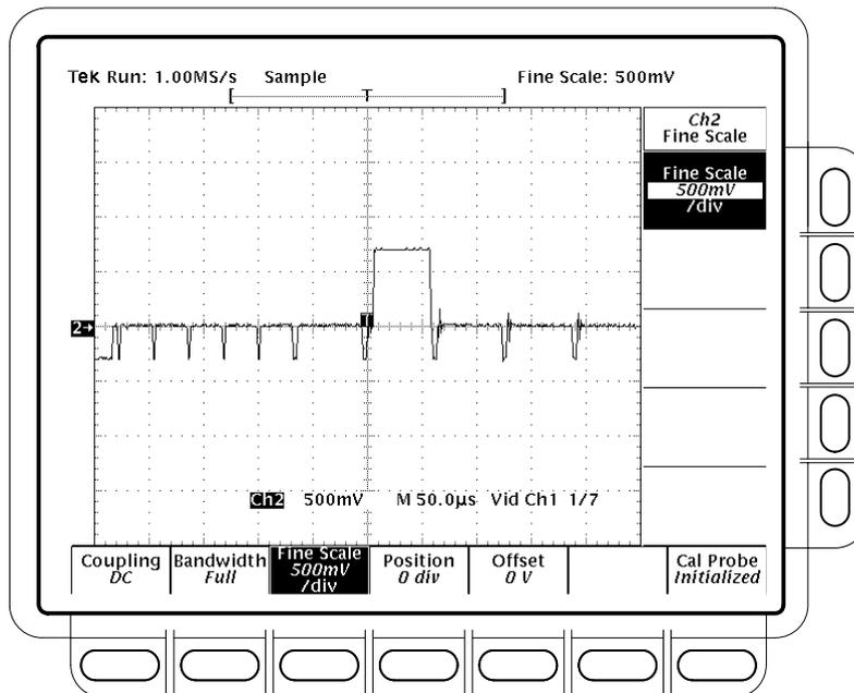
Figure 4–34: 60 Hz Rejection Test Result – TDS 684B Shown
