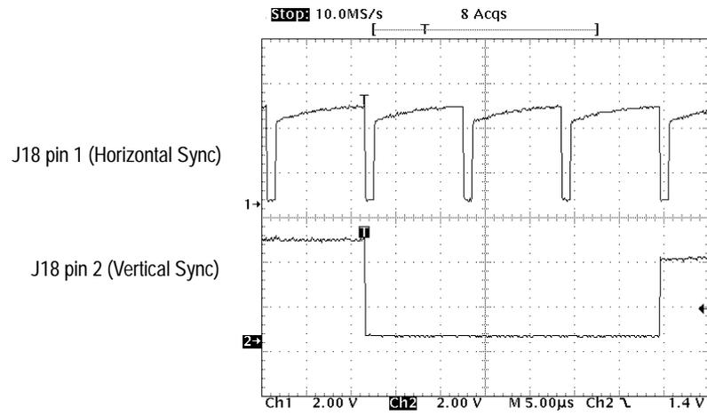
Figure 6-31: Horizontal and vertical sync signals – color display
