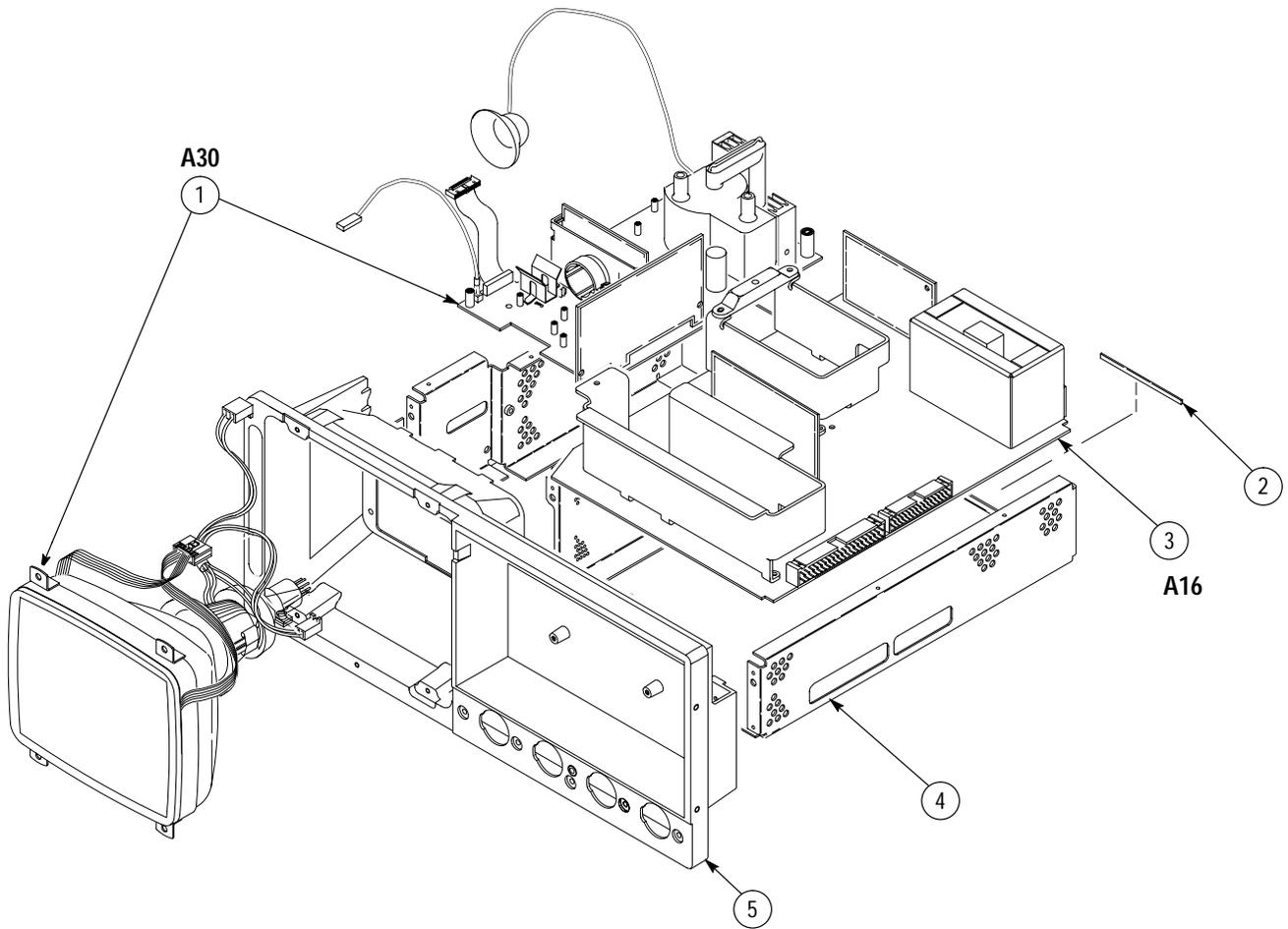
Figure 10-3: Inner-Chassis Modules
