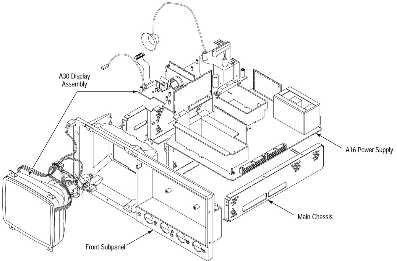
Figure 6-3: Inner-Chassis Modules
