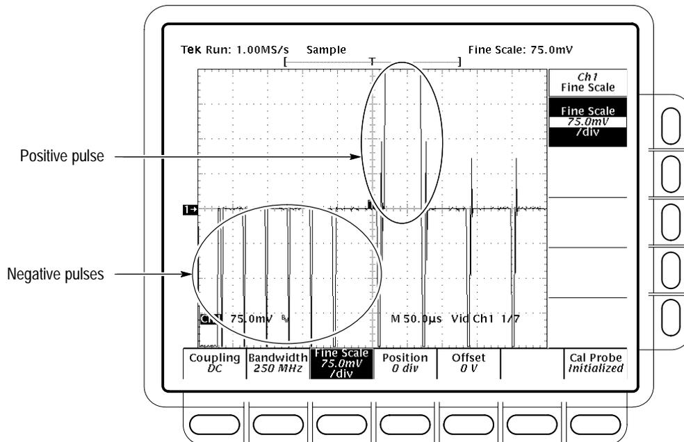
Figure 4-30: Triggered Signal Range Test – 75 mV
