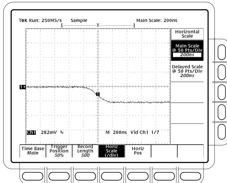
Figure 4-27: Jitter Test Displayed Waveform – TDS 684B Shown
