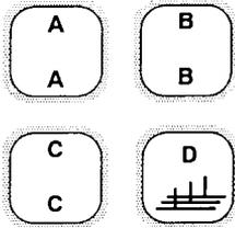
The 2710 can display an analog spectrum or up to four digitally sampled and stored spectra. A major advantage of display storage is that it results in a flicker-free display. The digital display storage registers are named A, B, C, and D. Their status is controlled by [A A], [B B], [C C], and [D ]; the red and green LED's to the left of each key indicate the status
