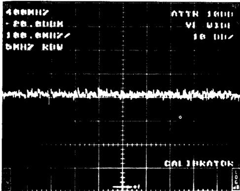
Average calibration signal plus noise subtracted from the current sweep
