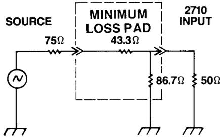
Figure 4-4. 75/50 ohm matching minimum loss pad.
