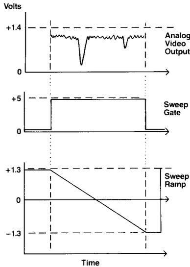
Figure 5-1. Sweep gate and ramp timing.
