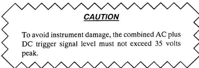
If the previous sweep is completed and item 2, EXTERNAL, is selected from the Sweep/Trigger Menu, an external trigger signal meeting the foregoing specification will start a new sweep each time it rises above a threshold established by the setting of the trigger LEVEL control. Typical external trigger signals might be a +5 volt logic level signifying that a transmitter has been keyed on, or that a receiver has detected a signal which rises above its squelch setting. For instance, to determine
