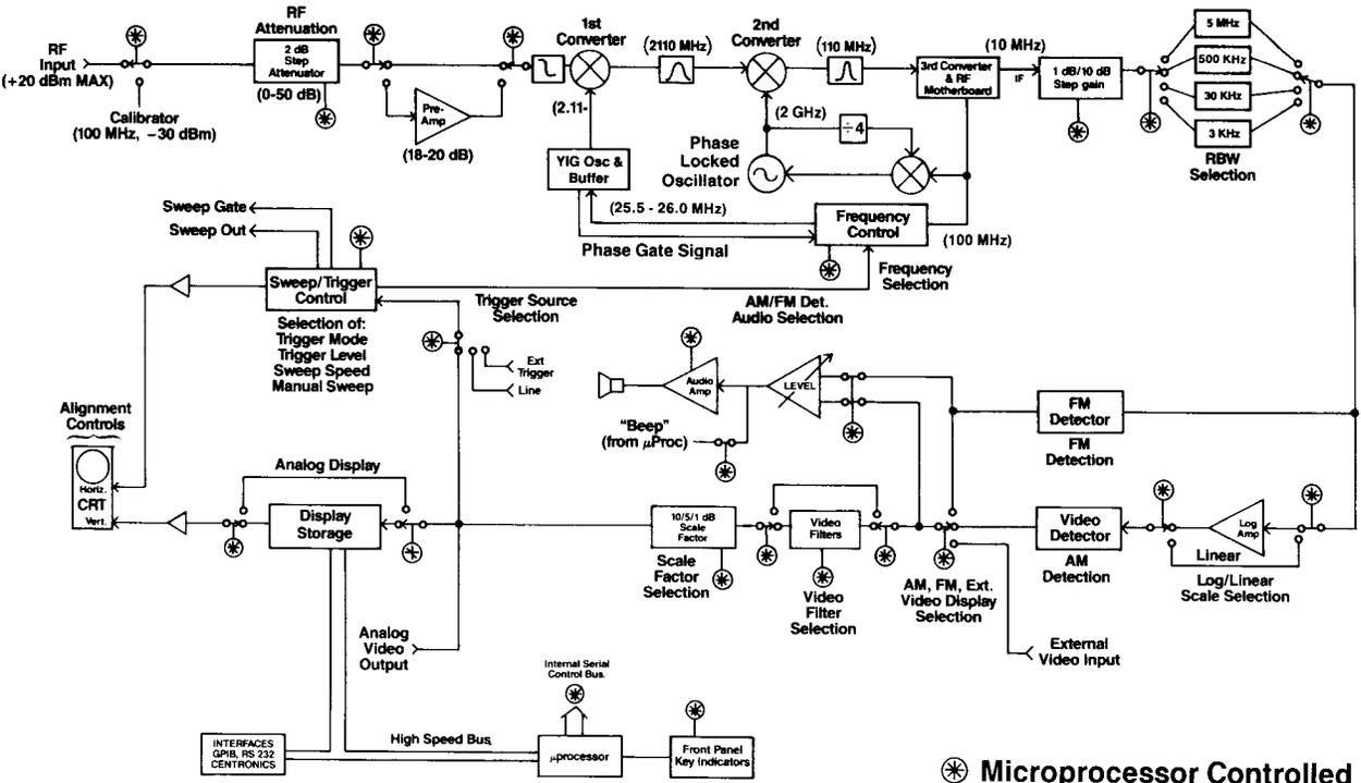
Figure 1-1. Spectrum analyzer block diagram (late model).
