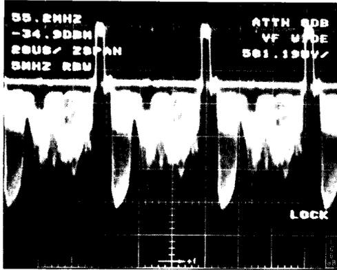
**Figure 4-17. Video signal using continuous horizontal line triggering.**
