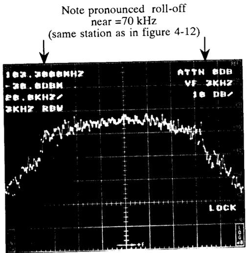
Figure 4-13. Frequency deviation by MAX HOLD technique.
