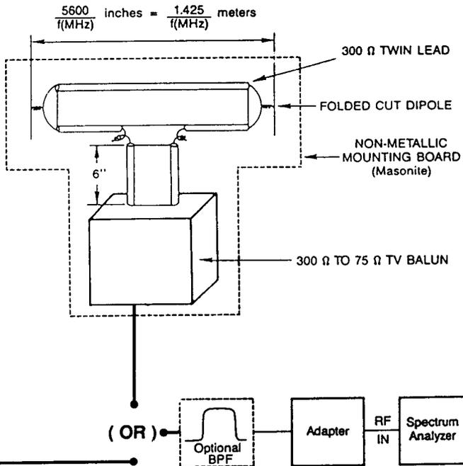
**Figure 4-5. Equipment setup for field strength measurements.**
