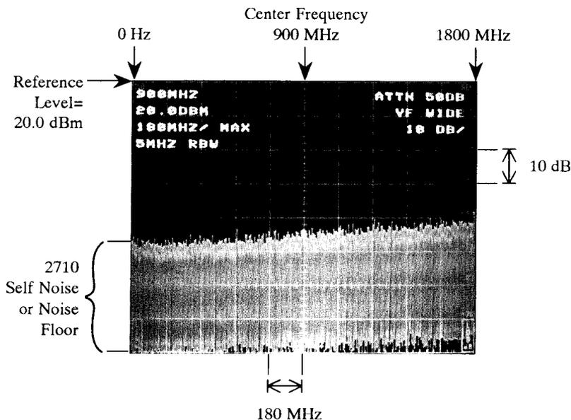
**Figure 2-1. 2710 display with factory power-up settings.**
