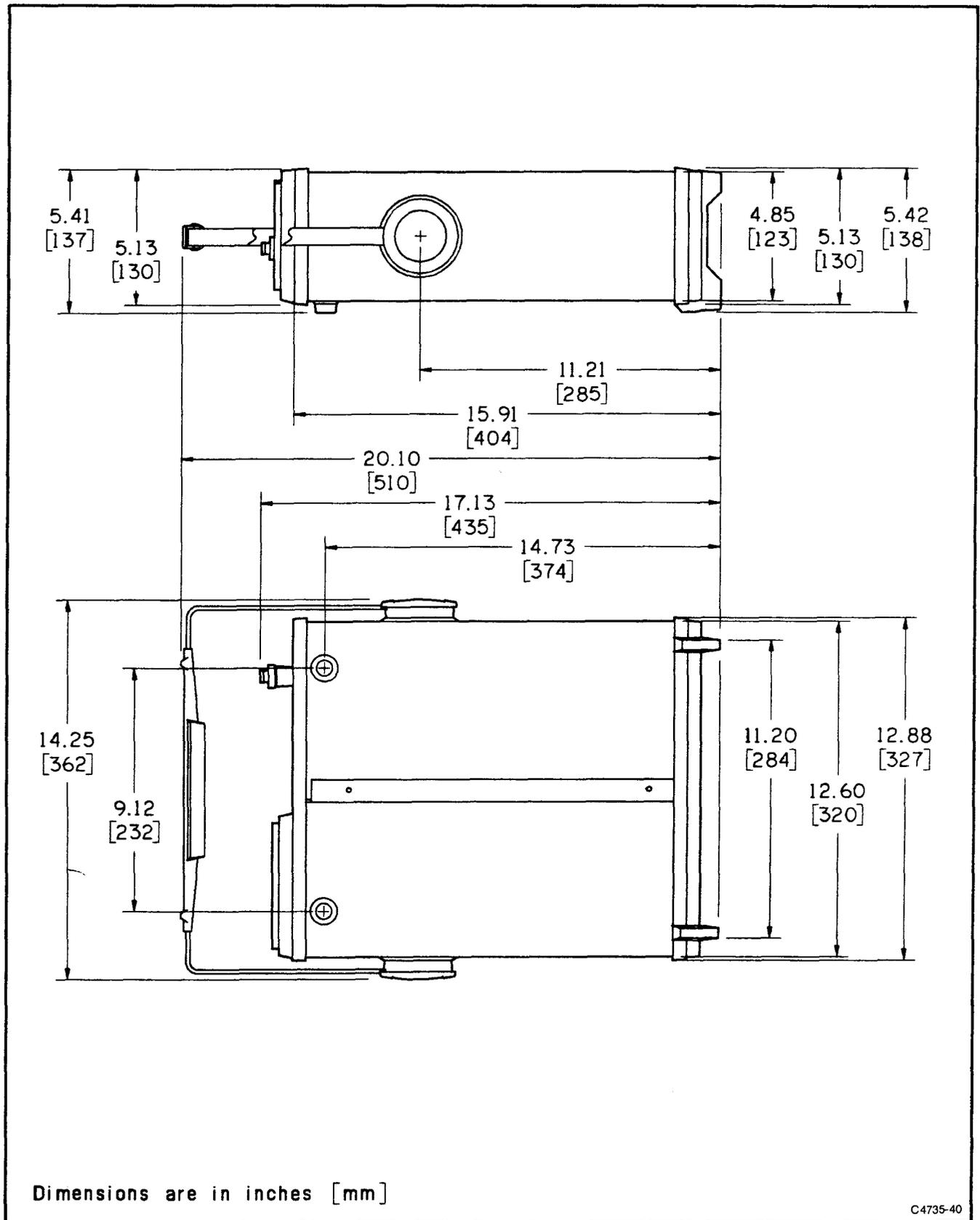
Figure 1-2. Physical dimensions of the 2213A Oscilloscope.
