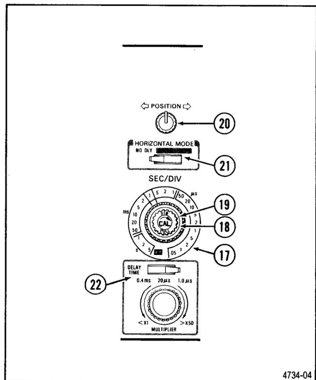
Figure 2-5. Horizontal controls.
