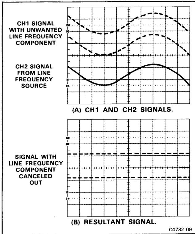
Figure 4-3. Common-mode rejection.
