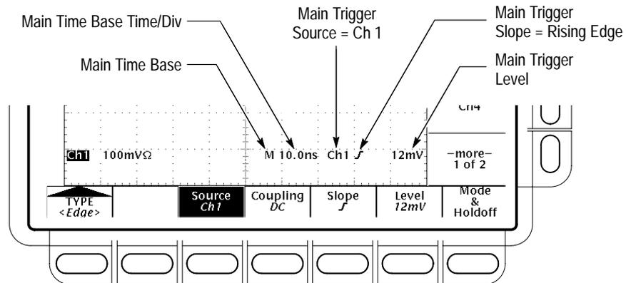
Figure 3-34: Example Trigger Readouts — Edge Trigger Selected
