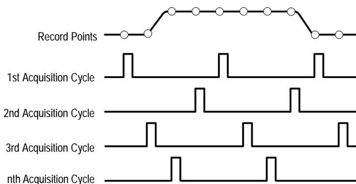
**Figure 3–12: Equivalent-Time Sampling**
