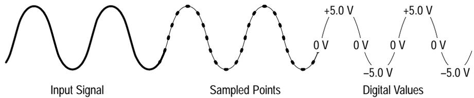
**Figure 3-9: Acquisition: Input Analog Signal, Sample, and Digitize**
