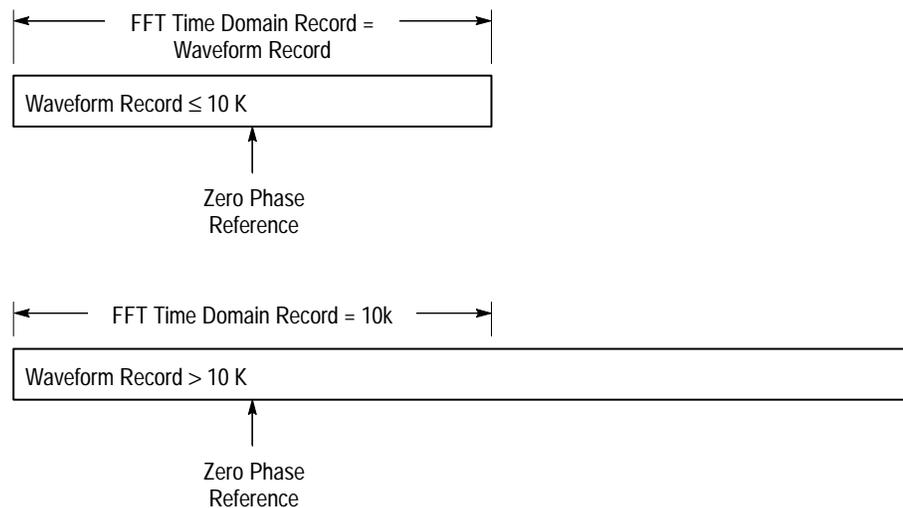
**Figure 3–90: Waveform Record vs. FFT Time Domain Record**
