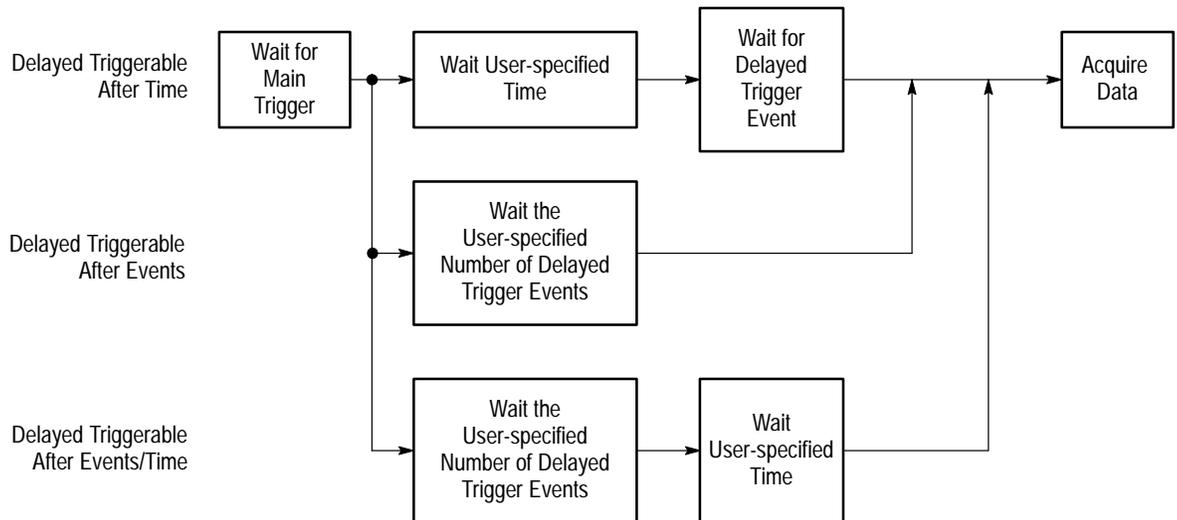
Figure 3–48: Delayed Triggerable
