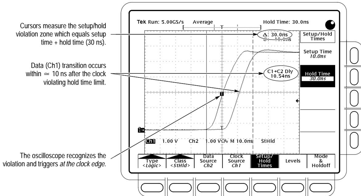
Figure 3-42: Triggering on a Setup/Hold Time Violation
