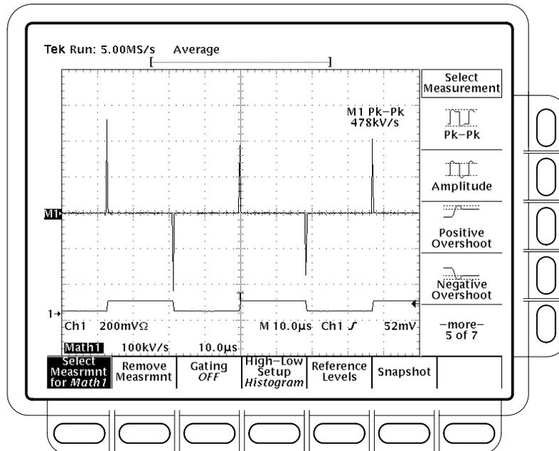
**Figure 3-96: Peak-Peak Amplitude Measurement of a Derivative Waveform**
