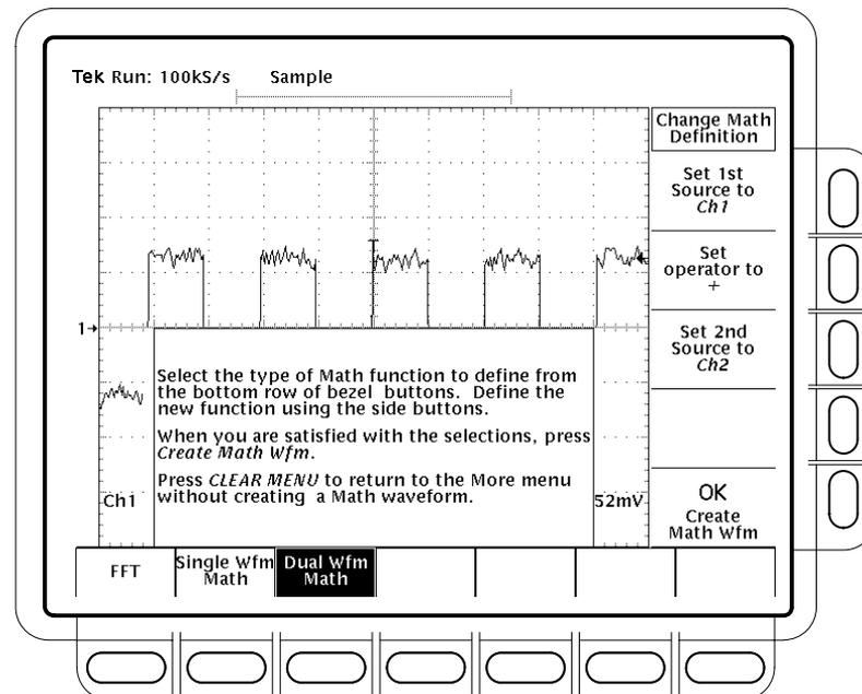
Figure 3–85: Dual Waveform Math Main and Side Menus
