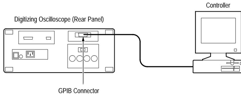
**Figure 3–77: Connecting the Oscilloscope to a Controller**
