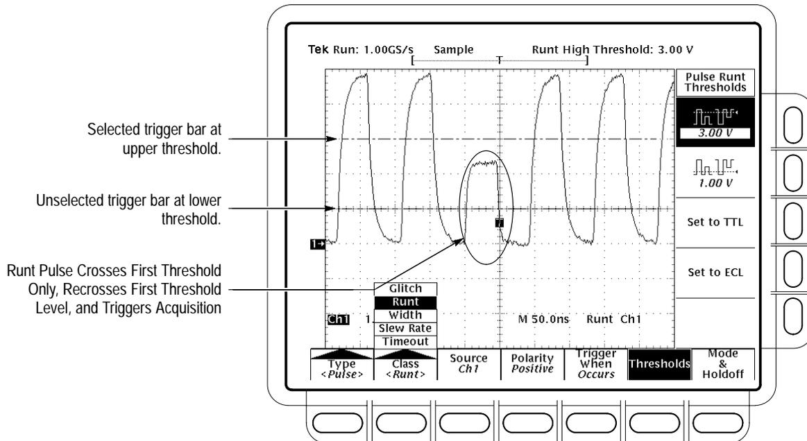
Figure 3–45: Main Trigger Menu — Runt Class
