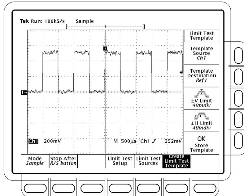
Figure 3-83: Acquire Menu — Create Limit Test Template
