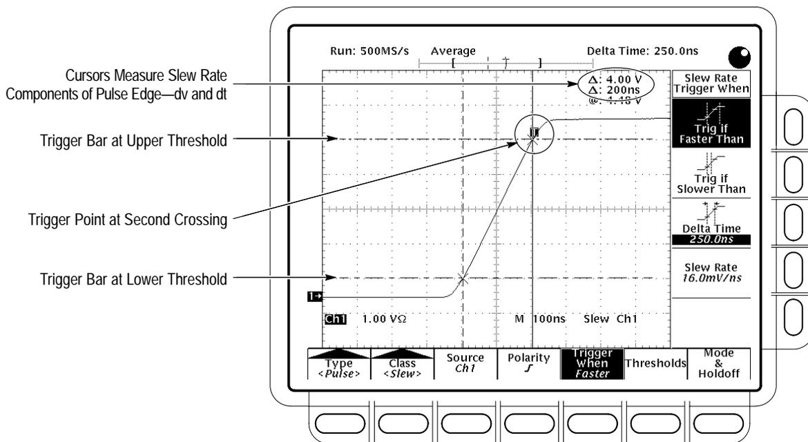
Figure 3-46: Main Trigger Menu — Slew Rate Class
