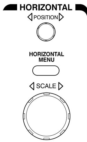
Figure 3–8: Horizontal Controls
