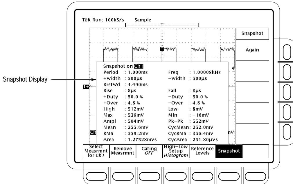
Figure 3-57: Snapshot Menu and Readout
