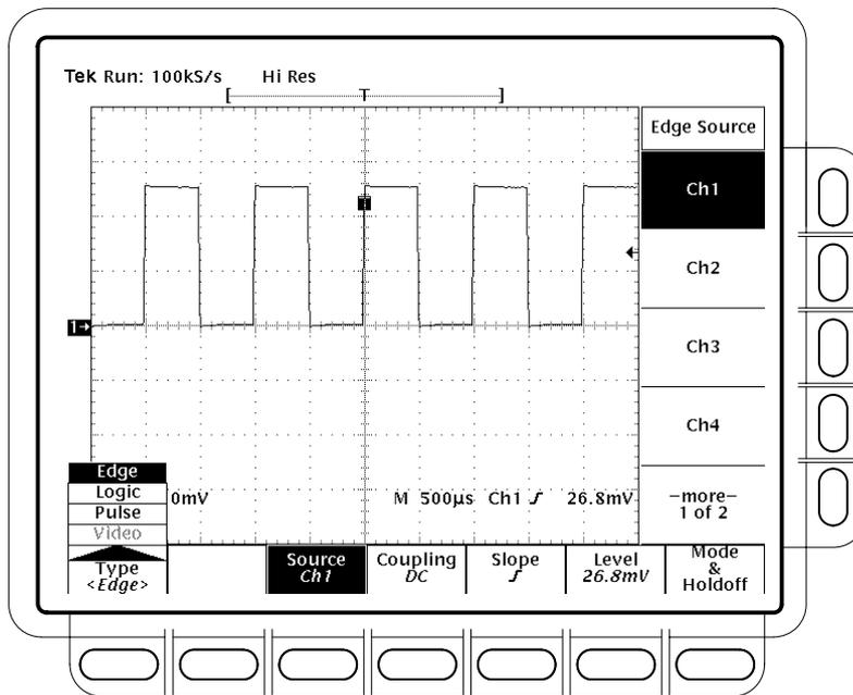
**Figure 3–37: Main Trigger Menu — Edge Type**
