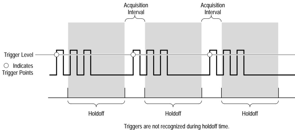
**Figure 3–31: Trigger Holdoff Time Ensures Valid Triggering**
