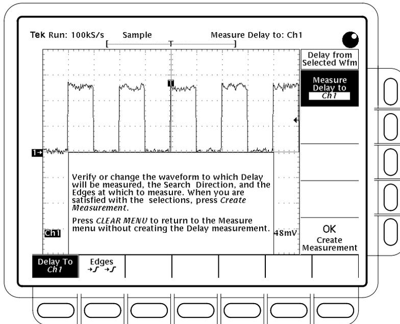
Figure 3–56: Measure Delay Menu — Delay To
