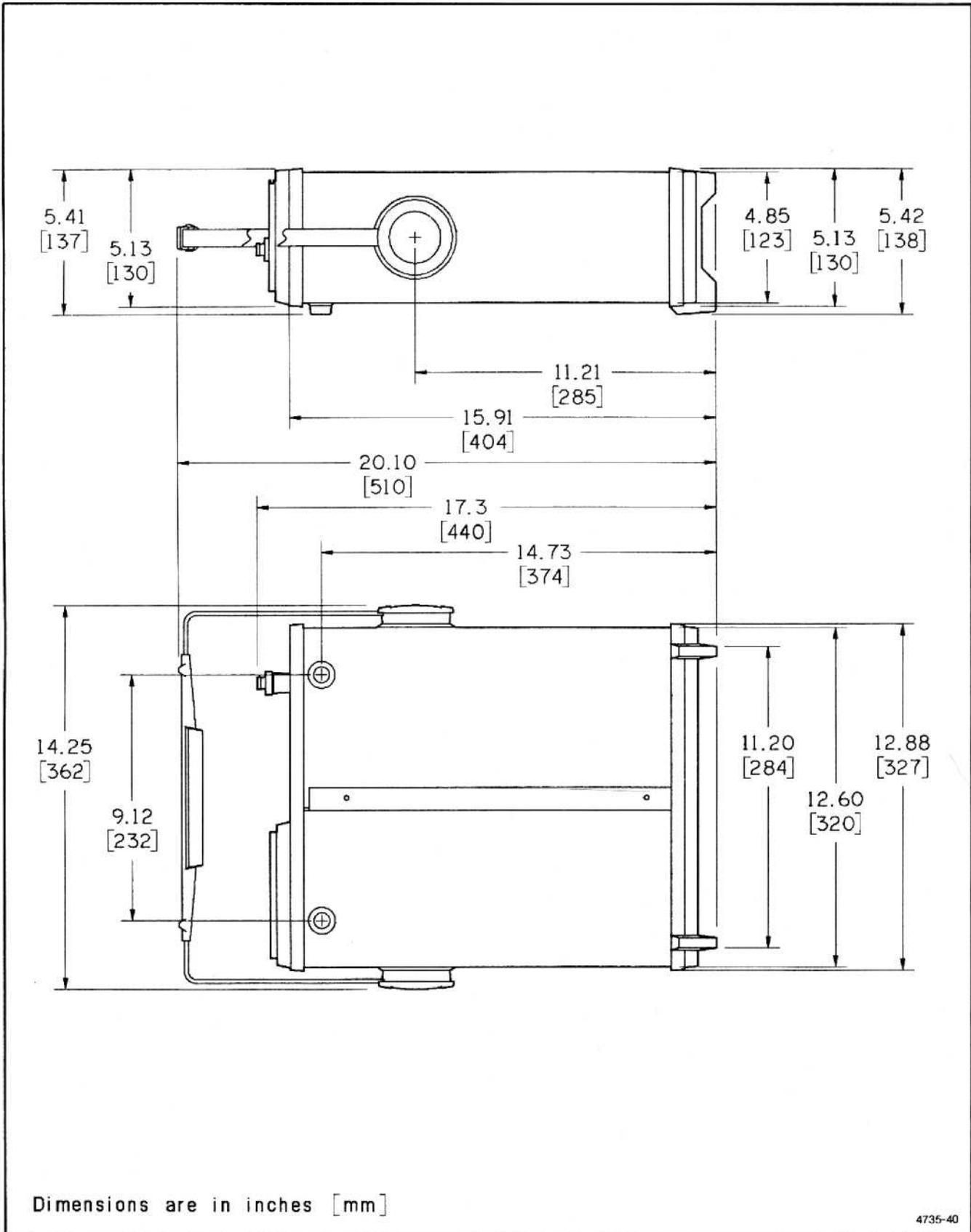
Figure 1-2. Physical dimensions of the 2235 Oscilloscope.
