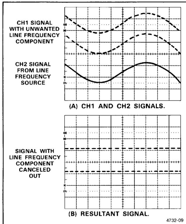
Figure 4-4. Common-mode rejection.
