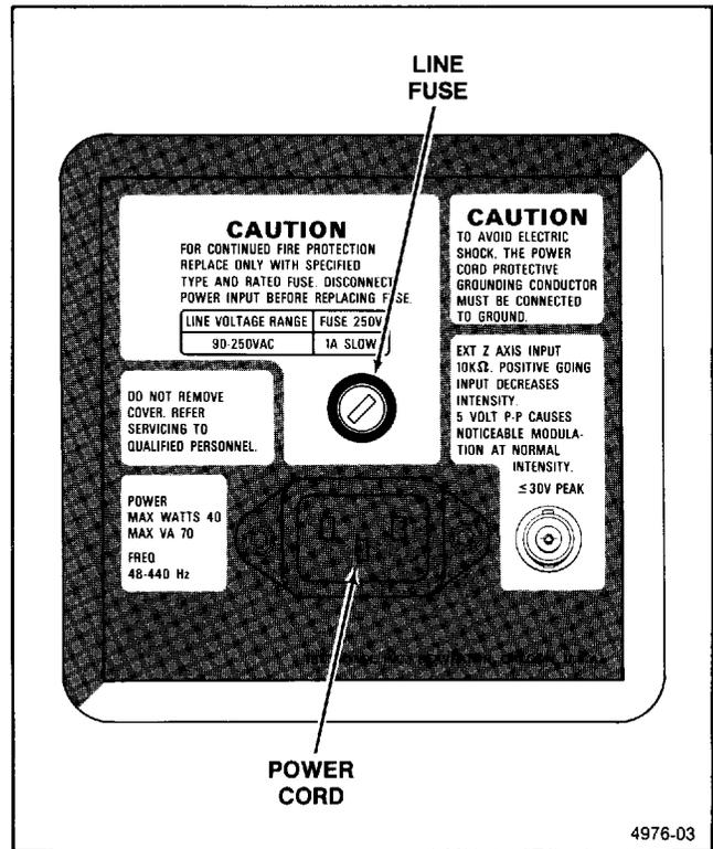
Figure 2-2. Fuse holder and power cord connector.
