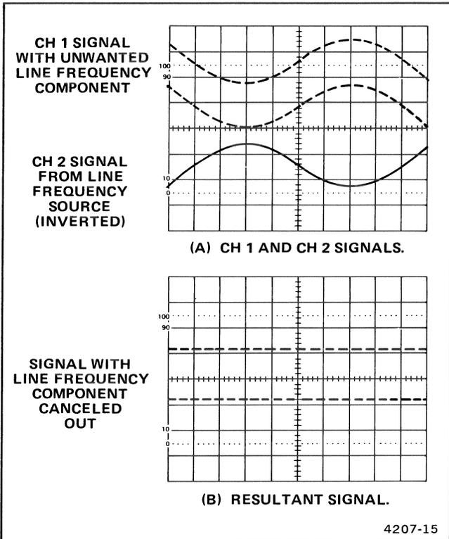
Figure 4-5. Common-mode rejection.
