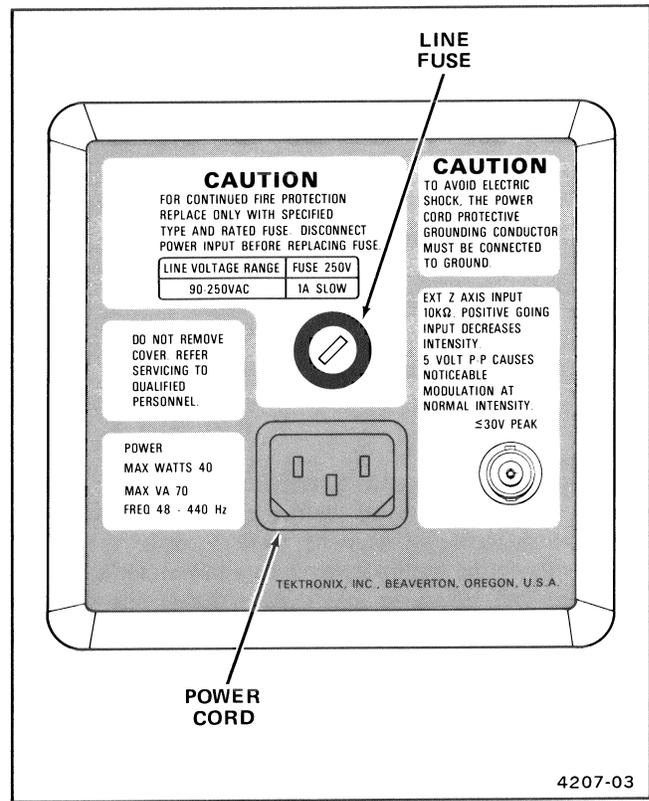
Figure 2-2. Fuse holder and power cord connector.
