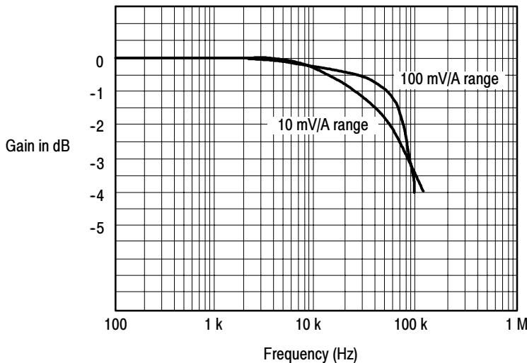
**Figure 6: Gain versus frequency at 1 A peak, typical**
