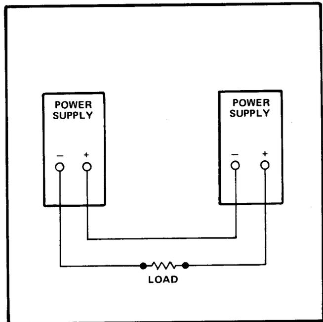
Fig. 1-5. Series-connected supplies.
