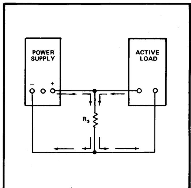
Fig. 1-4. Reverse current shunt ( $R_s$ ) with active load.
