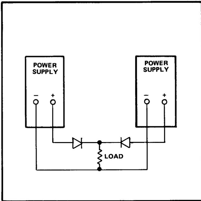
Fig. 1-6. Parallel-connected supplies.
