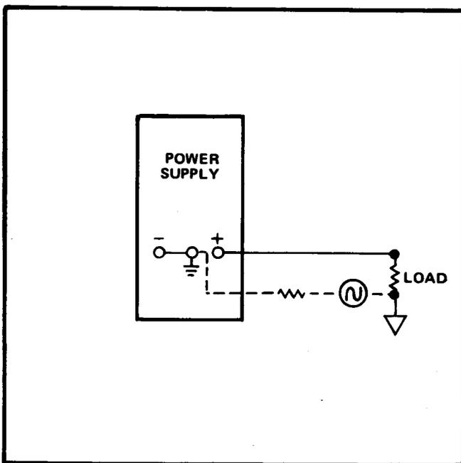
Fig. 1-3. Ground loop created by grounded remote load.
