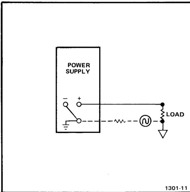
Fig. 2-10. Ground-loop current caused by remote grounded load.
