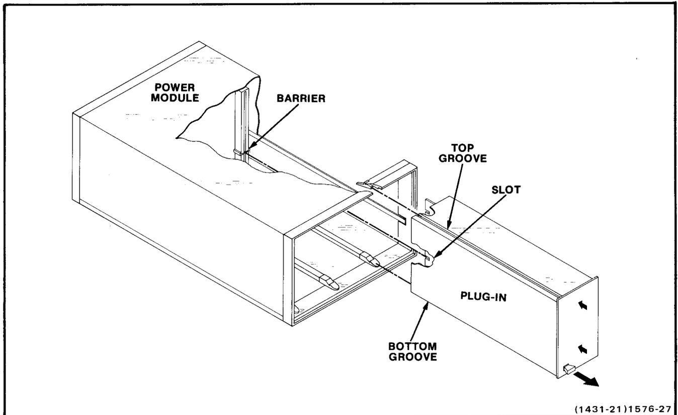
Fig. 2-1. PS 501 (-1, -2) Installation and removal.
