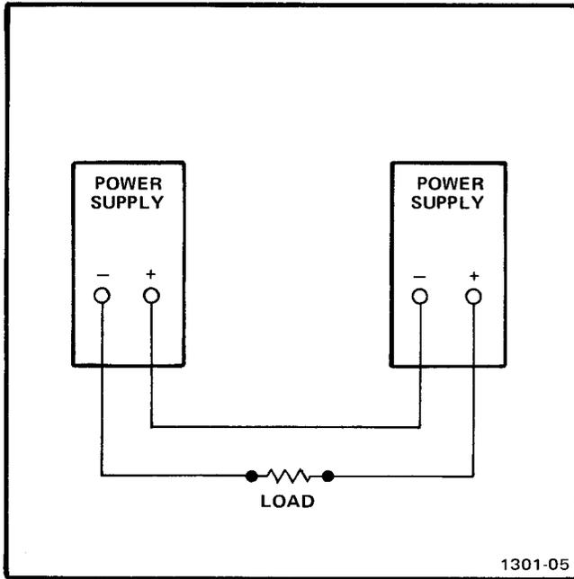
Fig. 2-4. Series-connected supplies.
