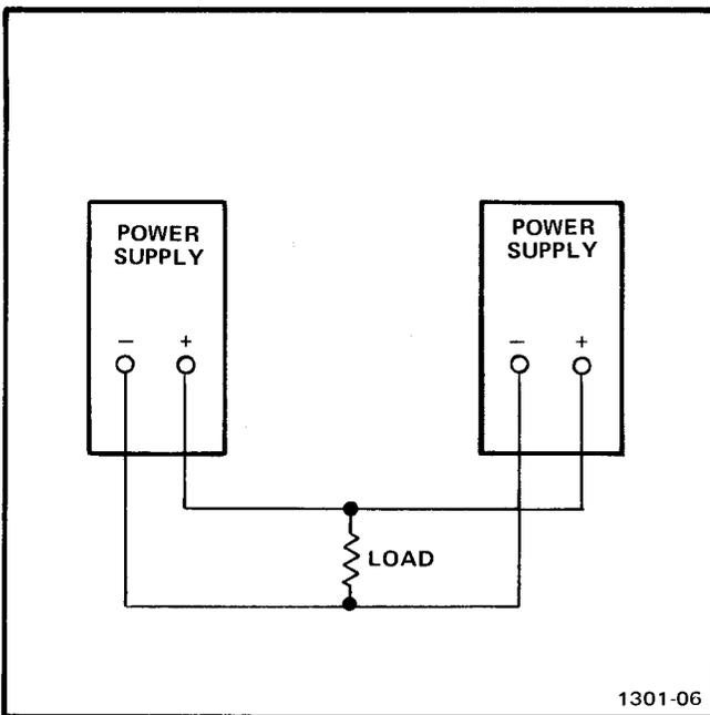
Fig. 2-5. Parallel-connected supplies.
