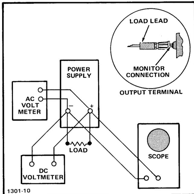
Fig. 2-9. Monitor connections.
