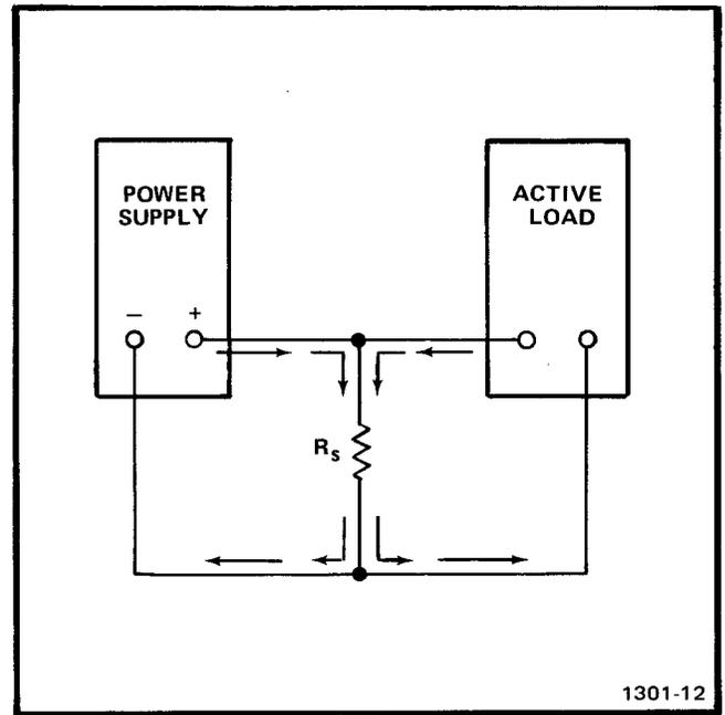
Fig. 2-11. Reverse-current shunt ( $R_s$ ) with active load.
