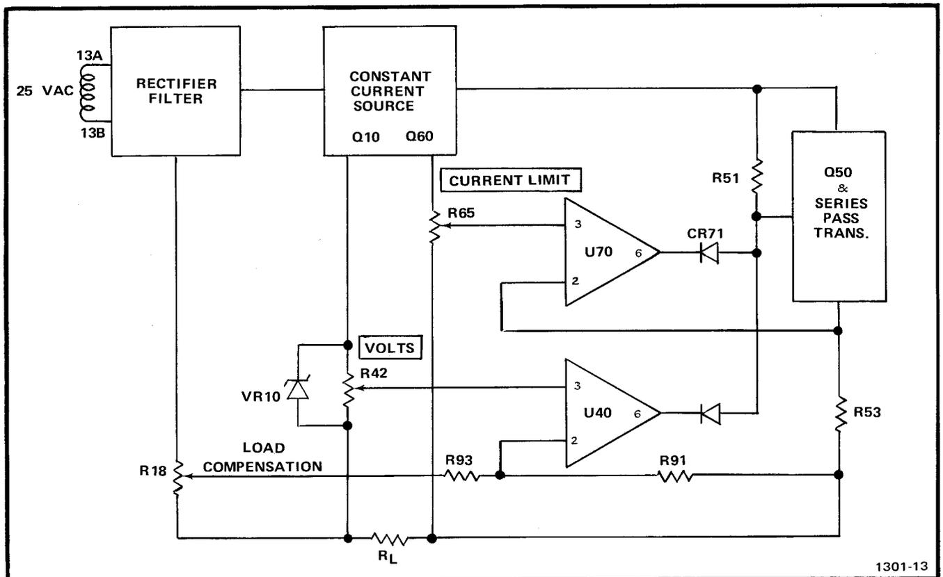
Fig. 3-1. Simplified diagram of PS 501 (-1, -2).
