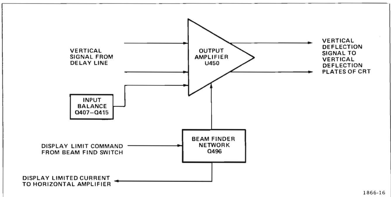
Figure 3-17. Vertical Amplifier circuit detailed block diagram.
