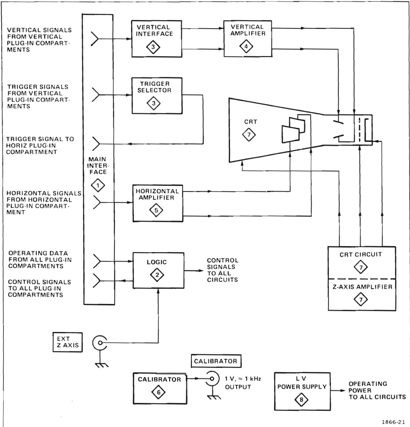
Figure 3-1. Basic block diagram of the Oscilloscope.
