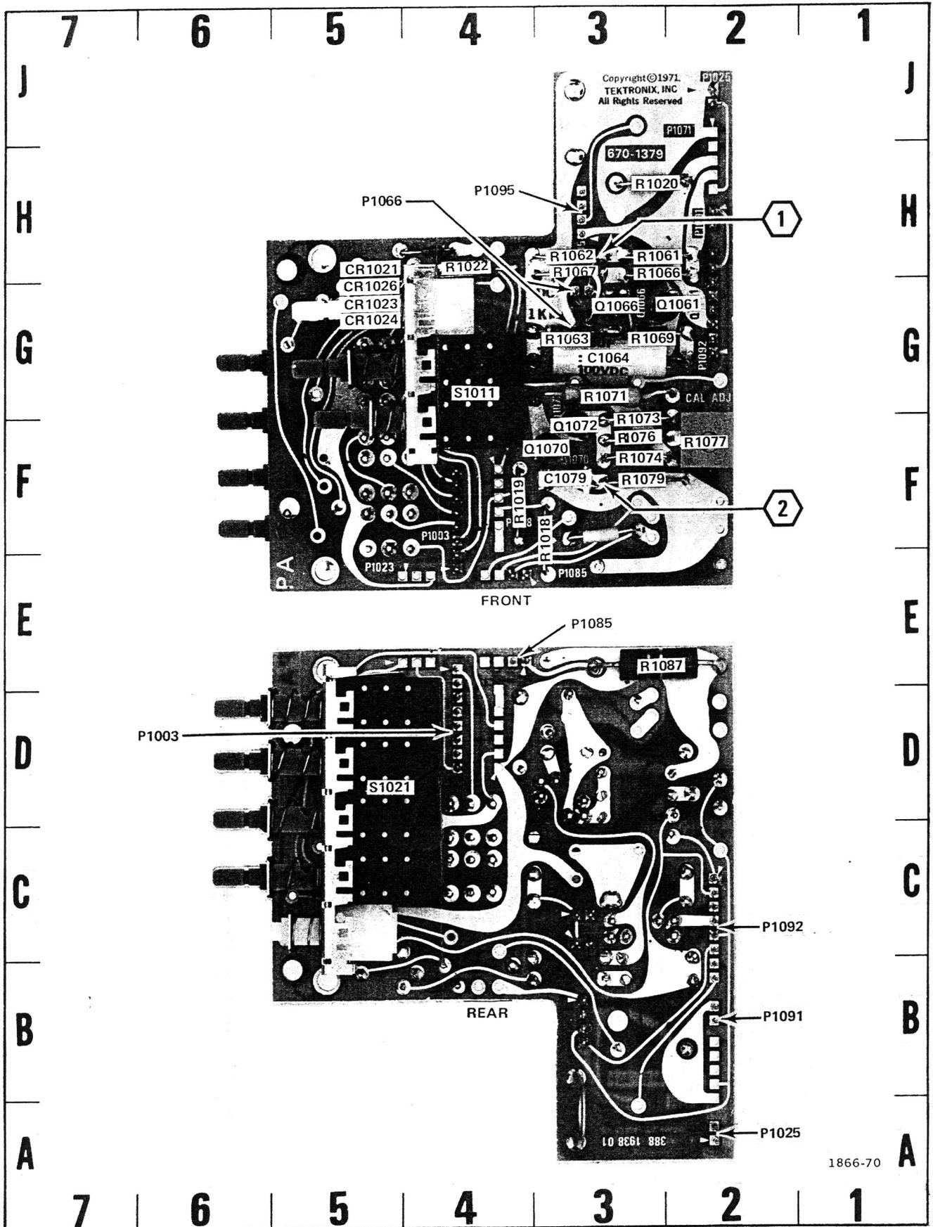
Figure 7-9. A7-Calibrator and Mode Switches circuit board assembly.
