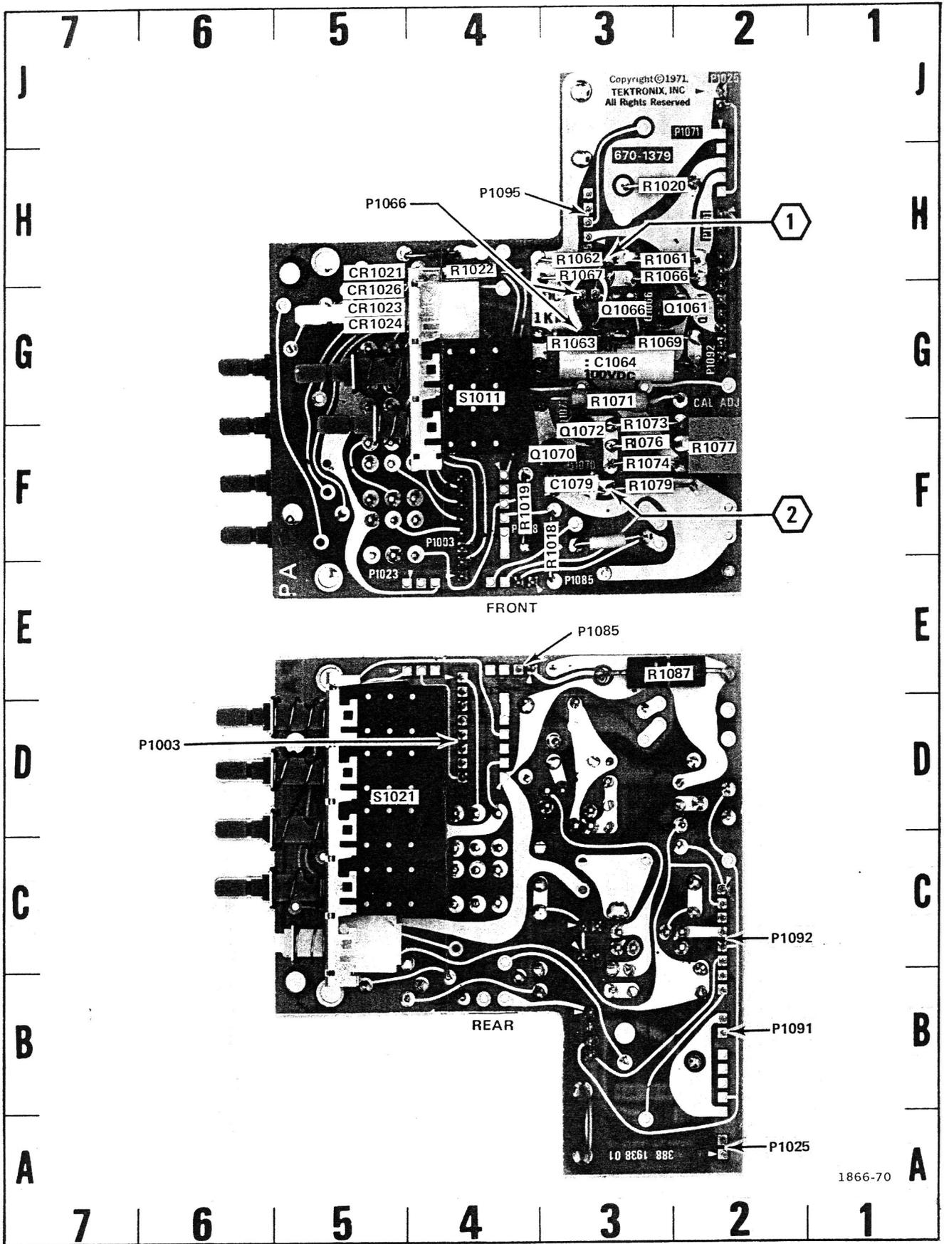
Figure 7-9. A7-Calibrator and Mode Switches circuit board assembly.
