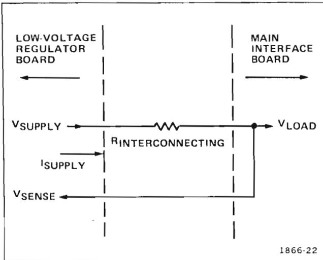
Figure 3-22. The voltage drop between the supply output and the load is overcome because feedback voltage is sensed at the load.
