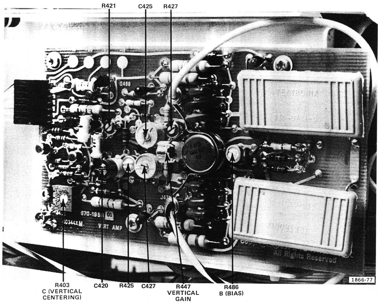
Figure 7-16. Locations of adjustments on Vertical Amplifier board.
