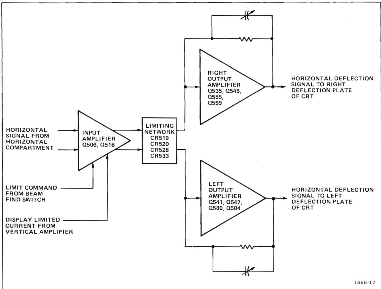
Figure 3-18. Horizontal Amplifier circuit detailed block diagram.
