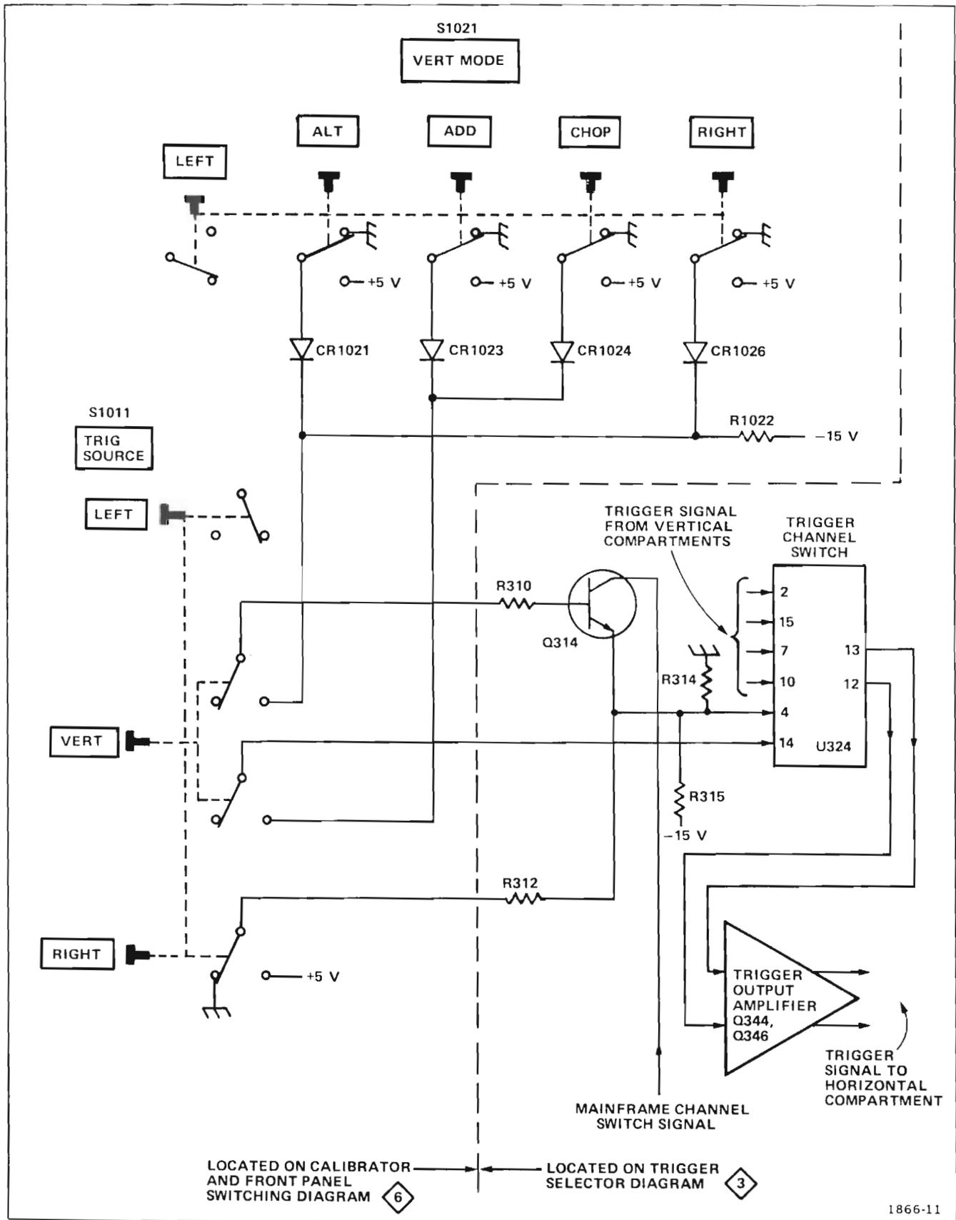
Figure 3-12. Trigger Selector and trigger-source selection circuitry.
