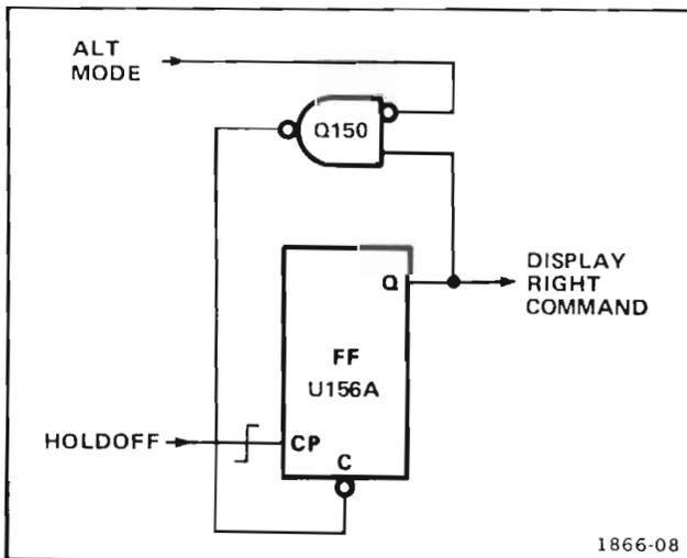
Figure 3-9. Vertical Binary stage logic diagram.
