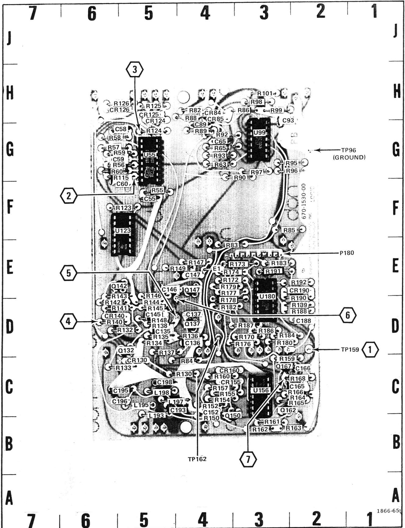
Figure 7-4. A2-Logic circuit board assembly.
