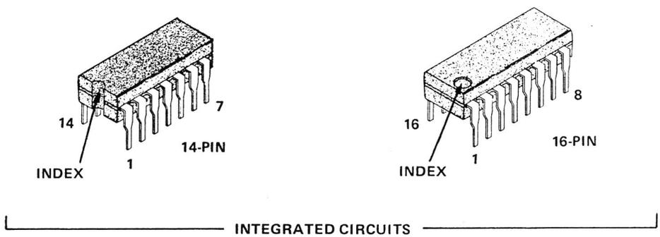
Figure 7-1. Semiconductor lead configurations.
