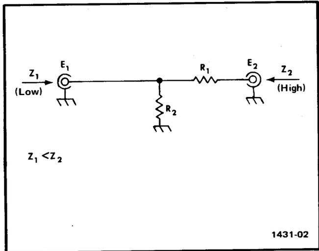
Fig. 1-4. Impedance-matching network that provides minimum attenuation.
