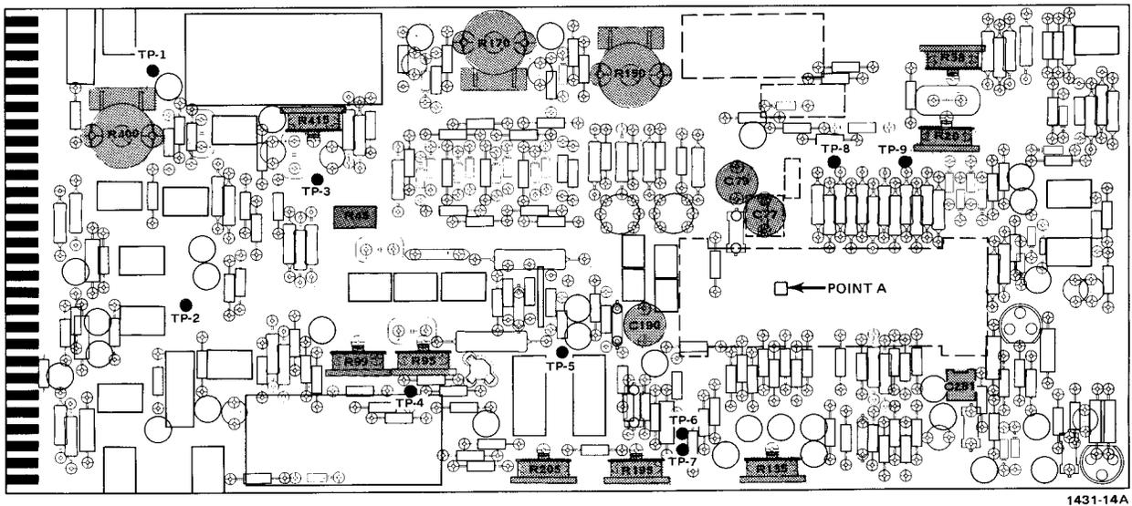
Fig. 3-2. Adjustment and test point locations, below SN B020000.
