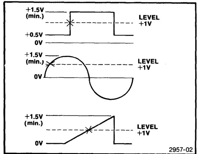
Fig. 2-7. Trigger Signal amplitude requirements and triggering points.
