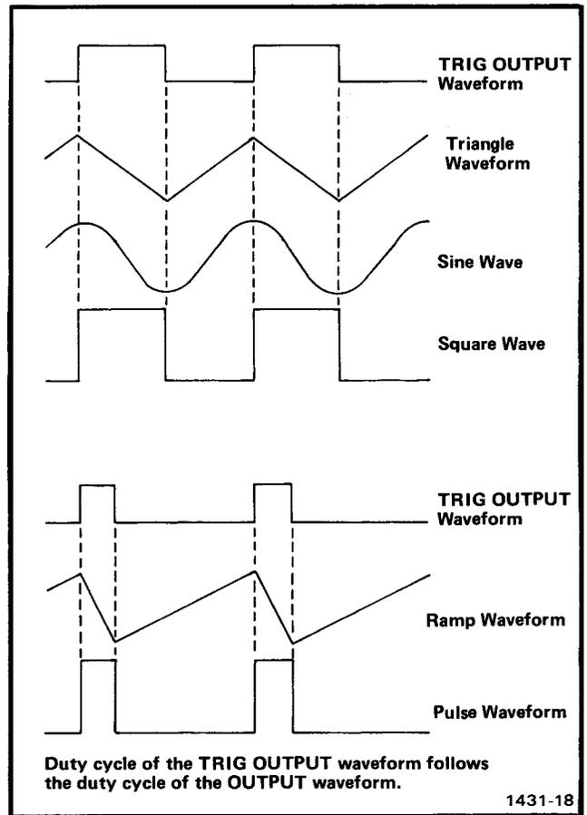
Fig. 1-8. Phase relationships between various waveforms from OUTPUT and TRIG OUTPUT connectors.
