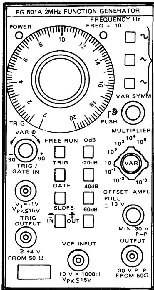
FIG.0-1. FG 501A 2MHz FUNCTION GENERATOR
