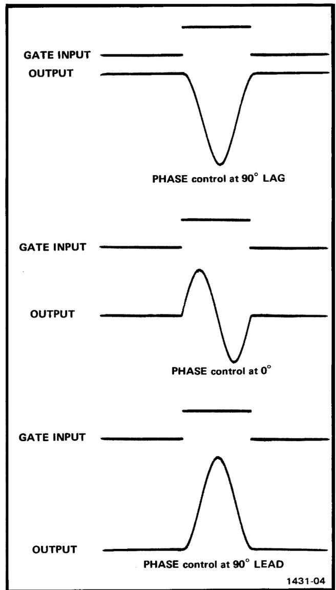
Fig. 1-6. Single cycle output with variable phase.
