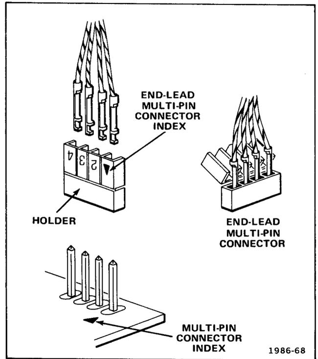
Fig. 5-2. Orientation and disassembly of multipin connectors.
