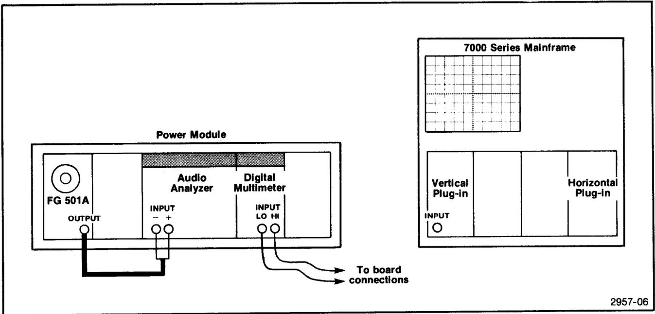
Fig. 4-2. Test setup for SINE DISTORTION adjustment.
