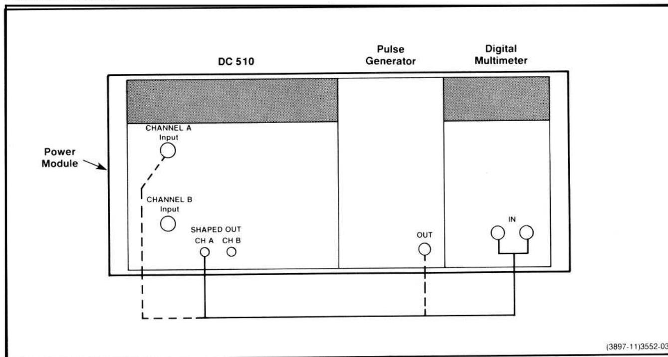
**Fig. 4-1. Performance Check setup for step 3.**
