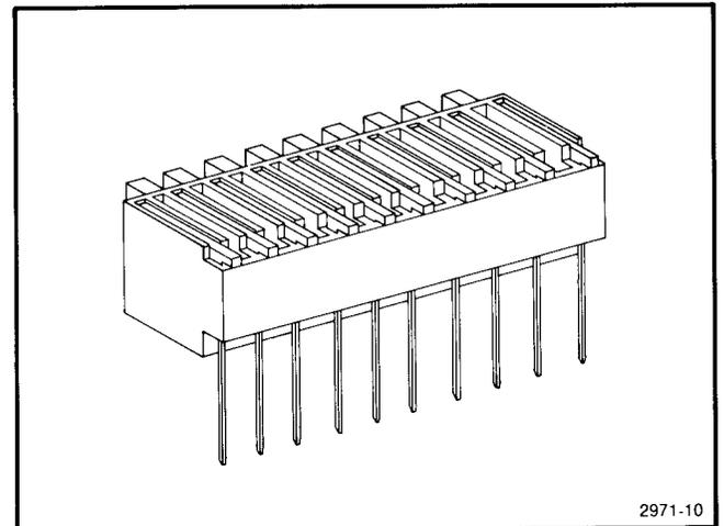
Fig. 5-4. Bottom entry circuit board pin socket.
