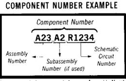
Chassis-mounted components have no Assembly Number prefix—see end of Replaceable Electrical Parts List.
