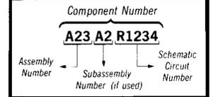
Chassis-mounted components have no Assembly Number prefix—see end of Replaceable Electrical Parts List.
