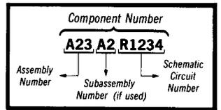
Chassis-mounted components have no Assembly Number prefix—see end of Replaceable Electrical Parts List.
