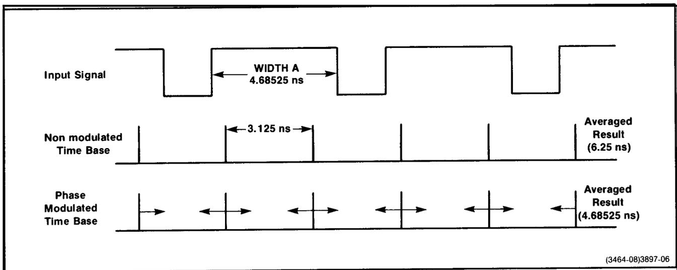
Fig. 2-6. Measurement example for synchronous input signals.
