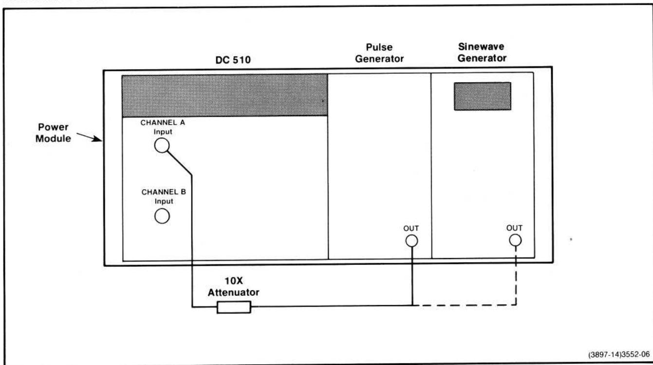
**Fig. 4-3. Performance Check setup for steps 5 and 14.**
