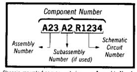
Chassis-mounted components have no Assembly Number prefix—see end of Replaceable Electrical Parts List.
