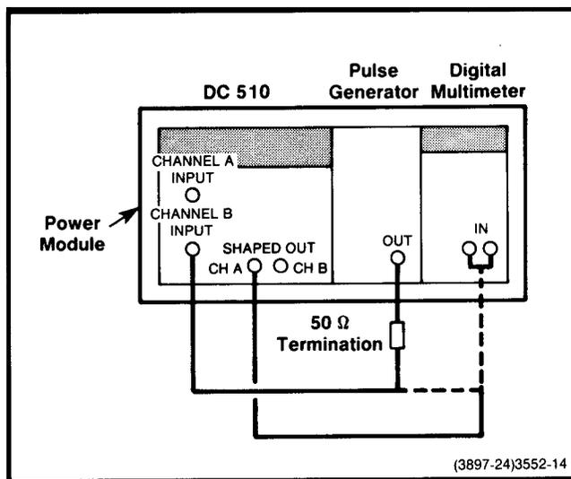
Fig. 8-3. Adjustment setup for steps 10 and 11.
