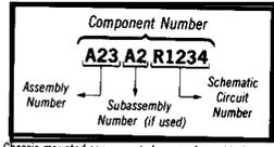
Chassis-mounted components have no Assembly Number prefix—see end of Replaceable Electrical Parts List.
