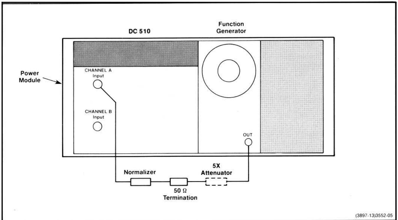
Fig. 4-4. Performance Check setup for step 6.
