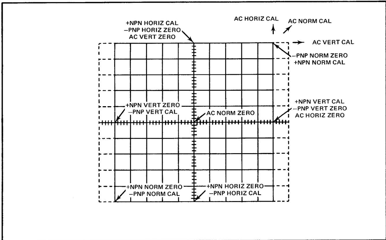
Fig. 2-20. Positions of spot on CRT graticule when ZERO or CAL buttons are pressed, for various positions of the POLARITY switch and the DISPLAY OFFSET Selection switch, assuming the position controls are centered.
