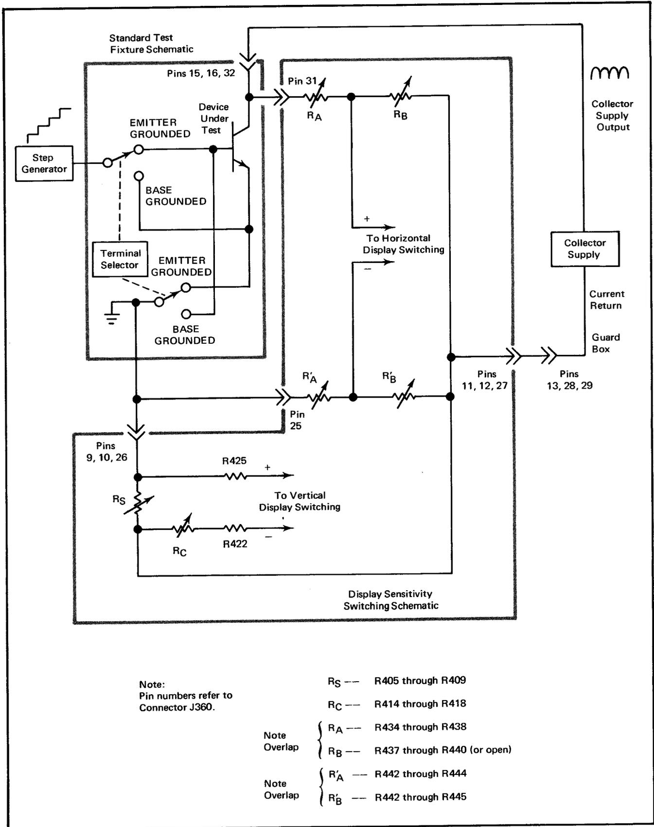
Fig. 3-8. Simplified schematic of Display Sensitivity Switching and Standard Test Fixture schematics for measurement of collector current ( $I_C$ ) and collector-emitter voltage ( $V_{CE}$ ) or collector-base voltage ( $V_{CB}$ ).
