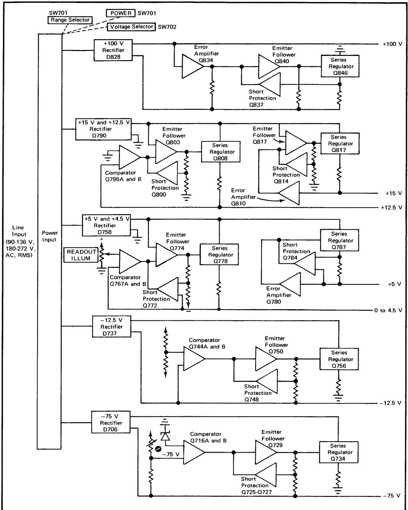
Fig. 3-14. Block diagram of L. V. Power Supply.
