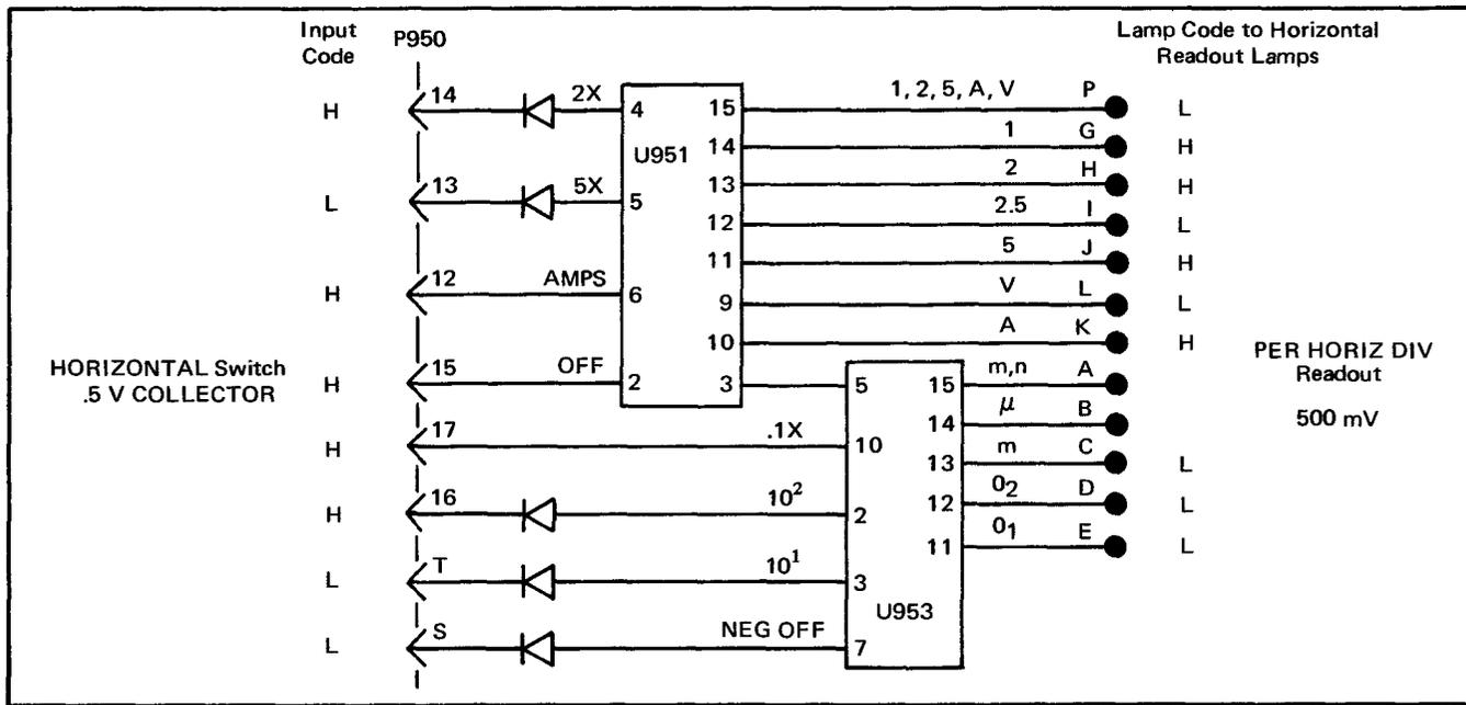
Fig. 3-13. Example of operation of Horizontal Readout decoders.
