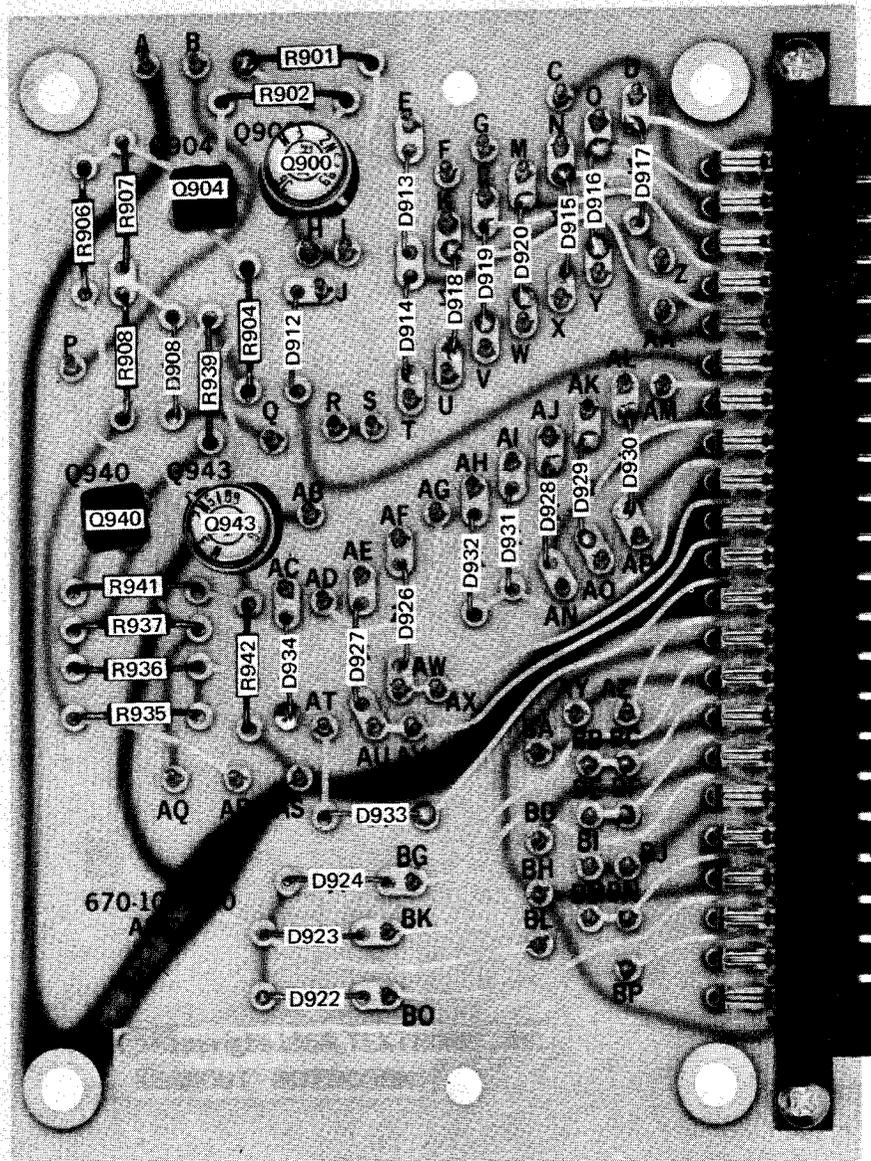
Fig. 4-18. Component locations on Readout Interconn circuit board.
