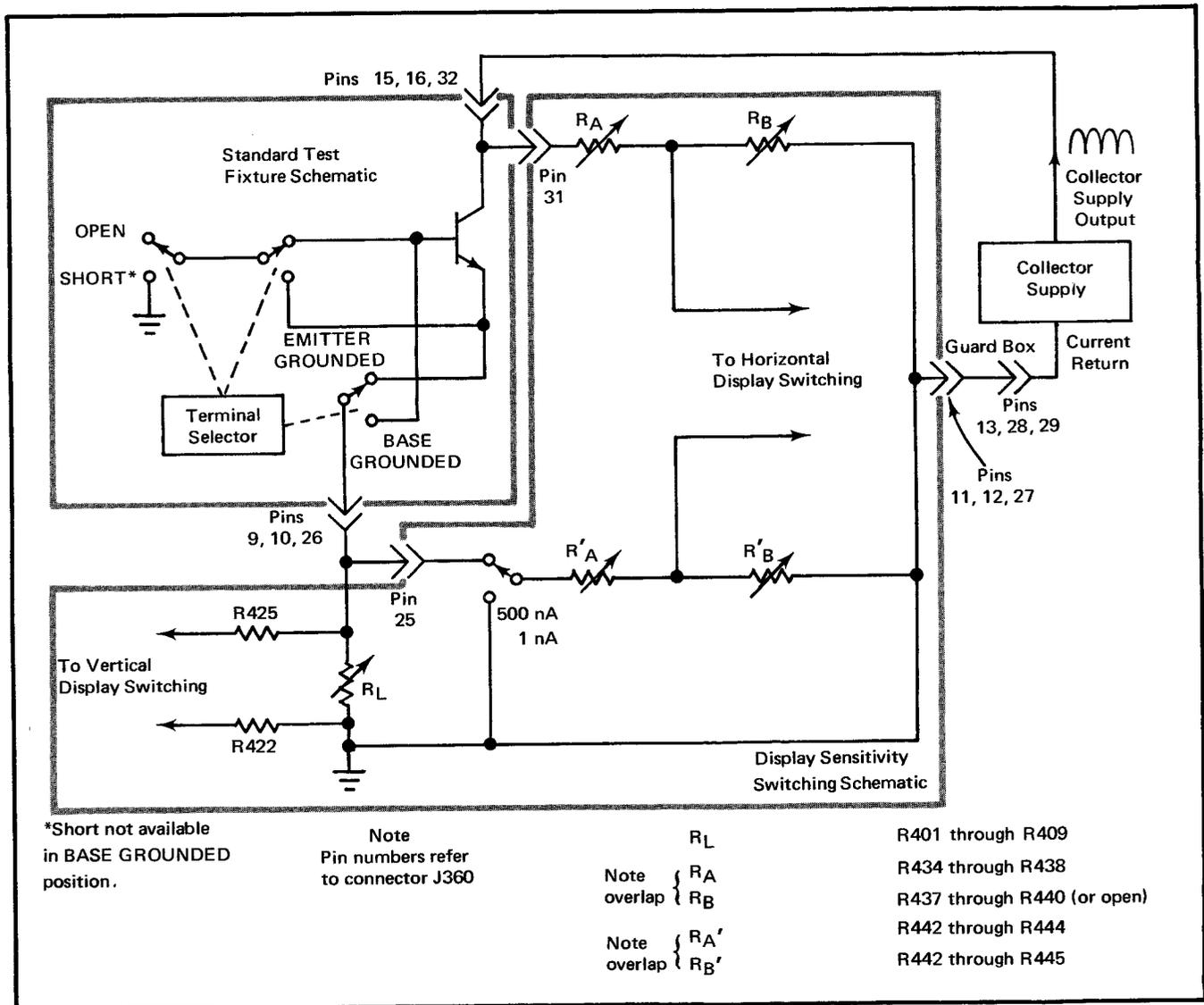
Fig. 3-10. Simplified schematic of Display Sensitivity switching and Standard Test Fixture schematics for measurement of emitter current ( $I_E$ ), collector-base current ( $I_{CB0}$ ), collector-emitter voltage ( $V_{CE}$ ) or collector-base voltage ( $V_{CB}$ ).
