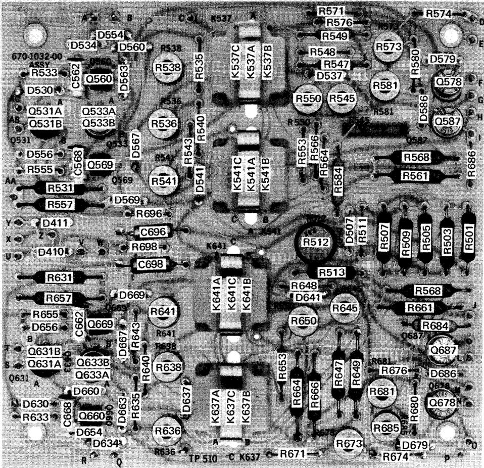
Fig. 4-16. Component locations on Display Amp circuit board.
