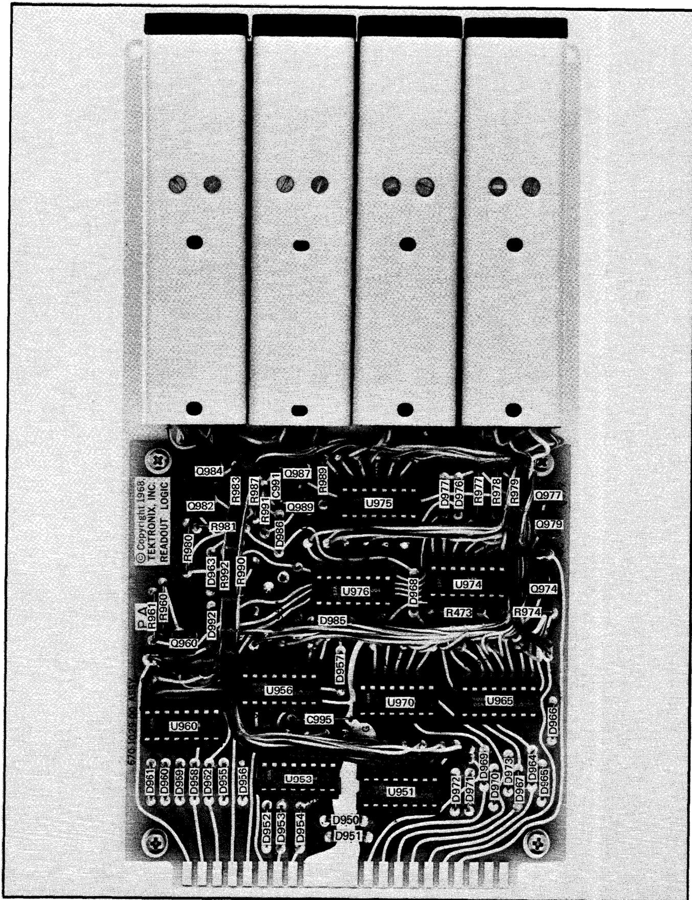
Fig. 4-20. Component locations on Readout Logic circuit board.
