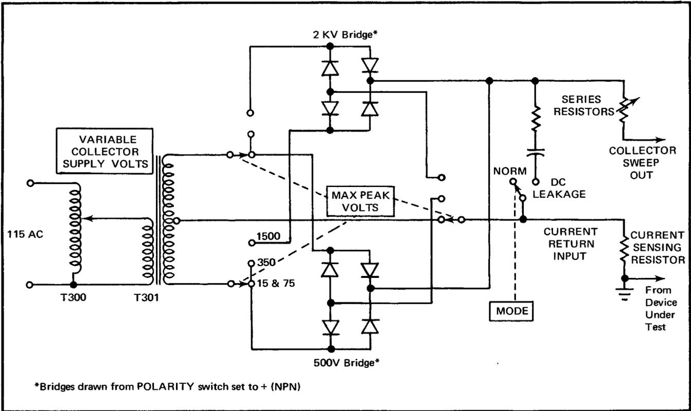
Fig. 3-1. Simplified schematic of collector supply circuit.
