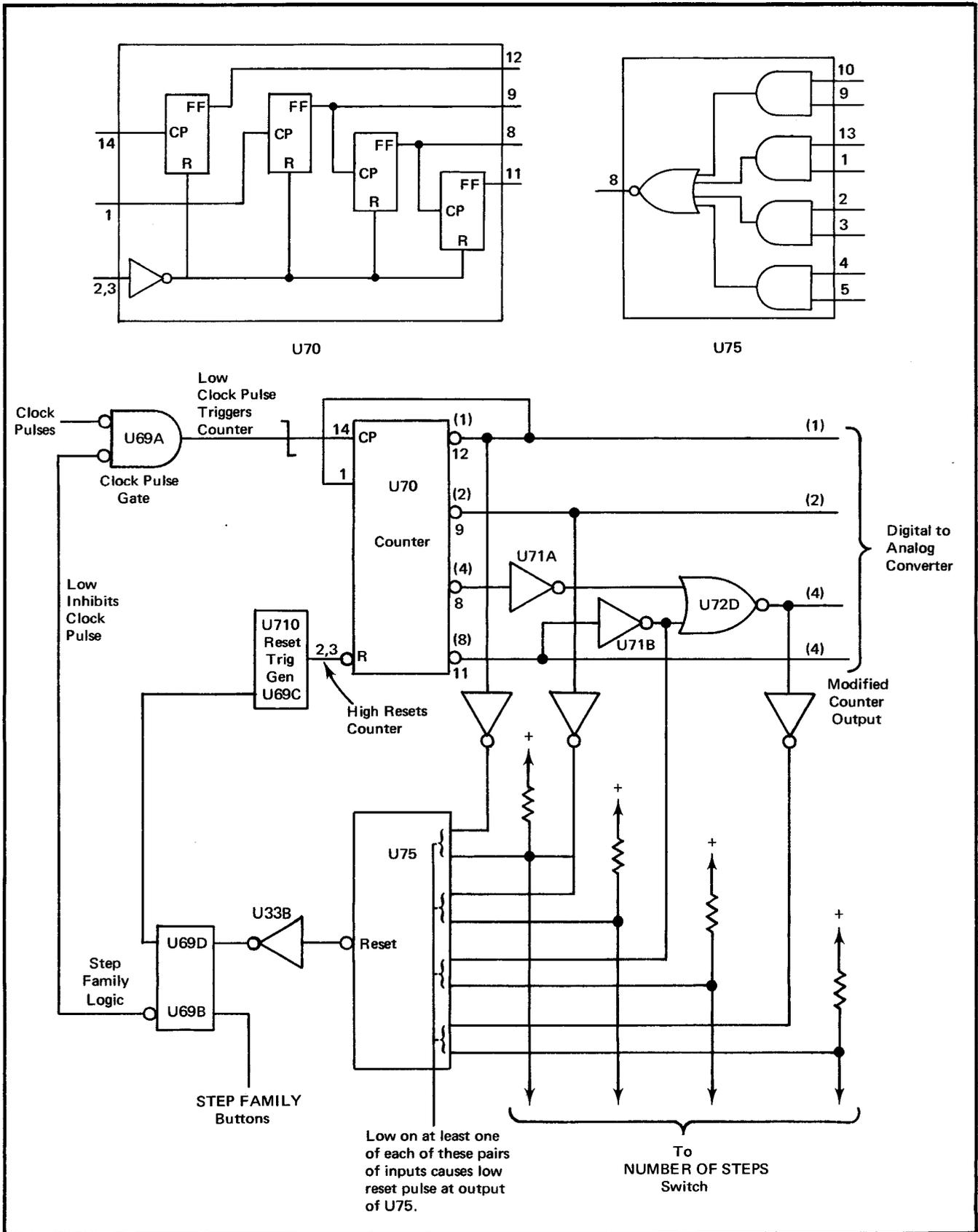
Fig. 3-5. Block diagram of counter and reset logic.
