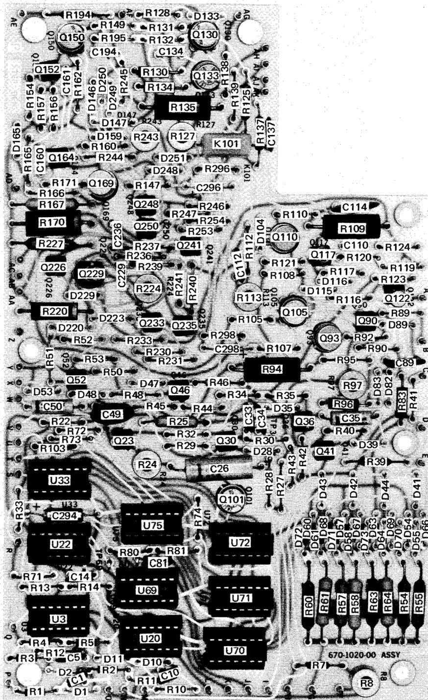
Fig. 4-6. Component locations on Step Gen circuit board.
