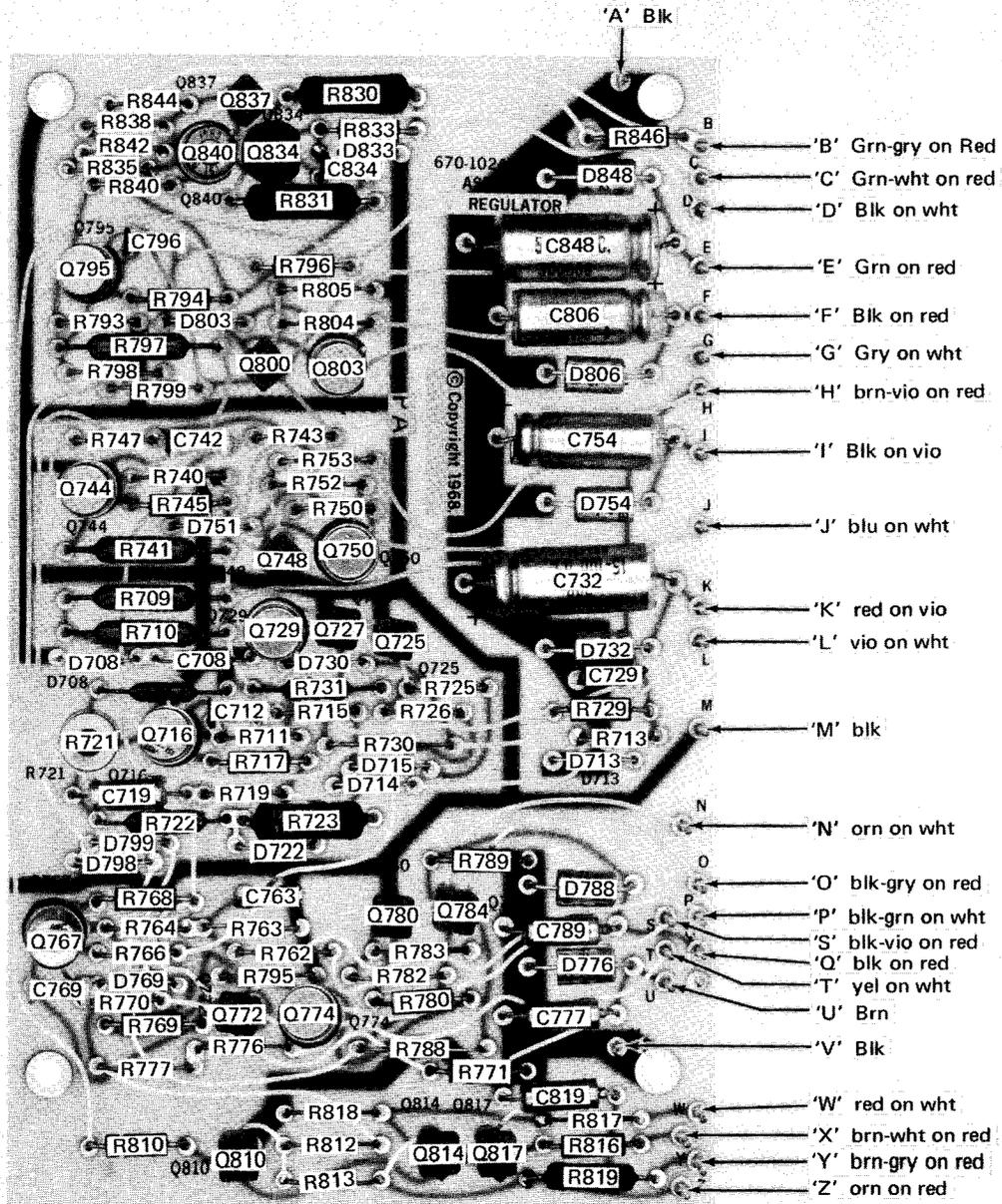
Fig. 4-24. Component locations and wiring color codes on L. V. Regulator circuit board.
