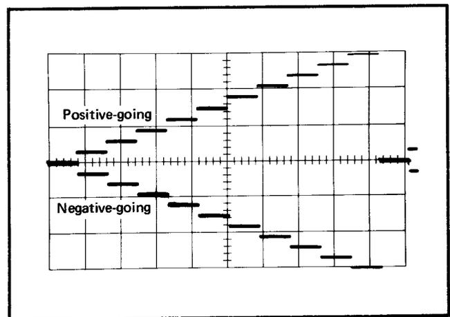
Fig. 2-24. Step Generator output in both polarities
