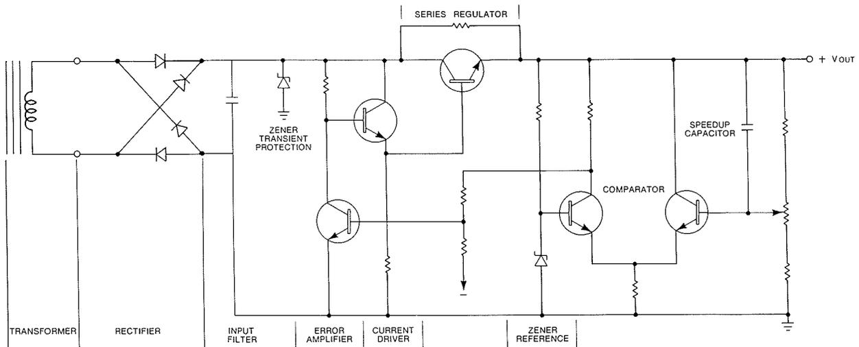
Fig 2. Simplified schematic of solid-state power supply.
