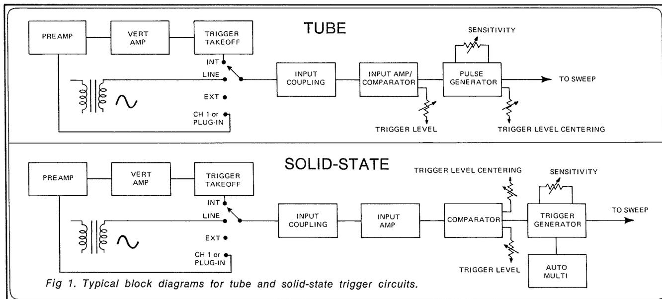
Fig 1. Typical block diagrams for tube and solid-state trigger circuits.
