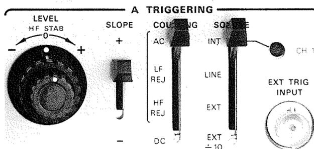
Typical Oscilloscope Triggering Controls
