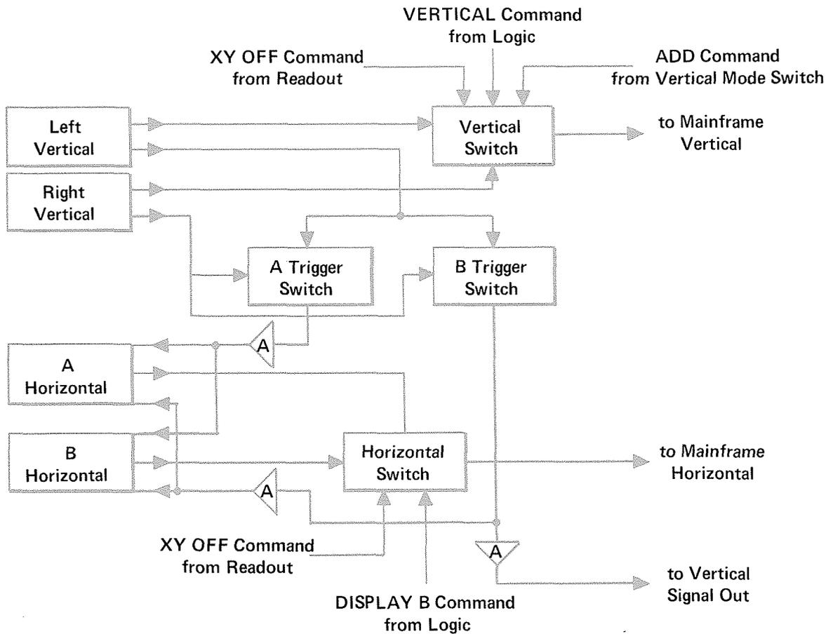
Fig. 1 Vertical, Horizontal and Trigger switching block diagram.
