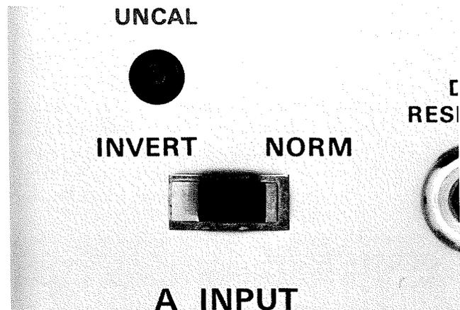
*Slide switches of this type "break before make". This allows the troubleshooter to select a mid-range break position that opens the input to the output amplifier.*
