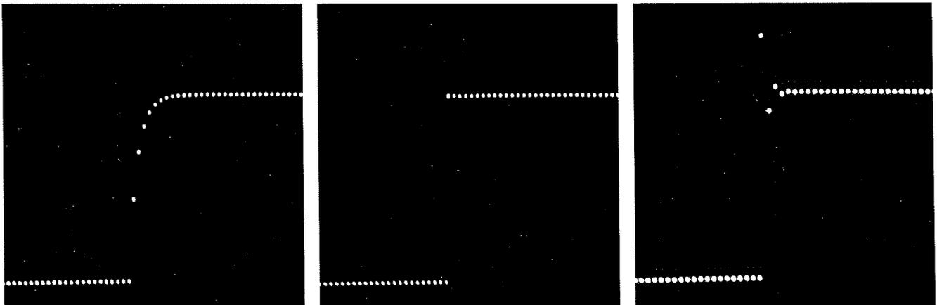
The sampling gate is unable to fully charge the amplifier input capacity with one sample. Feedback after the gate completes the charging process. Adjustments in the "Loop" produce (1) less than full charge (gain  $<1$ ) (2) full charge (gain = 1) (3) more than full charge (gain  $>1$ ).
