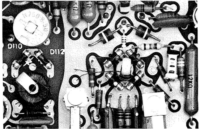
Here's where most of the fast action occurs. A four-diode bridge makes the sub-nanosecond voltage sample. The two-diode memory gate accepts processed sample and holds the information for CRT vertical deflection.
