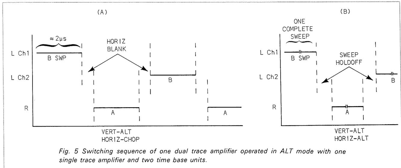
TP 167 A Sweep Inhibit – A high level prevents A sweep from running during the time B sweep is displayed.
