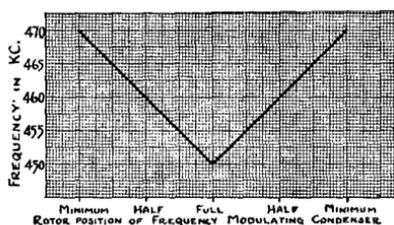
Obviously, the correct setting of the frequency modulating condenser for the correct mean frequency is about half capacity. The increase from half to maximum capacity serves to produce the change in frequency from the mean figure to the lowest frequency. The decrease from half capacity to minimum capacity serves to produce the change in output frequency from the mean frequency to the highest frequency.
