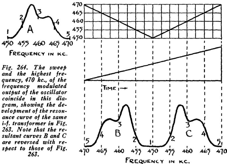
Fig. 264. The sweep and the highest frequency, 470 kc., of the frequency modulated output of the oscillator coincide in this diagram, showing the development of the resonance curve of the same i-f. transformer in Fig. 263. Note that the resultant curves B and C are reversed with respect to those of Fig. 263.
