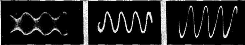
*Fig. 229-A, left, Fig. 229-B, middle, Fig. 229-C, right. A. The wave envelope of the modulated output of a commercial test oscillator. B. The a-f. output of the same oscillator. C. The a-f. signal resulting from demodulation of the modulated wave shown in A.*
