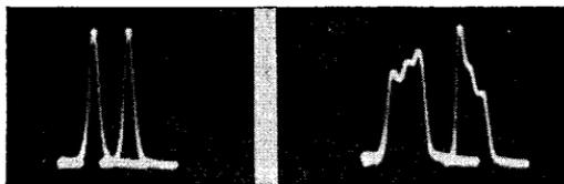
modulating unit, also is important. If the polarity is incorrect, the pattern is greatly distorted. Examples are shown in figures 316 and 317. The image shown in figure 316 is for correct polarity of the impulse generator signal and all other adjustments correct. The pattern shown in figure 317 is for the same signal under exactly the same conditions, except that the polarity of the signal obtained from the impulse generator has been reversed.
