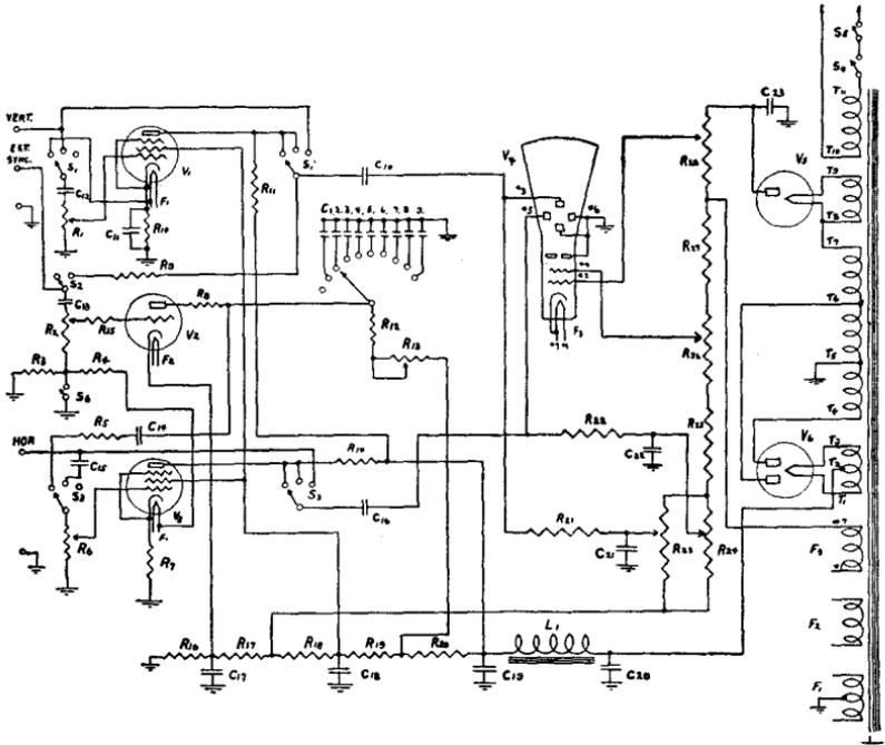
*Schematic diagram of the Triumph Model 800 cathode-ray oscillograph. Note the two rectifiers, the type 879 supplying the high voltages for the cathode-ray tube, type 906, and the type 80 supplying the bias and plate voltages for the remainder of the tubes.*
