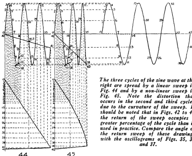
*The three cycles of the sine wave at the right are spread by a linear sweep in Fig. 44 and by a non-linear sweep in Fig. 45. Note the distortion that occurs in the second and third cycles due to the curvature of the sweep. It should be noted that in Figs. 42 to 45 the return of the sweep occupies a greater percentage of the cycle than is used in practice. Compare the angle of the return sweep of these drawings with the oscillograms of Figs. 35, 36 and 37.*
