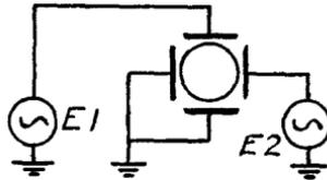
control, and the amplitude of the deflection in the other direction is made equal to the first. See figure 92. One voltage is applied to one set of plates and the other voltage in quadrature is applied to the other set of plates.
