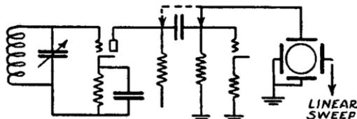
demodulator and ground. The same connections apply if the demodulator tube is transformer coupled to the audio stage following. If no condenser is in the high side of the vertical deflection plate, a .1-mfd. unit of suitable voltage rating will suffice.
