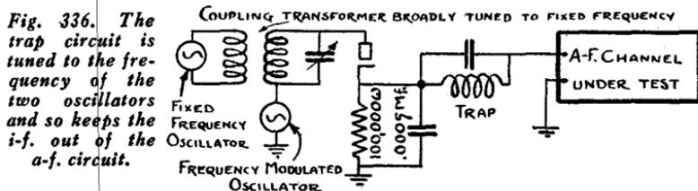
former tuned to about 200 kc. or whatever the frequency being used. To this winding is coupled the primary winding, which is connected to the other oscillator. The detector is a diode tube with a 100,000-ohm load resistor, shunted with a .0005-mfd. condenser. In the output voltage supply circuit is a trap tuned roughly to the frequency of the two oscillators, namely about 200 kc. This is used to keep i-f. out of the a-f. signal. The rest is the usual routine.
