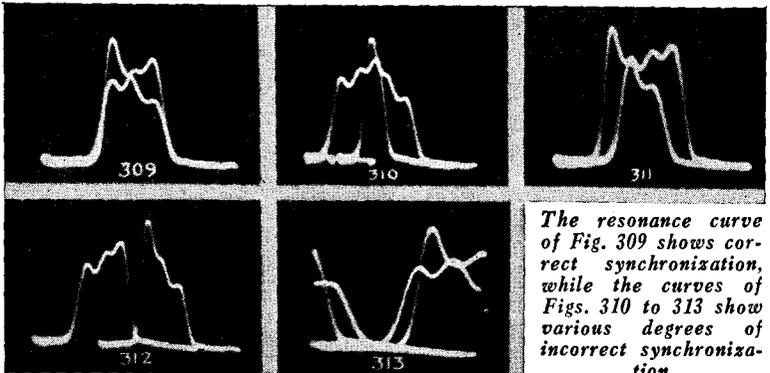
*The resonance curve of Fig. 309 shows correct synchronization, while the curves of Figs. 310 to 313 show various degrees of incorrect synchronization.*
