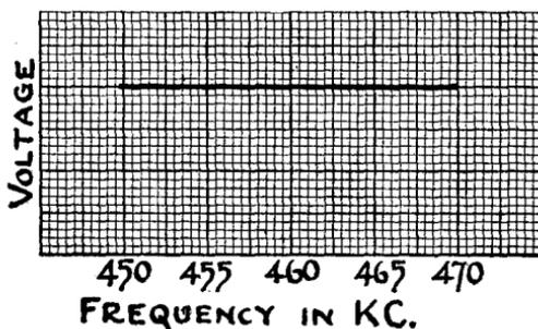
variation in voltage output may exist over the band used, but we shall assume for our discussion that the voltage output is of constant amplitude. The selection of the 450 kc. to 470 kc. band is purely illustrative. We assume that similar conditions prevail over any band width both sides of any periodic or mean frequency. It should be realized that a departure from such linearity of output will distort the final resonance curve.
