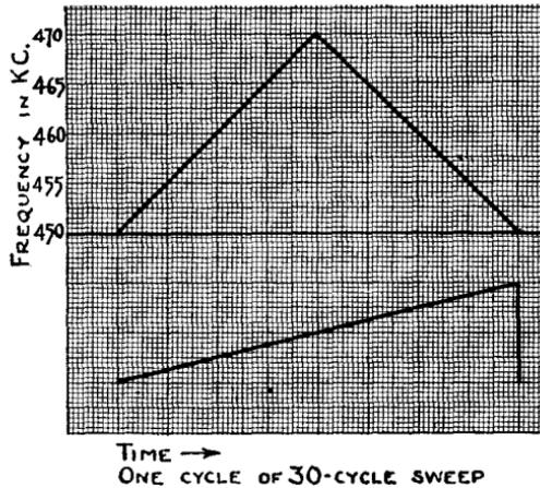
chronization. (The synchronizing pulse, secured from the impulse generator in the RCA frequency modulator unit will keep the sweep circuit in step, once the proper adjustment has been reached.)
