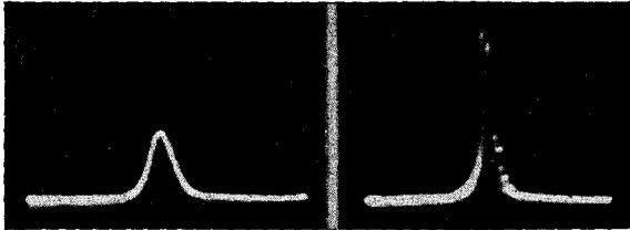
quency is indicated or spotted upon the pattern or image by the point where the two curves cross each other. A pattern of this type indicates that the response of the circuit is better to frequencies one side of the mean frequency than to frequencies on the other side of the mean frequency.
