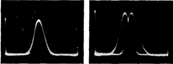
*The left pattern shows the circuit in resonance and that at the right, the circuit out of resonance. These oscillograms made with the Supreme 555.*
