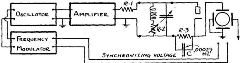
*Fig. 328. Schematic diagram of the circuit for checking the effect of damping upon the response of a simple tuned circuit.*
