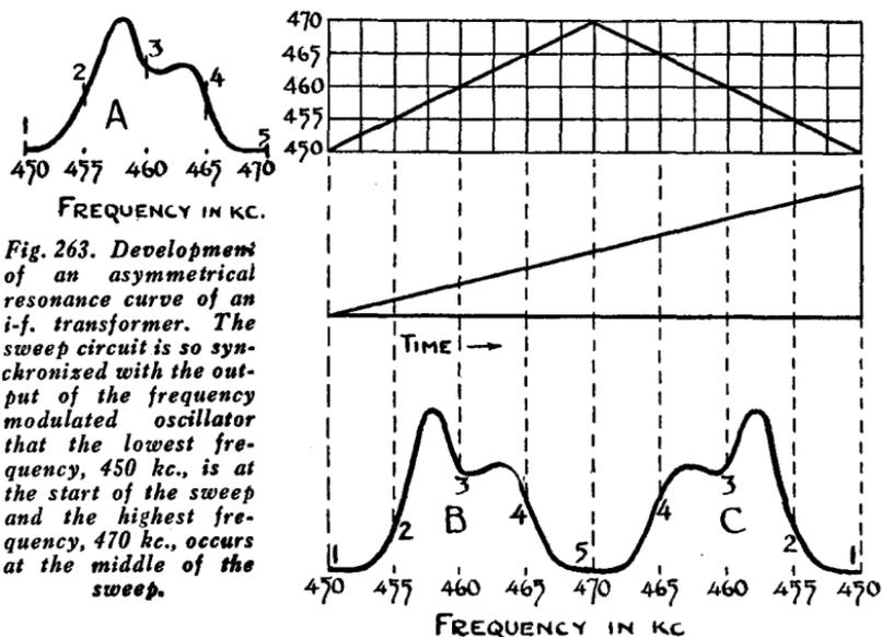
*Fig. 263. Development of an asymmetrical resonance curve of an i-f. transformer. The sweep circuit is so synchronized with the output of the frequency modulated oscillator that the lowest frequency, 450 kc., is at the start of the sweep and the highest frequency, 470 kc., occurs at the middle of the sweep.*
