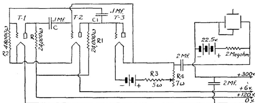
*Fig. 39. Schematic diagram of the so-called multi-vibrator circuit. Note that this is nothing more than a two-stage resistance-capacity coupled amplifier arranged to feed back on itself. It is possible to generate fundamental frequencies up to 30 or 40 kilocycles.*
