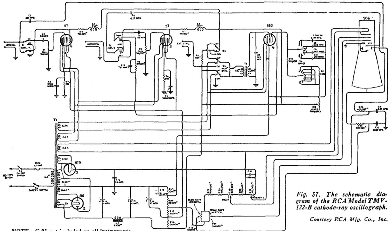
Fig. 57. The schematic diagram of the RCA Model TMV-122-B cathode-ray oscillograph.
