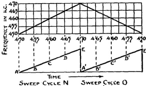
Fig. 271. The sweep frequency is here twice what it was in Fig. 261. Cycle N of the sweep spreads the frequency modulated output from 450 kc. to 470 kc. over the screen and cycle O spreads the descending part of the output. Points A to E and A' to E' coincide on the screen. See Figs. 272 to 274.
