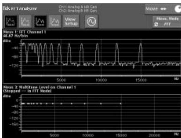
Figure 4-46: Display of FFT multitone signal and the corresponding multitone measurement
