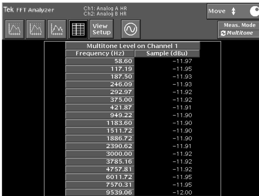
Figure 4-47: FFT multitone table display
