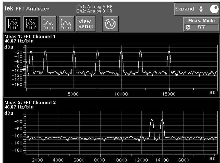
Figure 4-36: FFT Analyzer measurement showing a dual channel spectral display
