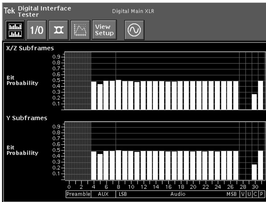
Figure 4-59: Bit Probability display with 24-bit digital data
