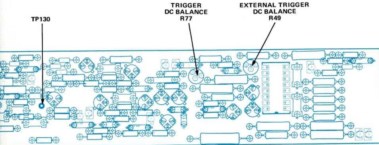
Fig. 6-10. Trigger circuit board adjustment locations.
