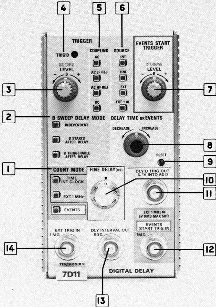
Fig. 1-2. 7D11 front-panel controls and connectors.
