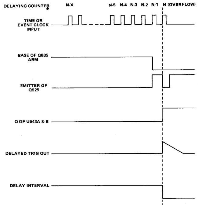
Fig. 2-9. Delaying Counter and Outputs Timing diagram.
