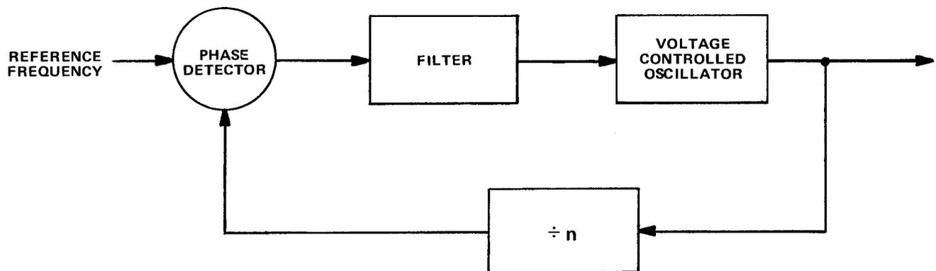
**Fig. 2-3.** Voltage Controlled Oscillator in Phase Locked Loop.
