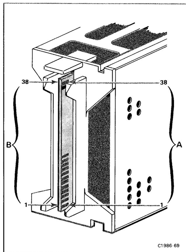
Figure 4-5. Location of pin numbers on Interface connector.
