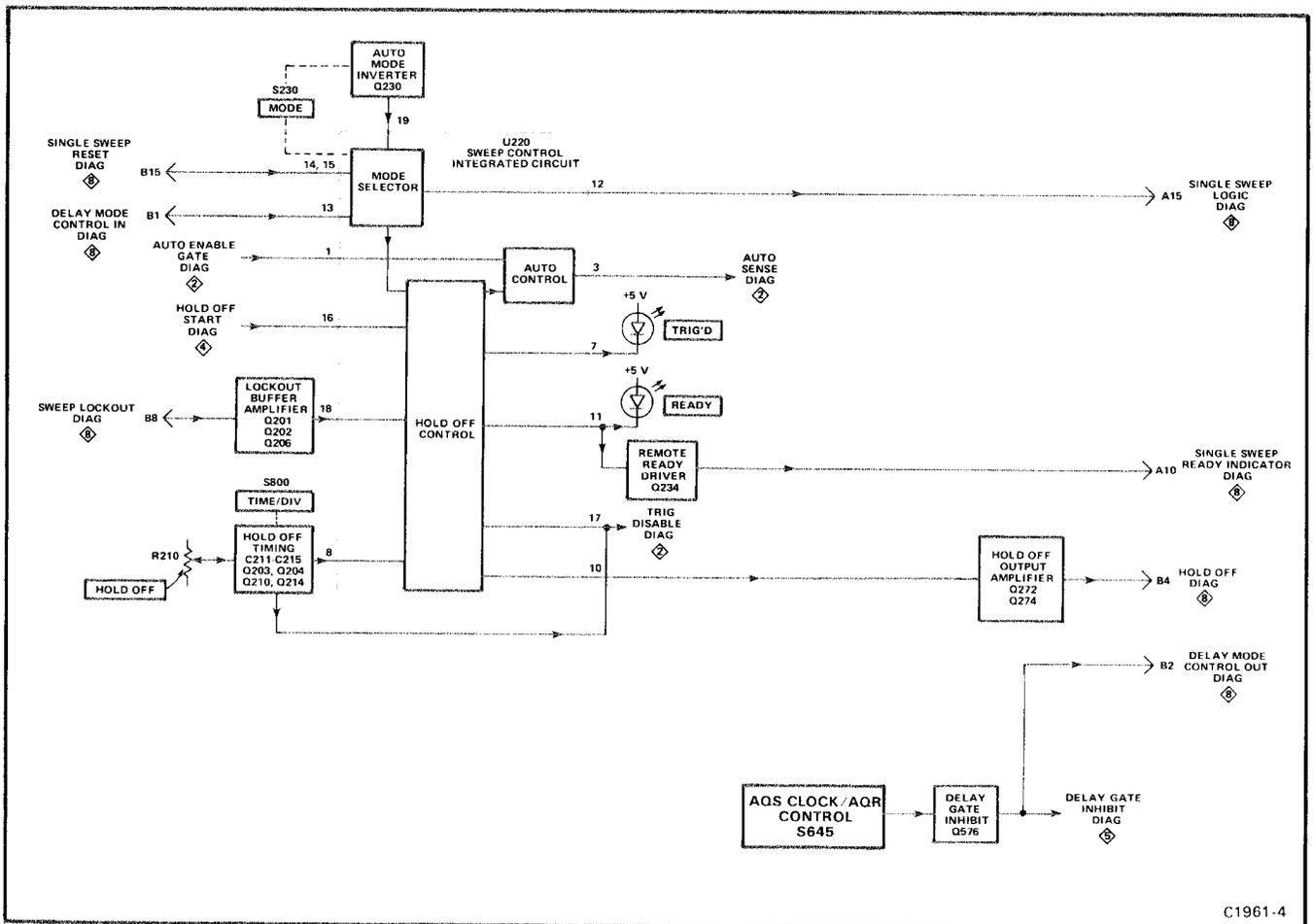
Figure 3-4. Detailed block diagram of Logic circuit.
