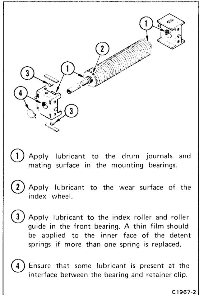
Figure 4-1. Lubrication procedure for a typical cam switch.
