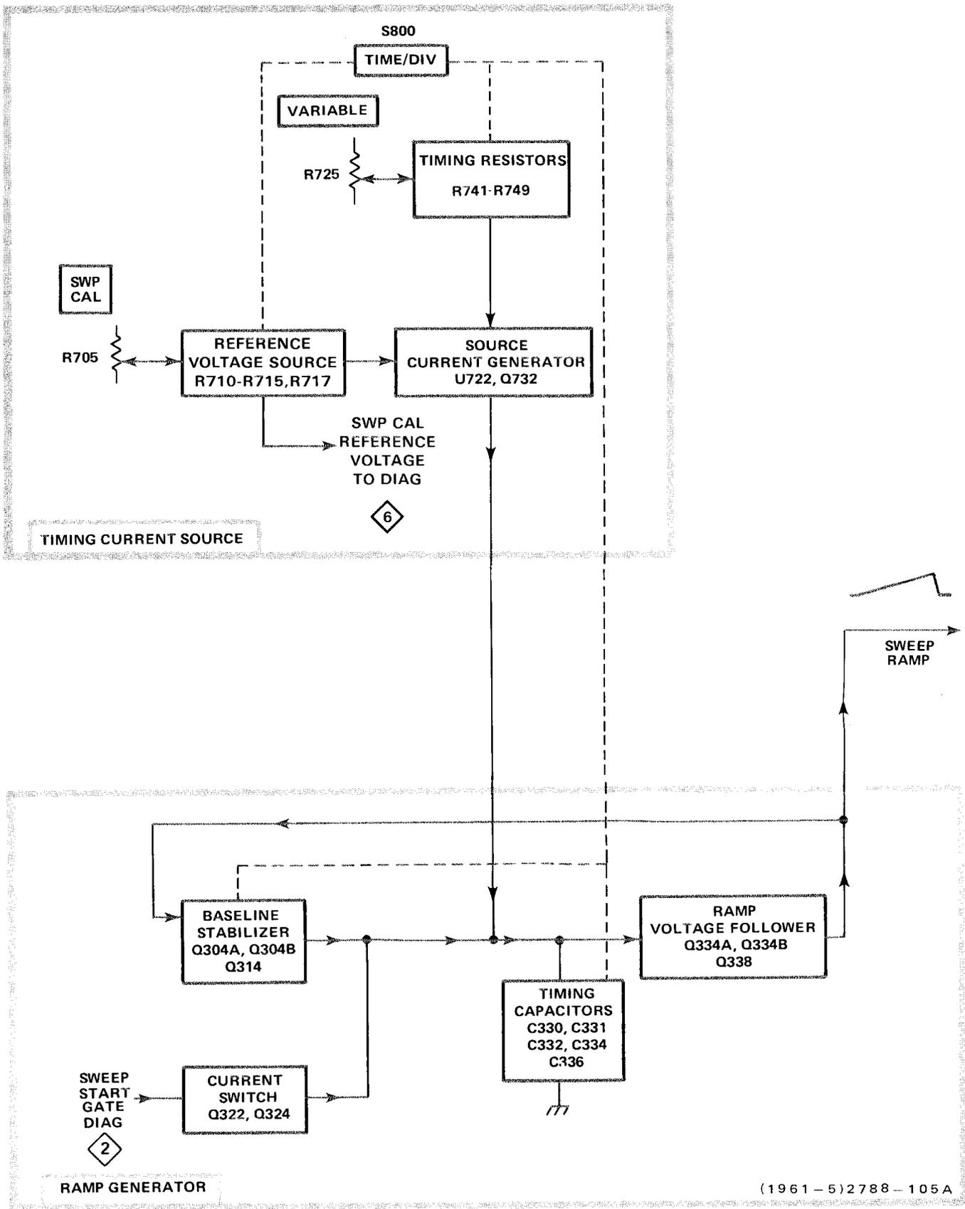
Figure 3-5. Detailed block diagram of Sweep Generator.
