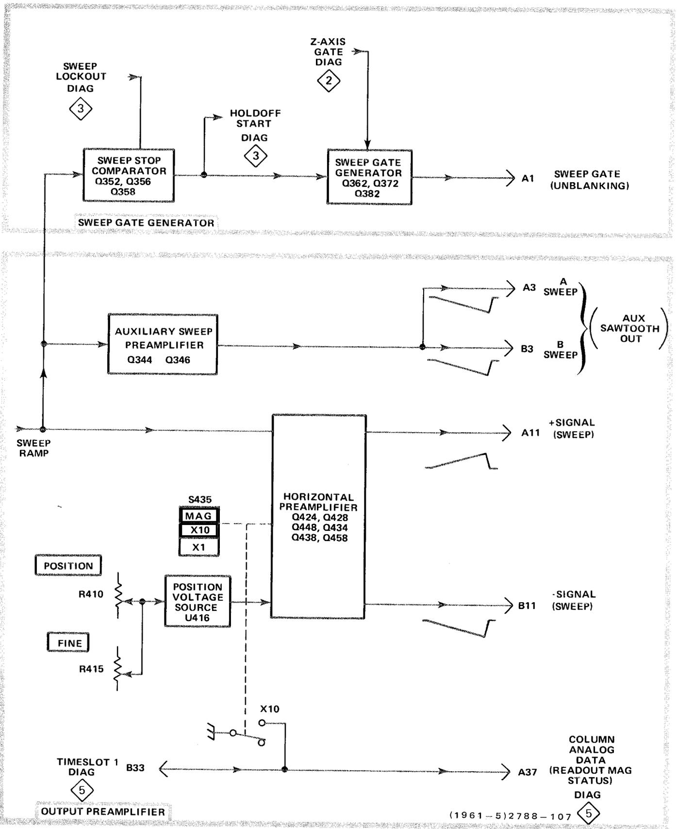
Figure 3-5 (cont). Detailed block diagram of Sweep Generator.
