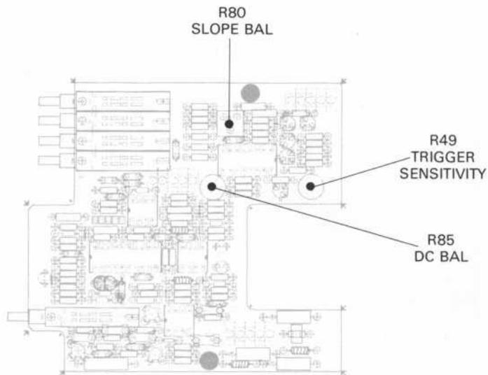
Figure 8-7. Test Point and Adjustment Locations
