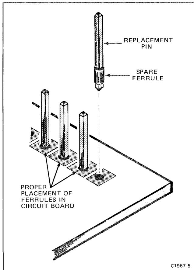
Figure 4-12. Exploded view of circuit-board pin and ferrule.
