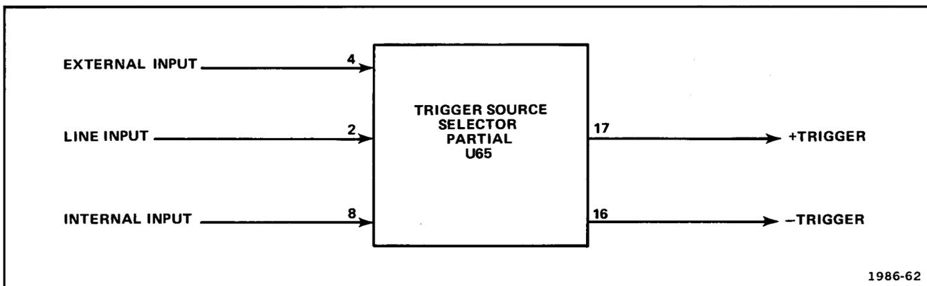
Fig. 3-3. Functional diagram of Trigger Source Selector.
