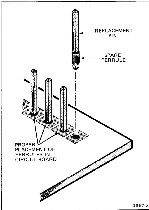
Fig. 4-11. Exploded view of circuit-board pin and ferrule.
