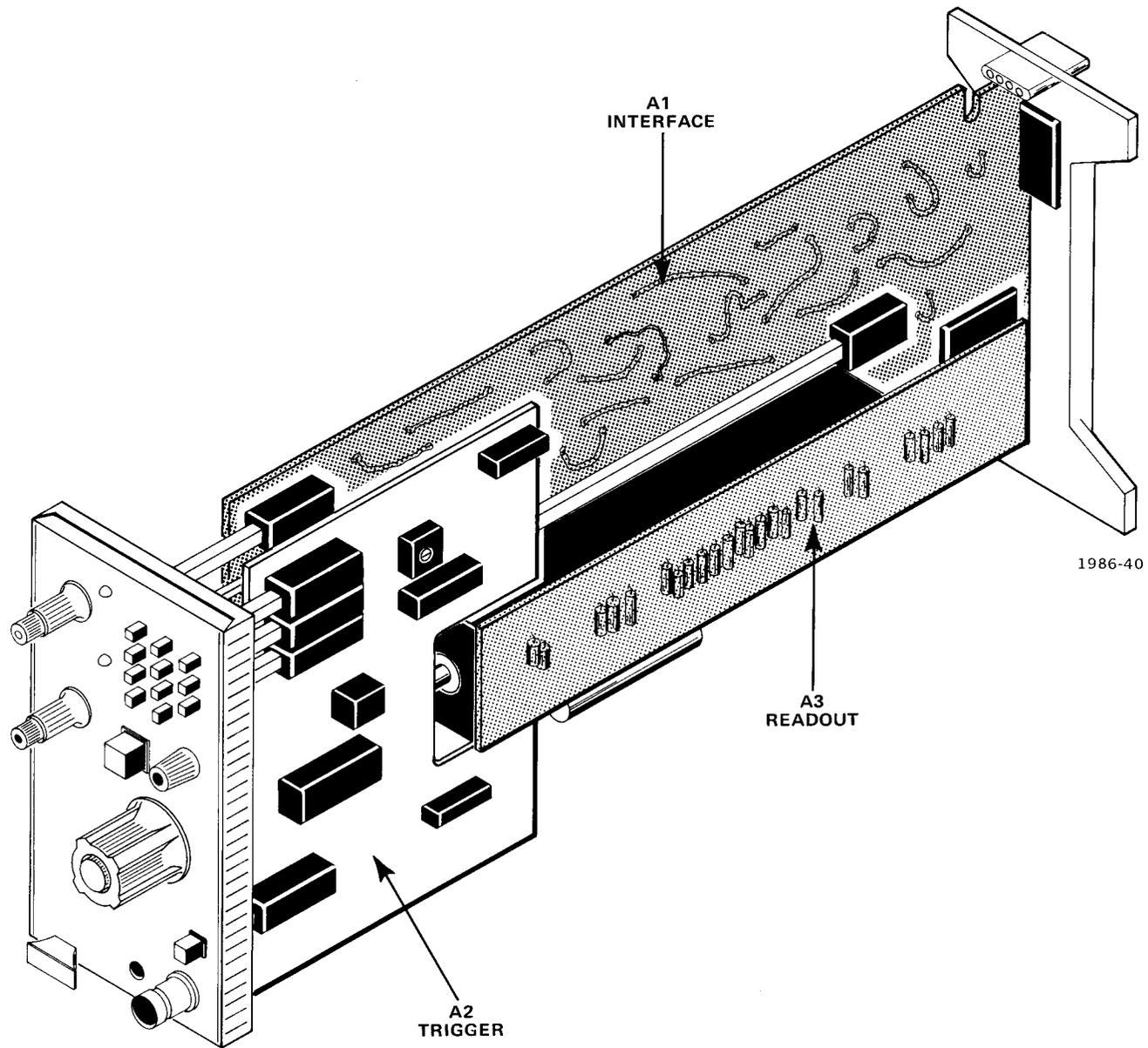
Fig. 8-2. Location of circuit boards in the 7B80.
