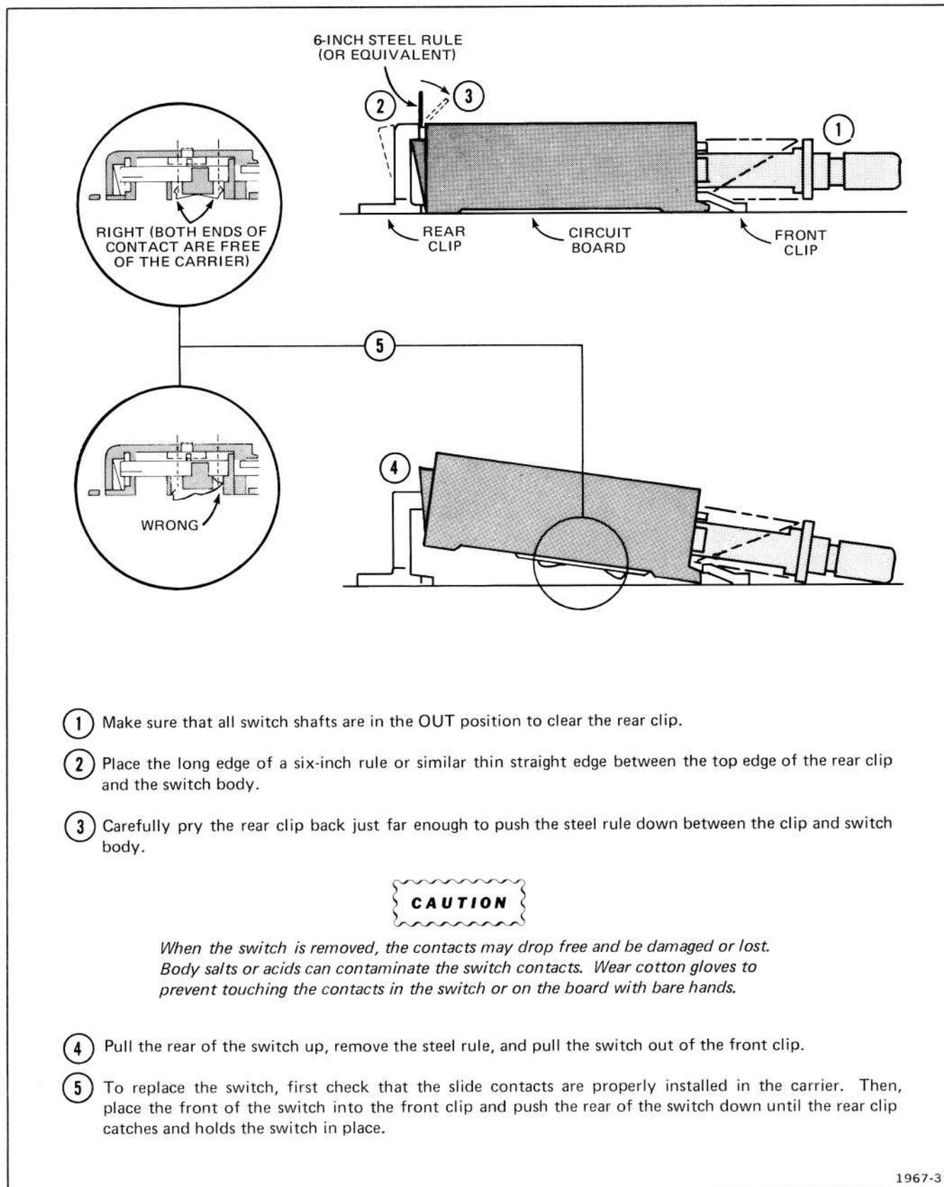
Fig. 4-10. Removal procedure for typical push-button switch.
