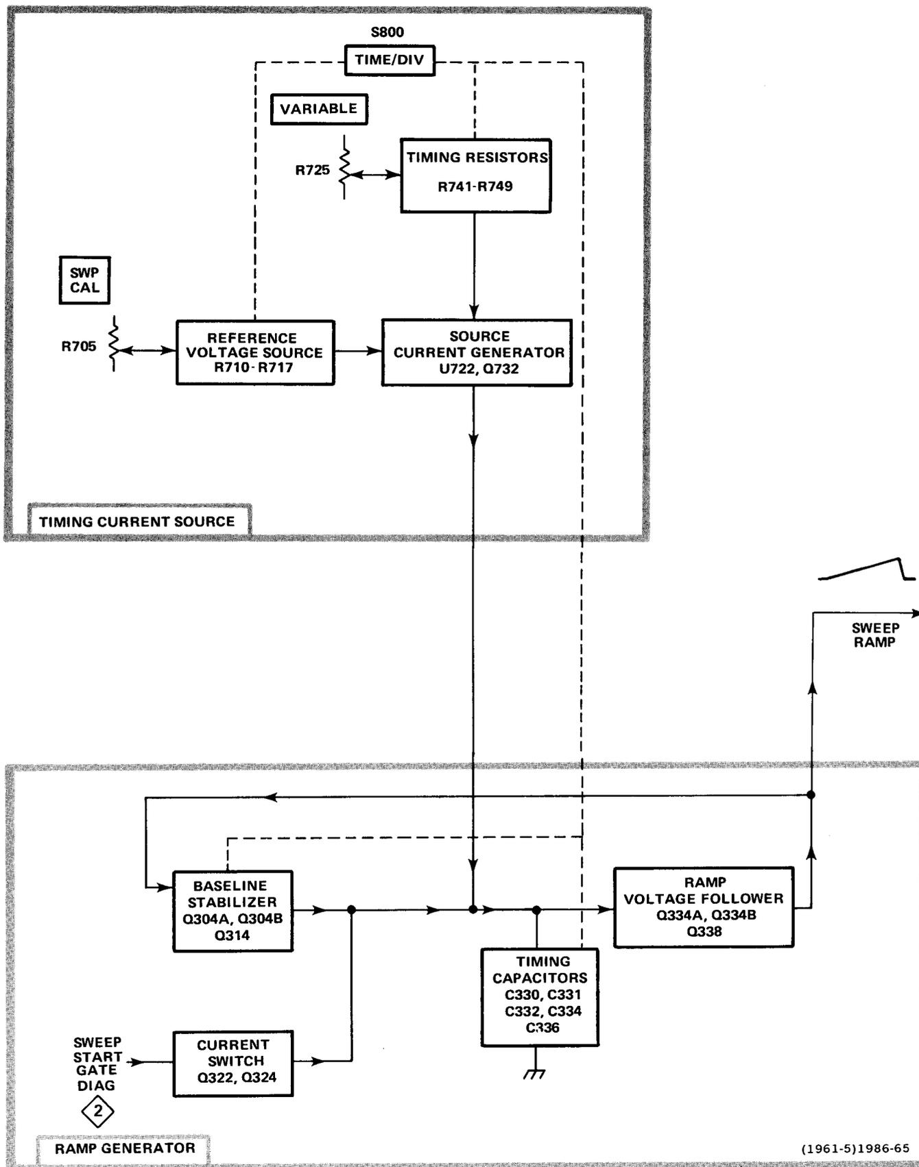
Fig. 3-6. Detailed block diagram of Sweep Generator.
