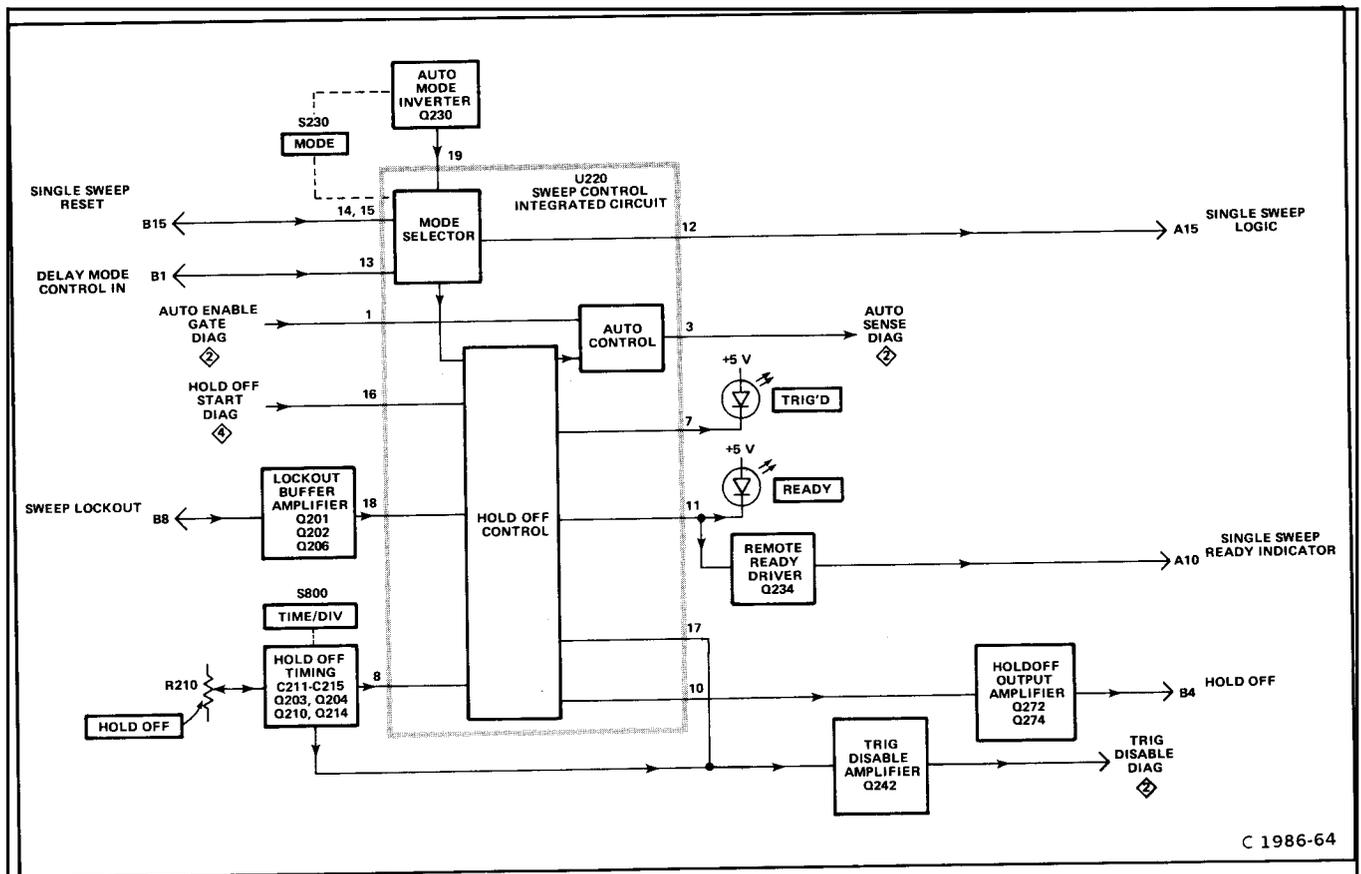
Fig. 3-5. Detailed block diagram of Logic circuit.
