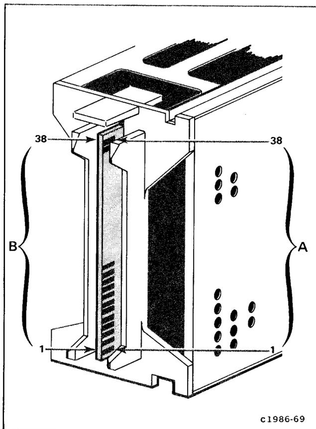
Fig. 4-5. Location of pin numbers on Interface connector.
