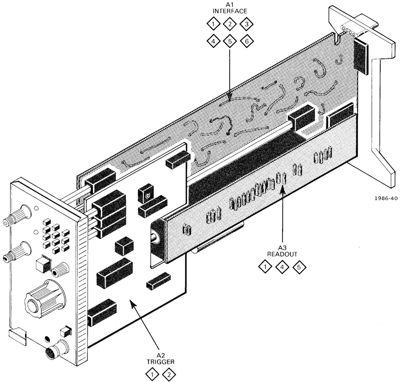
Figure 8-2. Location of circuit boards in the 7B10.
