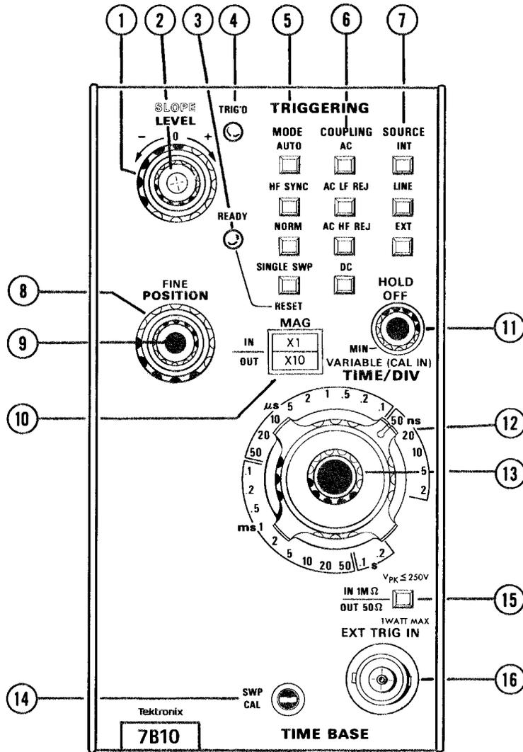
Fig. 2-1. Front-panel controls, connectors, and indicators.
