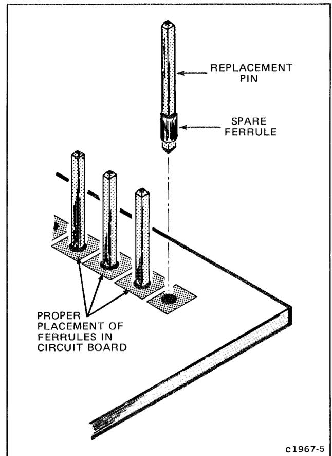
Fig. 4-11. Exploded view of circuit-board pin and ferrule.
