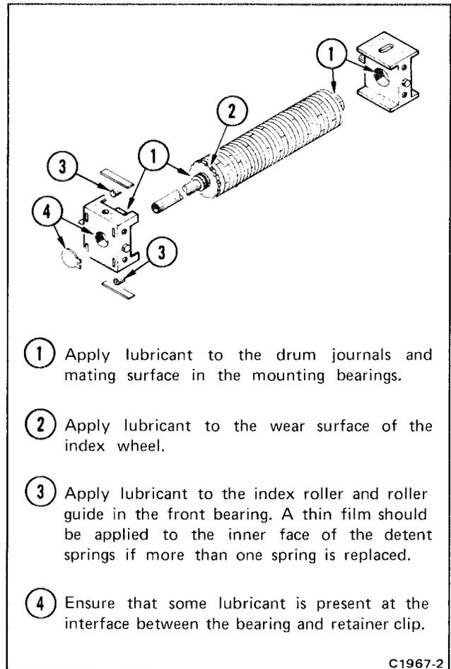
Fig. 4-1. Lubrication procedure for a typical cam switch.
