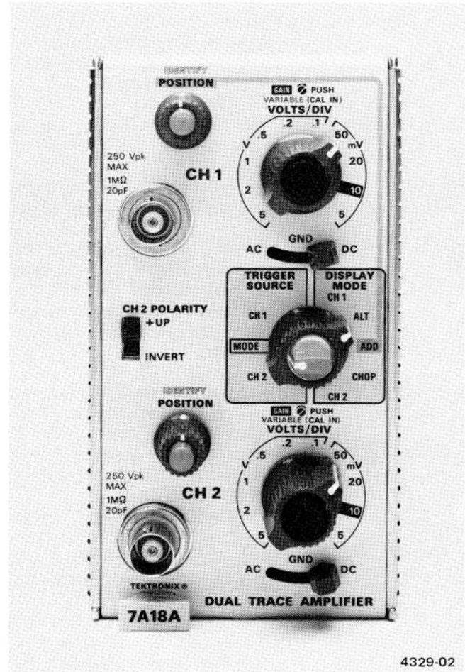
Fig. 2-1. Front-panel controls and connectors. (7A18A shown.)
