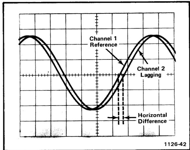
Fig. 2-4. Measuring phase difference between two signals.
