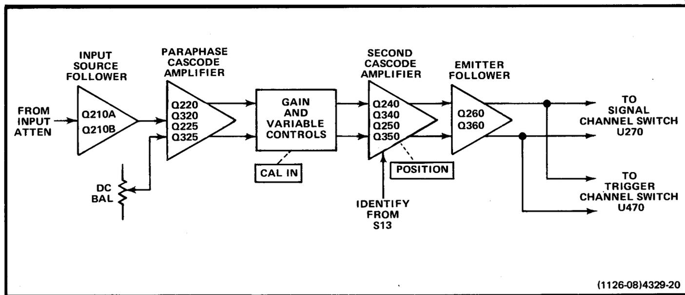
Fig. 3-1. Channel 1 Input Amplifier detailed block diagram.
