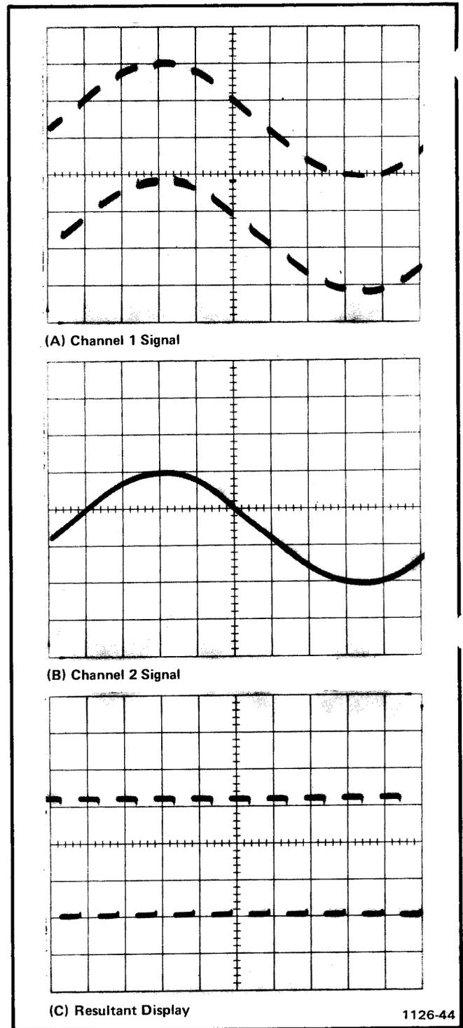
**Fig. 2-6.** Using the ADD mode for common-mode rejection. (A) Channel 1 signal contains desired information along with line-frequency component. (B) Channel 2 contains line frequency only. (C) Resultant CRT display using common-mode rejection.
