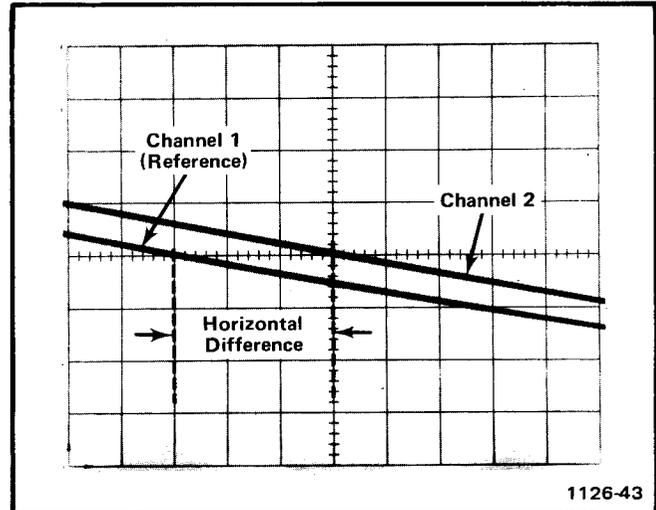
Fig. 2-5. High resolution phase measurement using time-base magnifier.
