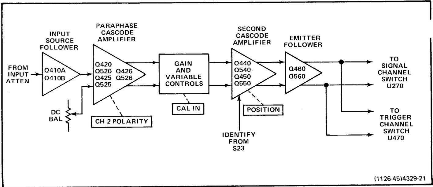
Fig. 3-2. Channel 2 Input Amplifier detailed block diagram.
