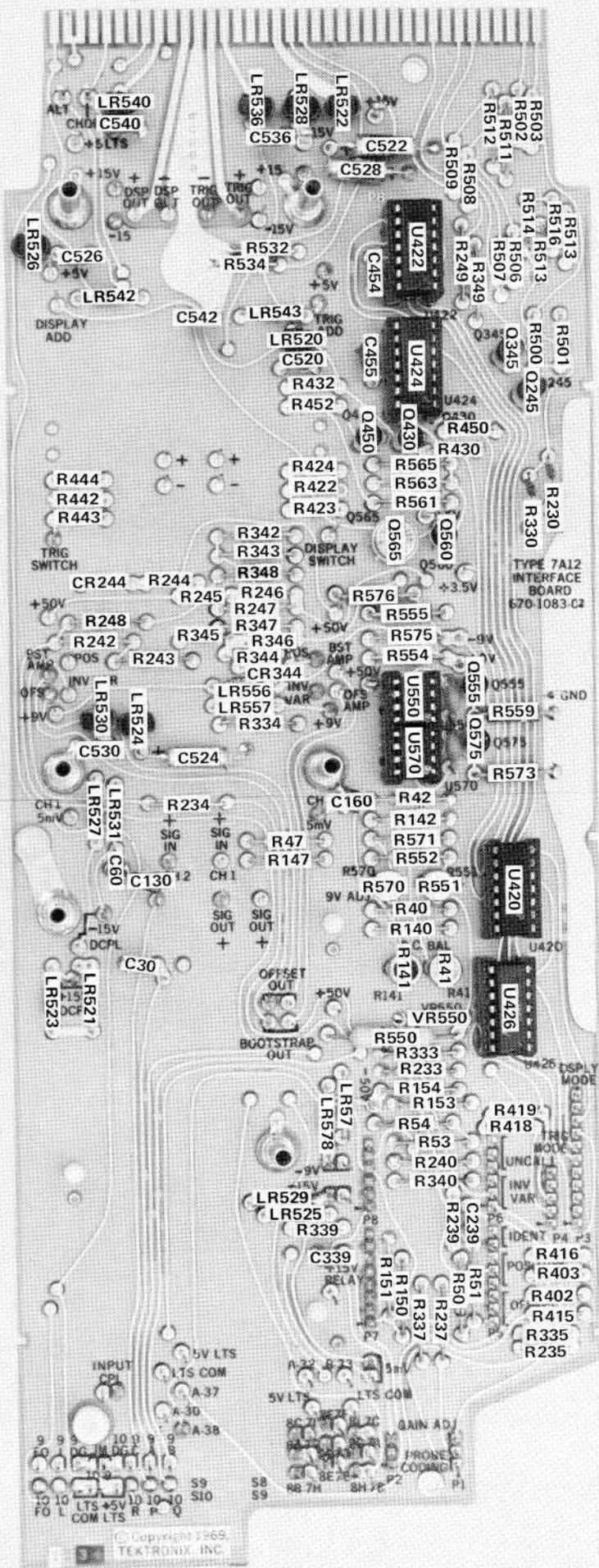
Fig. 7-5. Interface circuit board showing location of components.
