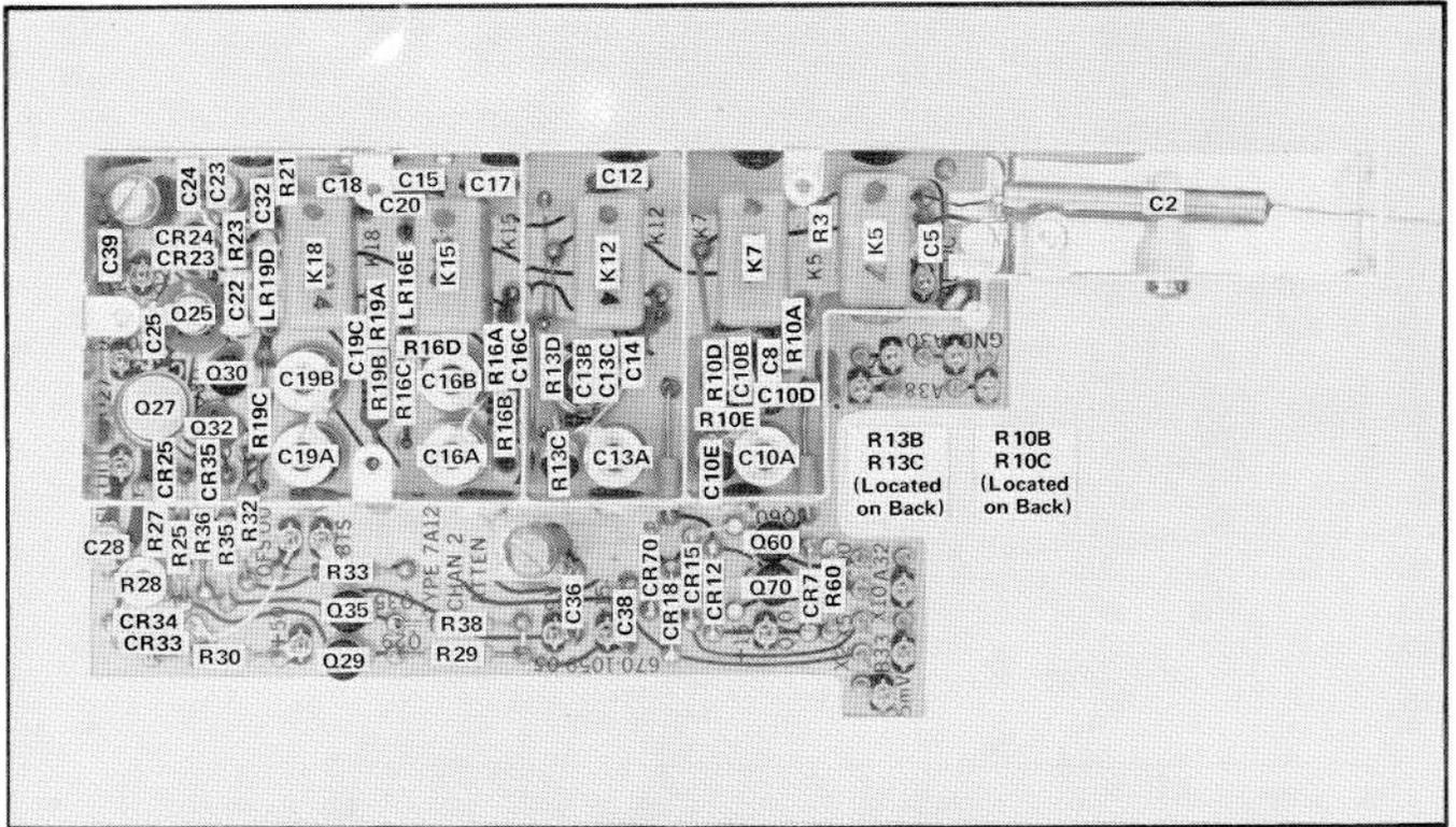
Fig. 7-2. Channel 2 Attenuator board showing location of components.
