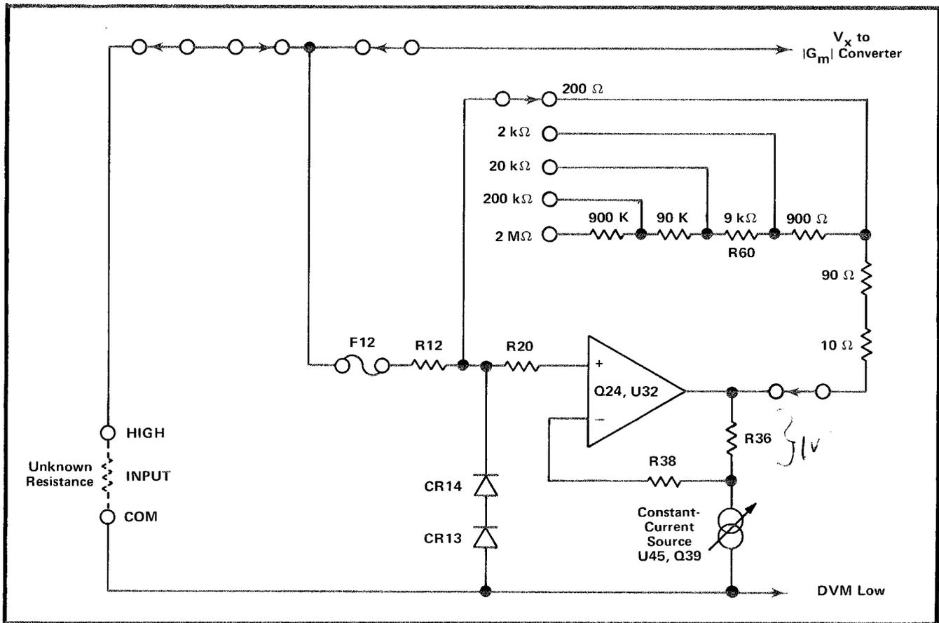
Fig. 3-1. Simplified diagram of the Ohms Converter circuit.
