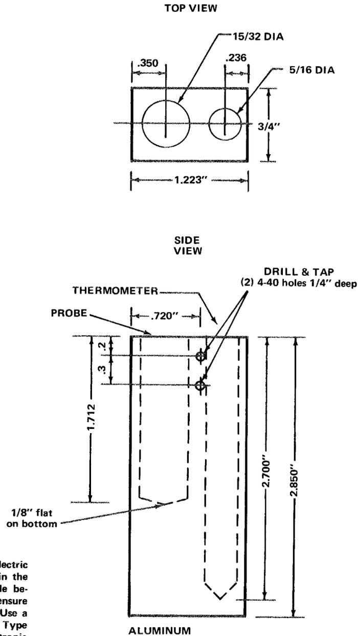
A small quantity of dielectric coolant should be placed in the equalizing block probe hole before installing the probe to ensure good thermal conduction. Use a dielectric coolant such as Type FC40 Fluorinert Brand Electronic Liquid.
