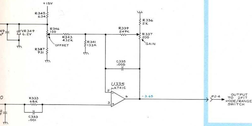
VOLTAGES obtained under conditions given on Page 72. Voltages are referenced to chassis ground except those marked with \* are referenced to TP422, floating power supply GND.
