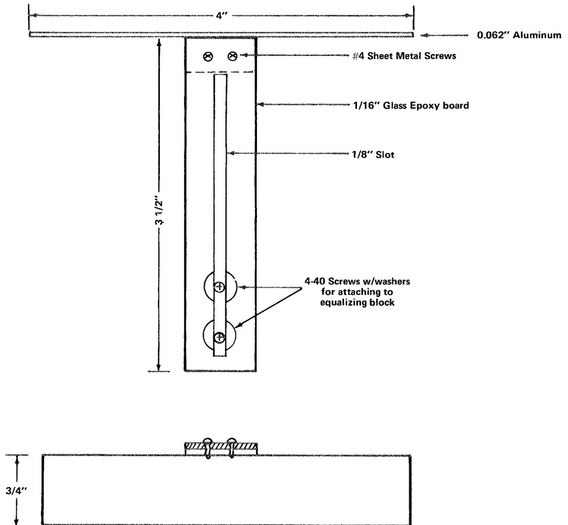
Fig. 5-3. Suspension bracket for temperature probe equalizing block.
