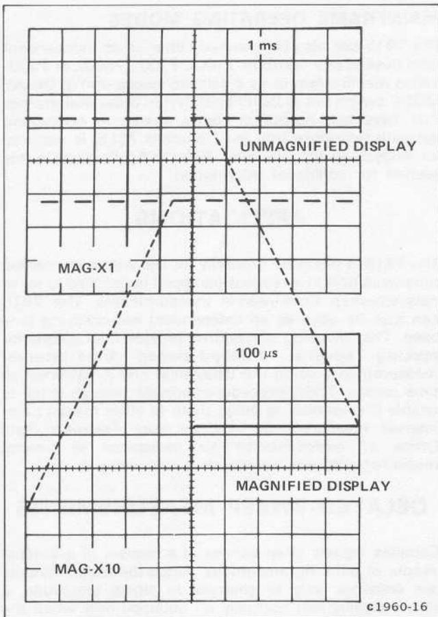
Figure 2-4. Effect of sweep magnifier on crt display.
