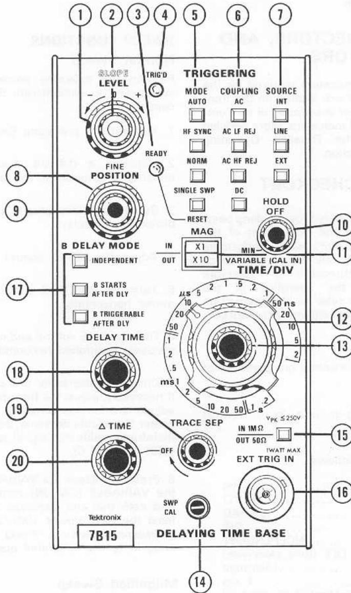
Figure 2-1. Front-panel controls, connectors and indicators.
