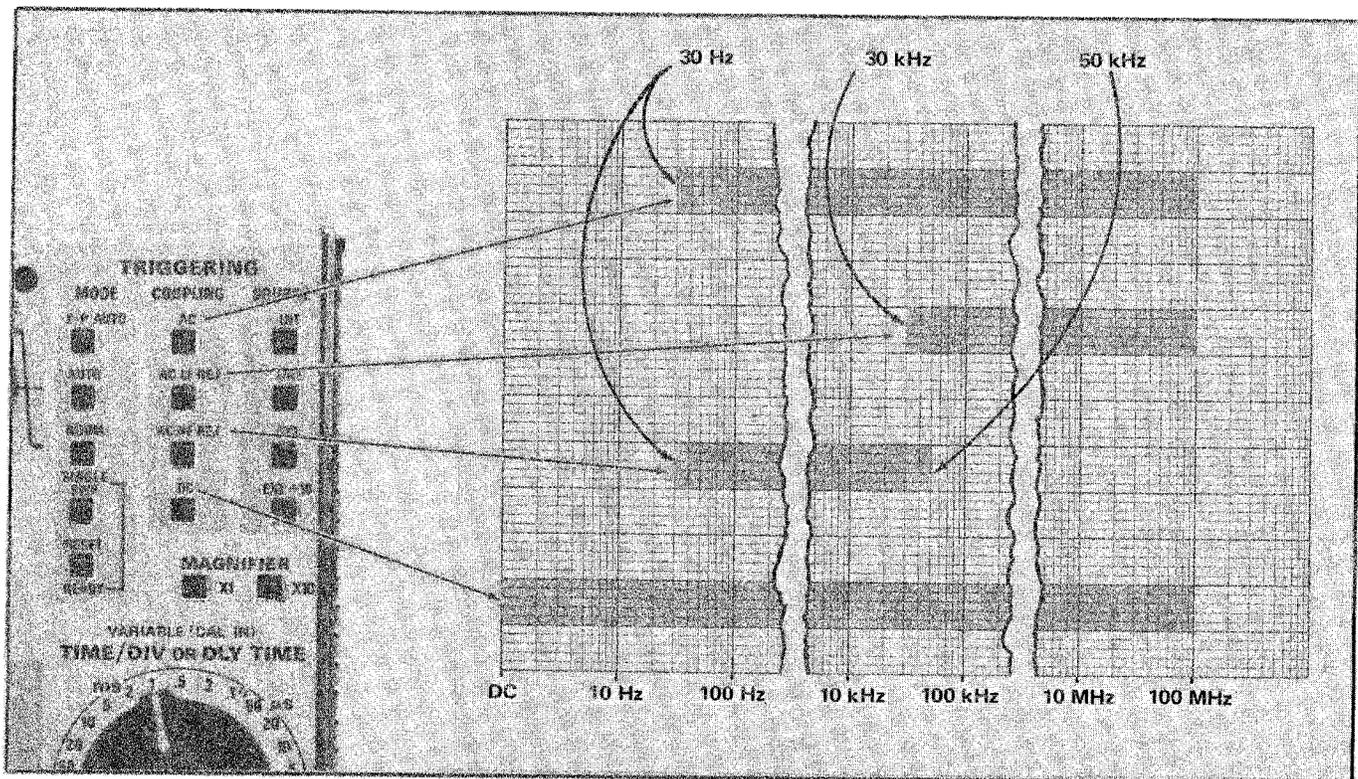
Fig. 2-6. Frequency range of each COUPLING switch position.
