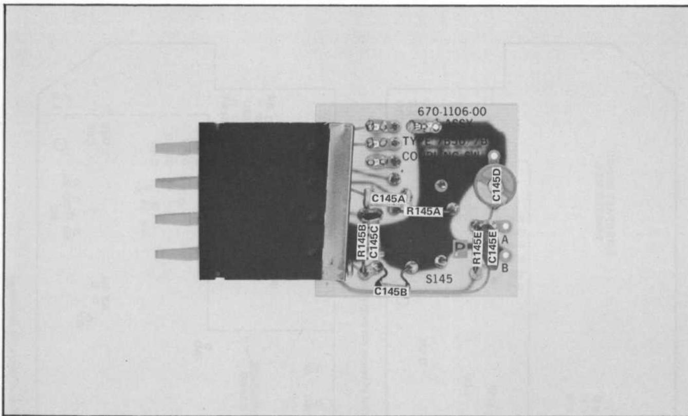
Fig. 4-7. Coupling switch board showing location of components.
