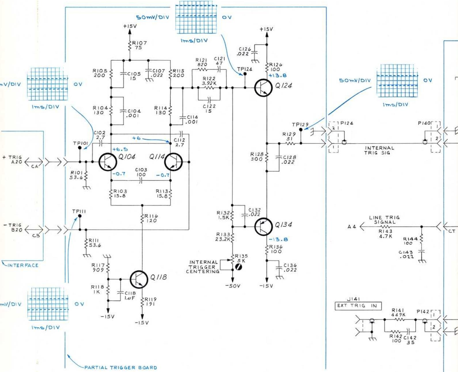
VOLTAGES and WAVEFORMS obtained under conditions on diagram ① except as follows:
