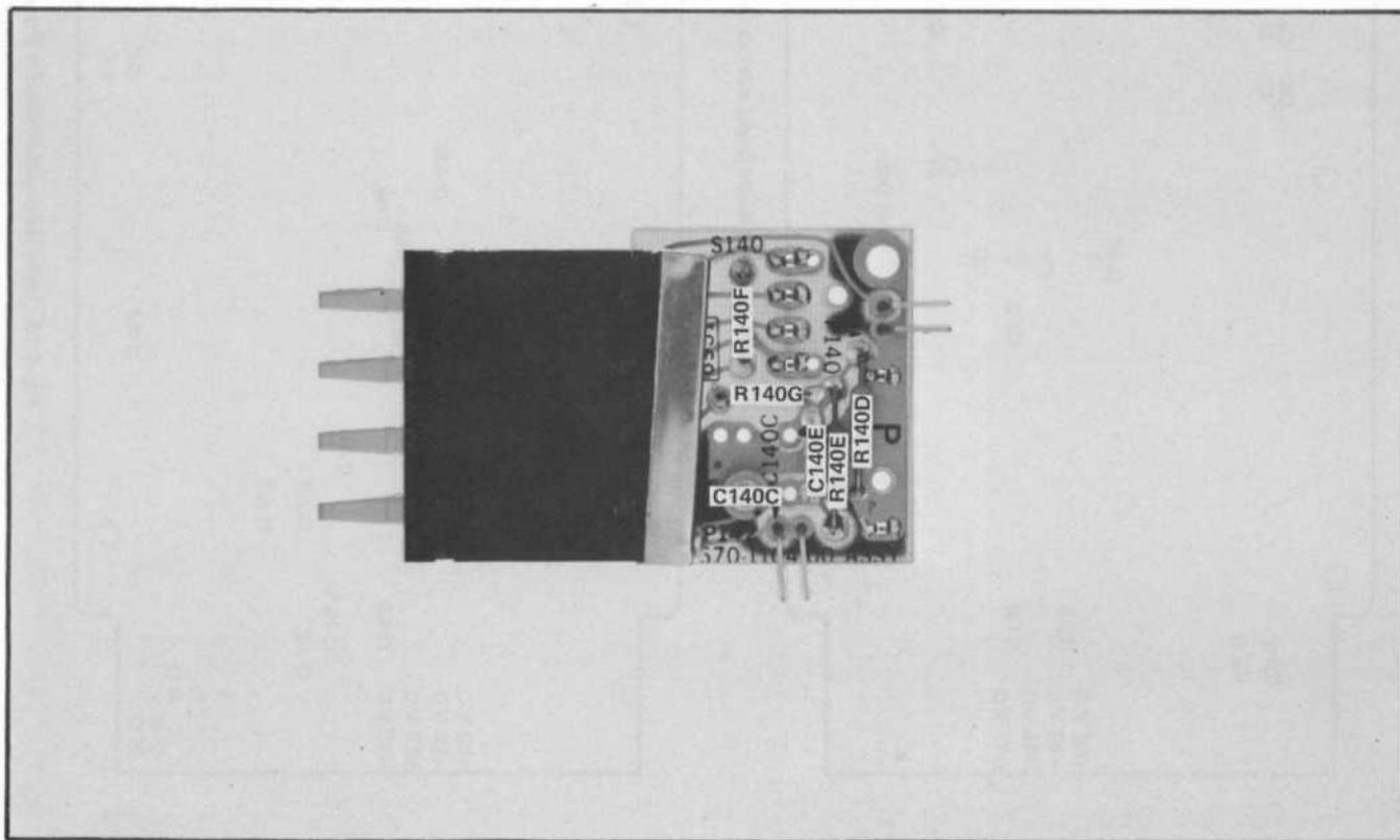
Fig. 4-8. Source switch board showing location of components.
