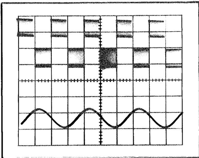
Fig. 2-14. Displaying a complex signal using delayed sweep.
