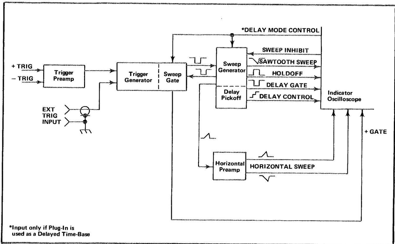
Fig. 3-1. Basic Block Diagram of the Type 7B51.
