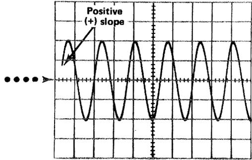
CRT displays obtained with LEVEL/SLOPE control in negative-slope region
