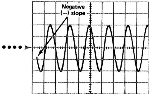
Fig. 2-7. Effect of LEVEL/SLOPE control on CRT display (AUTO P-P MODE).
